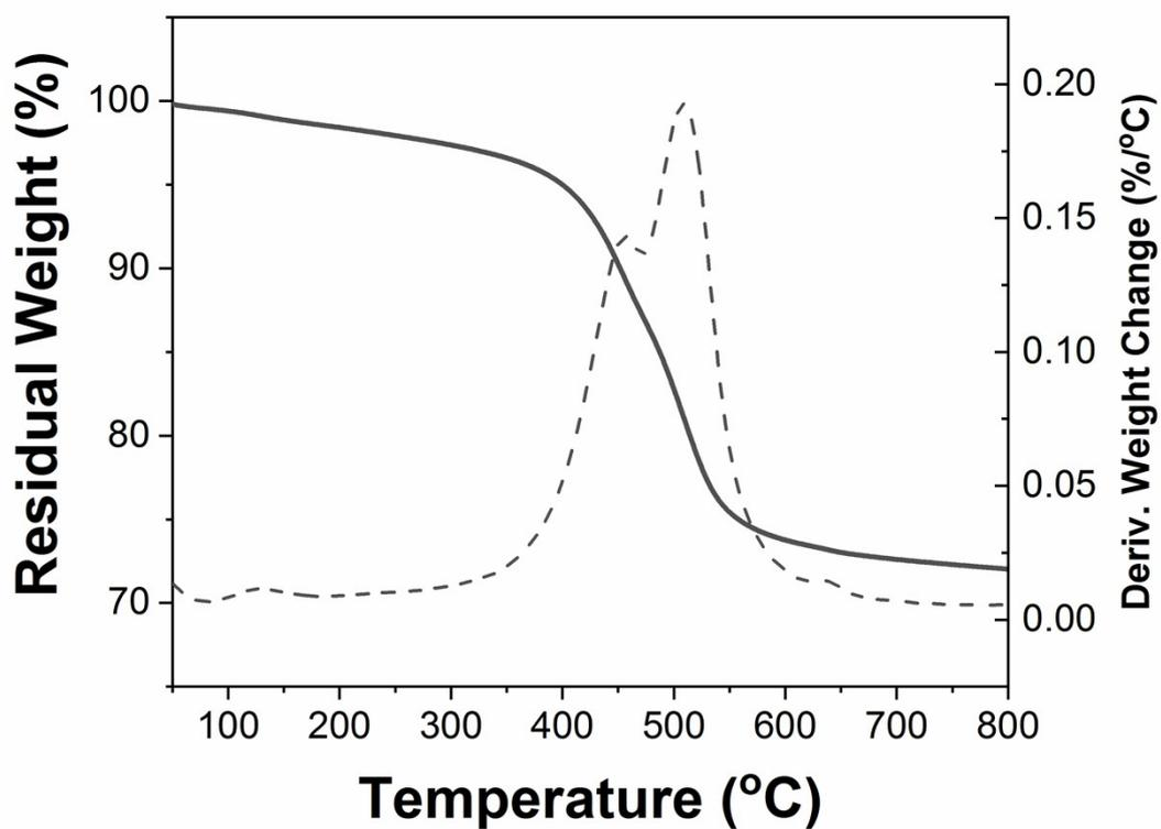
Figure S15. TG and DTG curves of HNTs-I-PS (Case.No.4 in Tab.1)
