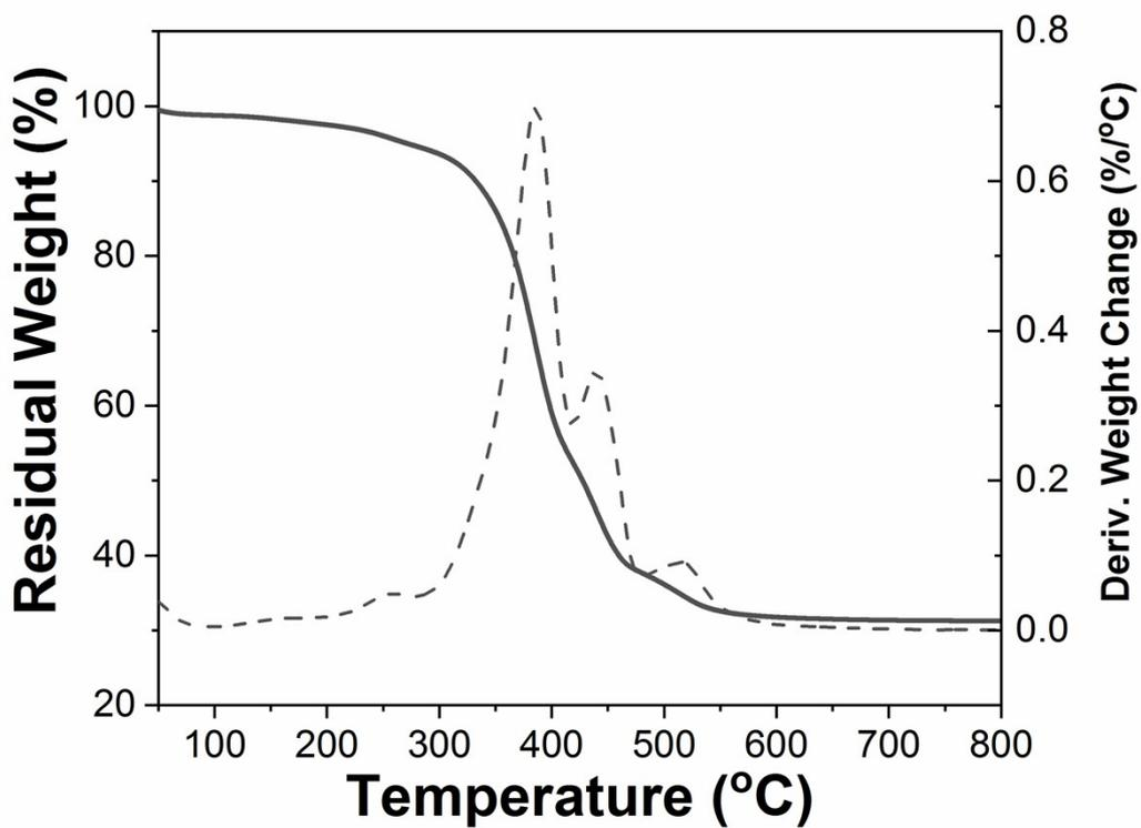
Figure S20. TG and DTG curves of HNTs-I-PHEMA (Case.No.9 in Tab.1)
