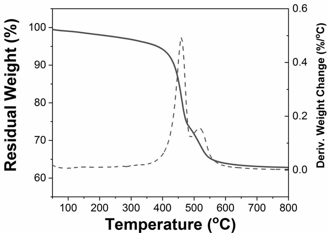
Figure S16. TG and DTG curves of HNTs-I-PS (Case.No.5 in Tab.1)
