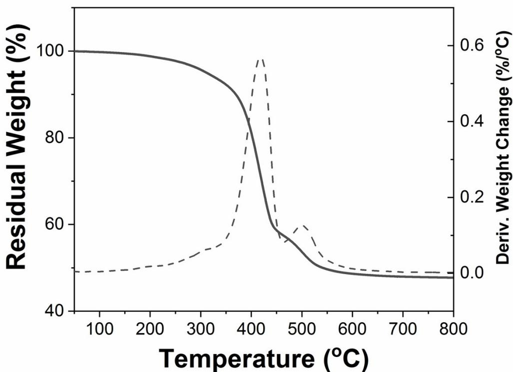
Figure S14. TG and DTG curves of HNTs-I-PMMA (Case.No.2 in Tab.1)
