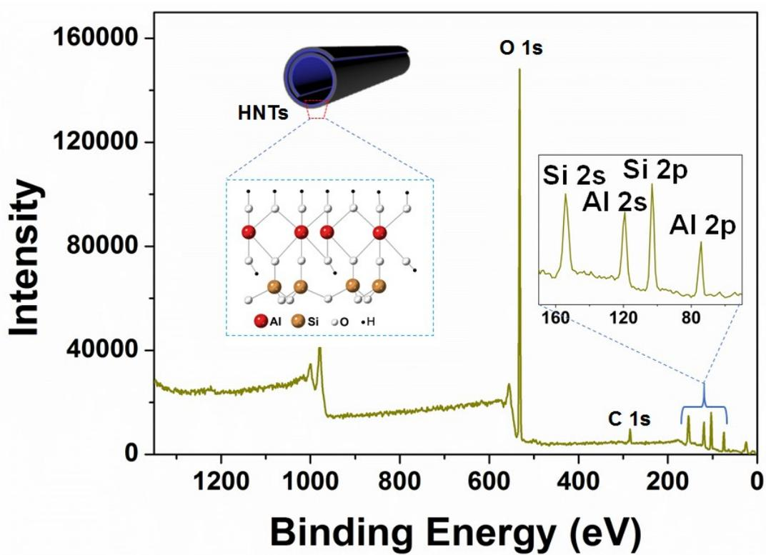
Figure S4. Schematic illustration of crystalline structure<sup>3</sup> and XPS spectrum of HNTs
