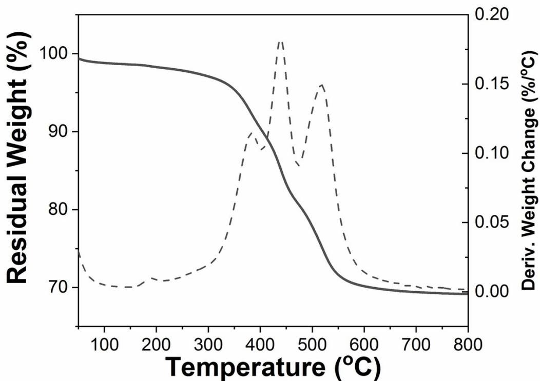
Figure S19. TG and DTG curves of HNTs-I-PHEMA (Case.No.8 in Tab.1)
