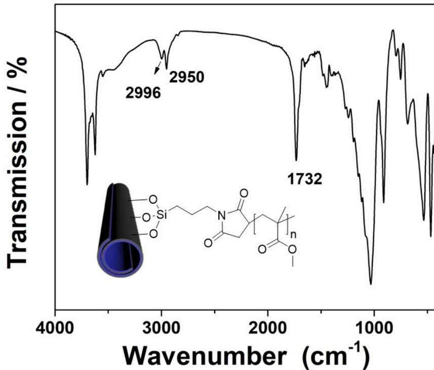
Figure S8. FTIR spectrum of HNTs-I-PMMA (Case.No.1 in Tab.1)
