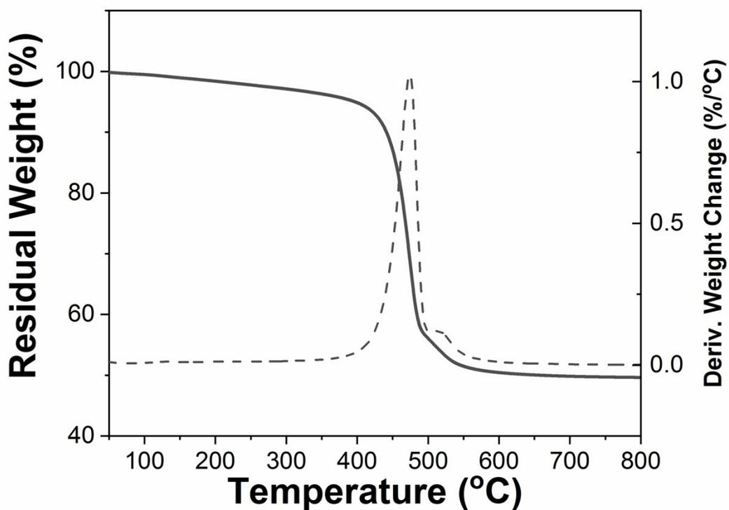
**Figure S18.** TG and DTG curves of HNTs-I-PS (Case.No.7 in Tab.1)
