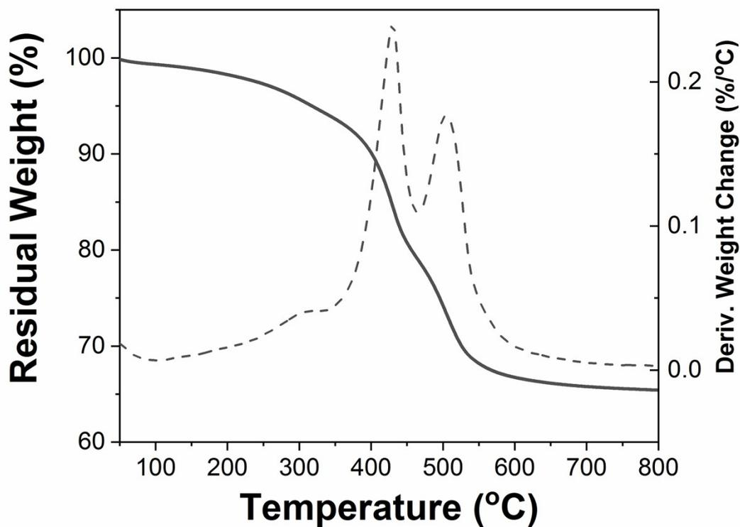
Figure S12. TG and DTG curves of HNTs-I-PMMA (Case.No.1 in Tab.1)
