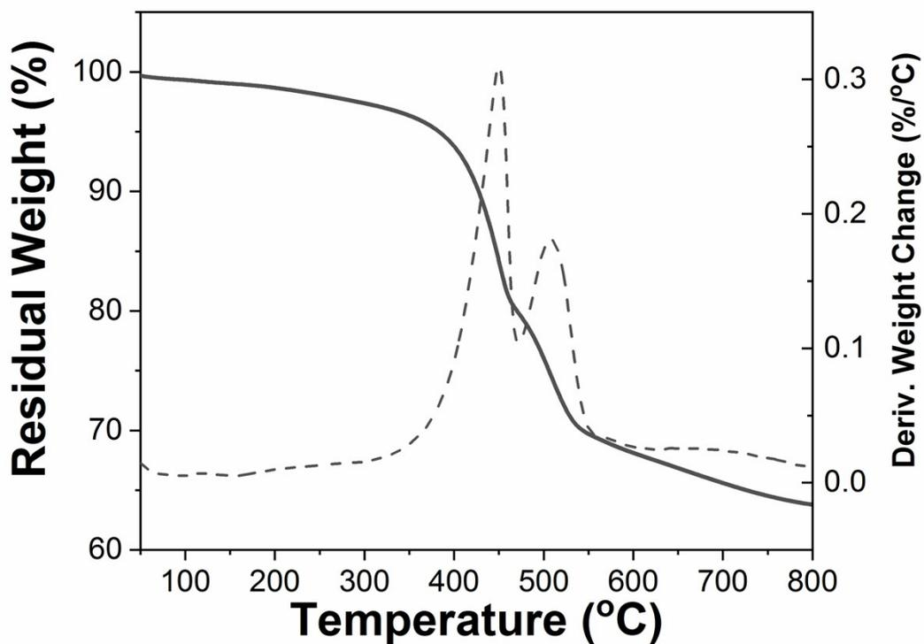
**Figure S17.** TG and DTG curves of HNTs-I-PS (Case.No.6 in Tab.1)
