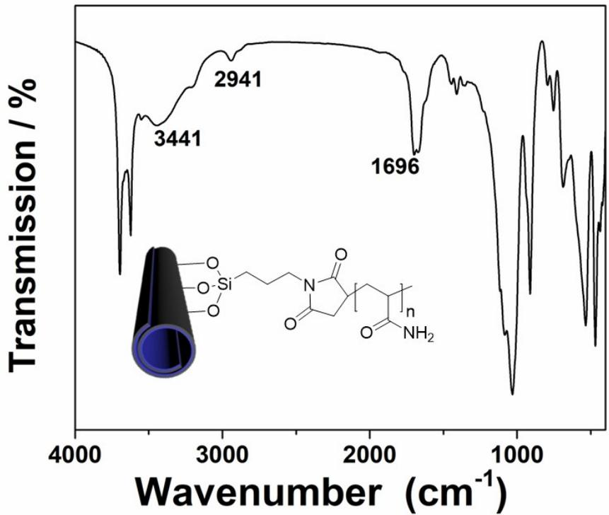
Figure S9. FTIR spectrum of HNTs-I-PAM (Case.No.10 in Tab.1)
