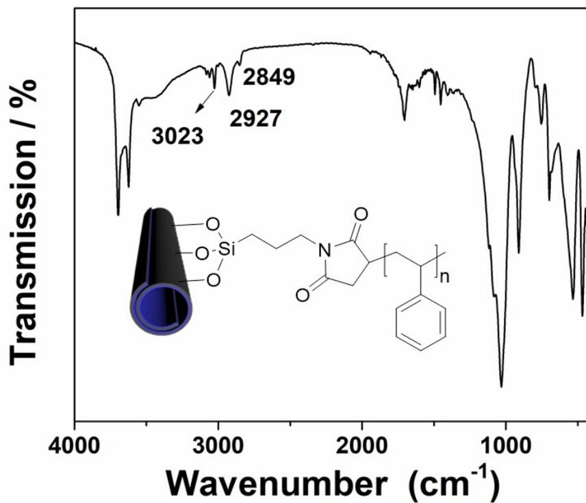
Figure S7. FTIR spectrum of HNTs-I-PS (Case.No.4 in Tab.1)
