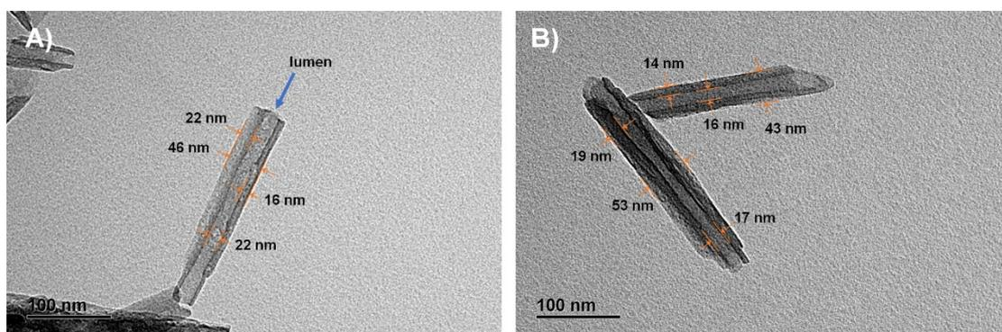
**Figure S2.** TEM images of pristine HNTs with calculated lumen diameters, outer diameters and walls thickness
