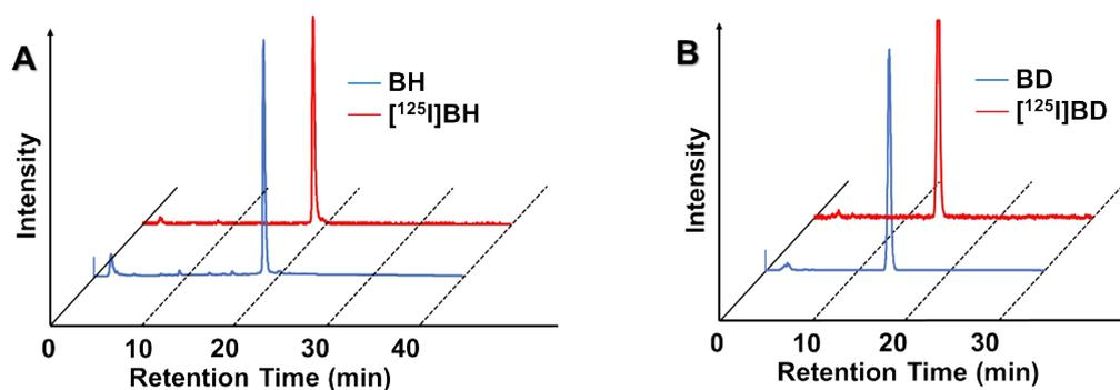
**Figure S1.** RP-HPLC coelution of [ $^{125}\text{I}$ ]BH with nonradioactive BH (A) and [ $^{125}\text{I}$ ]BD with BD (B). Mobile phase condition: (A)  $\text{H}_2\text{O}$  / MeCN / Trifluoroacetic acid = 70 / 30 / 0.1  $\rightarrow$  20 / 80 / 0.1 (0-40 min, gradient). (B)  $\text{H}_2\text{O}$  / MeCN / Trifluoroacetic acid = 50 / 50 / 0.1.
