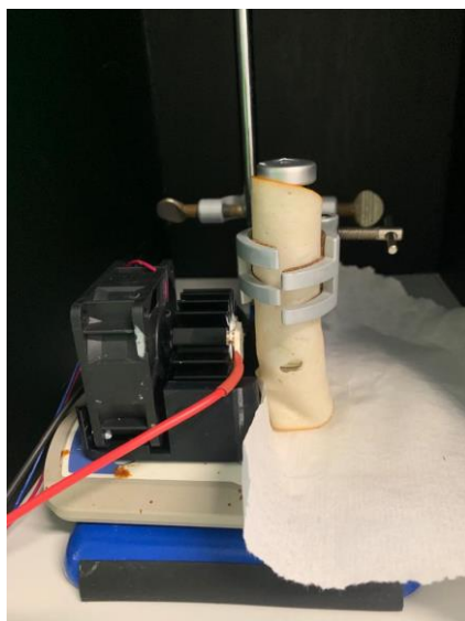
Figure S20. Setup of the photoreaction and folding of P1 through a tissue barrier. The sample vial is wrapped with a single slice of deli style chicken breast and irradiated with a red light LED ( \lambda_{\text{max}}=625 \text{ nm} )
