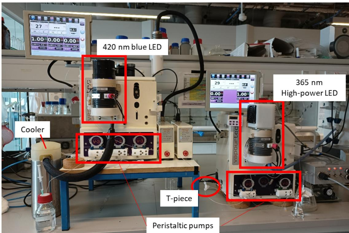
Image of dual flow coil (2 x 5 mL volume, PFA; filled with coloured solutions):
