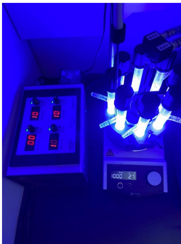
Figure S1. The Reaction Equipment and Light Source ( \lambda_{\text{max}} = 440 \text{ nm} , \Delta\lambda = 25 \text{ nm} )
