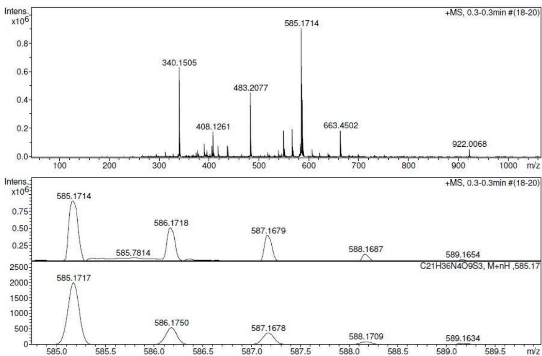
Figure S44: HRMS Spectra of NTASH compound
