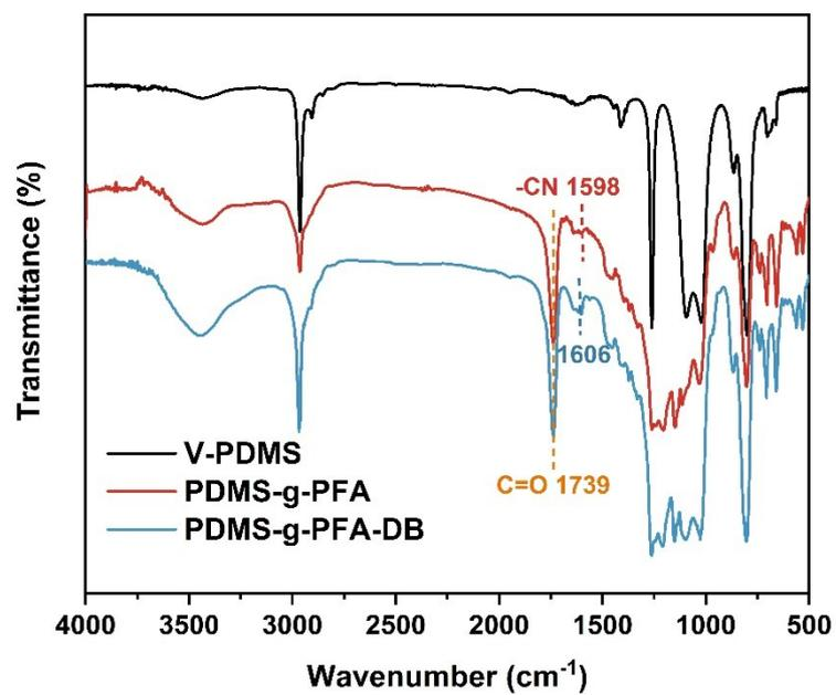
**Fig. S2** FTIR spectra of the V-PDMS, PDMS-g-PFA and PDMS-g-PFA-DB.
