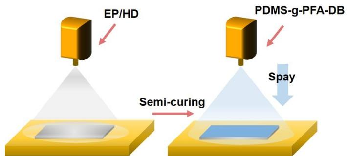
**Fig. S1** Fabrication route of EP/PDMS-g-PFA-DB.
