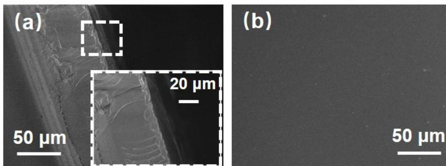
**Fig. S8** SEM images of (a) cross section and (b) surface for EP/PDMS-g-PFA-DB
