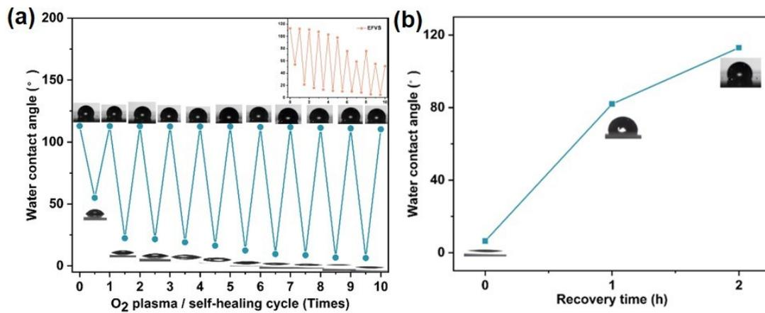
**Fig. S12** (a) reversible changes of CAs for EP/PDMS-g-PFA-DB during plasma/self-healing cycles; (b) plot of CA vs. recovery time for EP/PDMS-g-PFA-DB at 90 °C.
