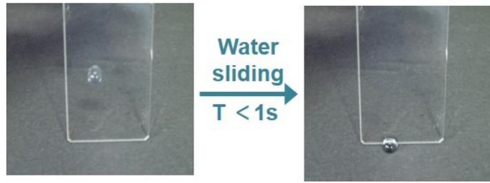
**Fig. S7** Snapshots of water sliding on EP/PDMS-g-PFA-DB with a tilt angle of 19°.
