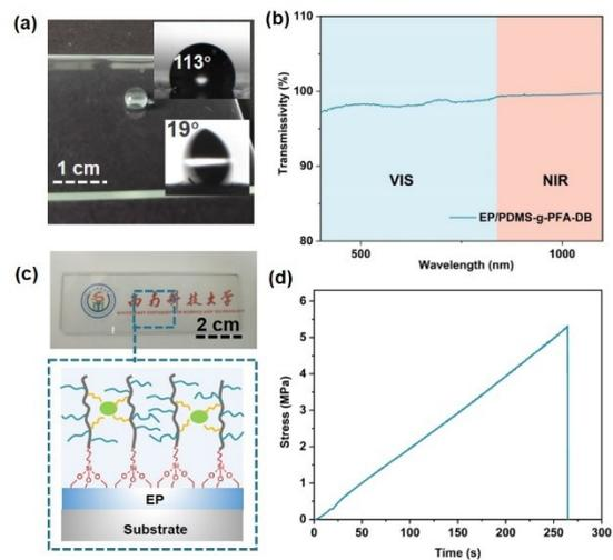
**Fig. S6** The CA and SA of EP/PDMS-g-PFA-DB; (b) the transmittance of EP/PDMS-g-PFA-DB in 400-1100 nm; (c) the anchoring groups enhance the adhesion of coating; (d) the adhesion strength of the EP/PDMS-g-PFA-DB coating
