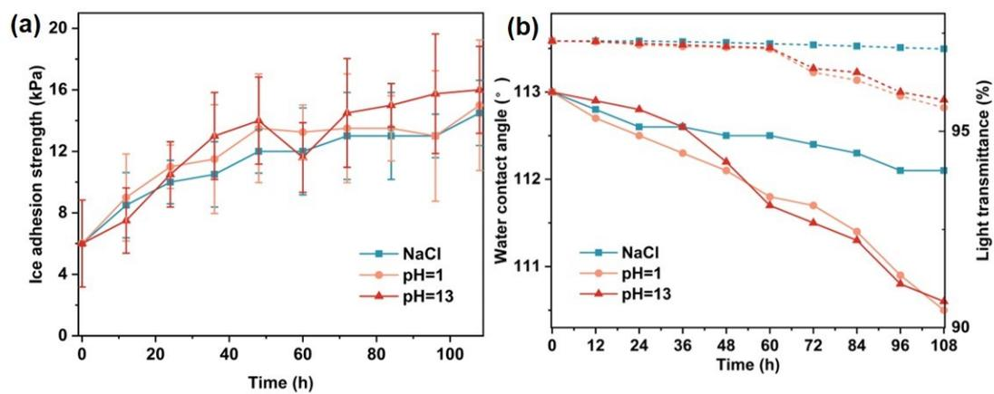
**Fig. S10** (a) ice adhesion strength, (b) CAs and light transmittance variations of EP/PDMS-g-PFA-DB in saturated sodium chloride solution, pH=1 sodium hydroxide solution and pH=13 hydrogen chloride solution.
