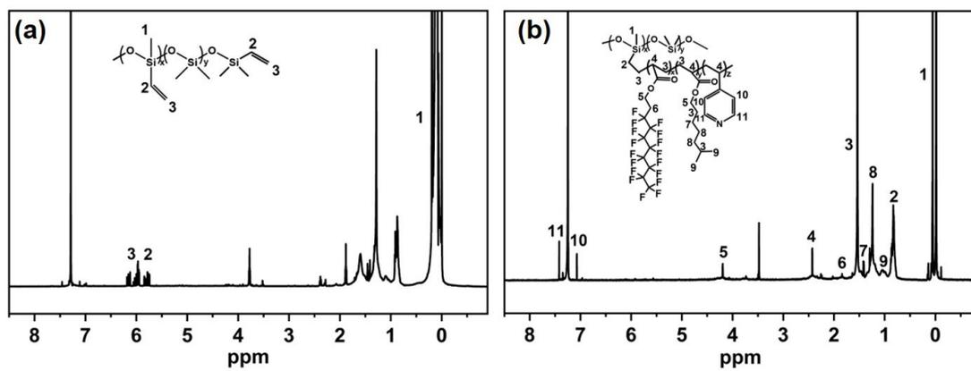
**Fig. S3**  $^1\text{H}$  NMR spectra of the (a) V-PDMS and (b) PDMS-g-PFA
