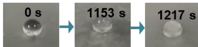
**Fig. S9** Static anti-icing optical photographs based on EP/PDMS-g-PFA-DB at -10.0 °C.
