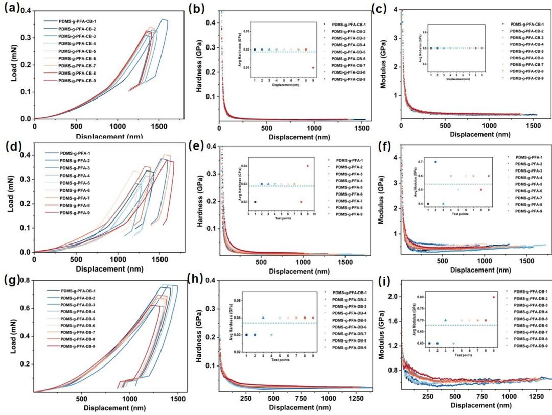
**Fig. S5** (a) Load-displacement curves, (b) hardness-displacement curves and (c) elastic modulus-displacement curves of EFVS; (d) load-displacement curves, (e) hardness-displacement curves and (f) elastic modulus-displacement curves of VEFVS; (g) load-displacement curves, (h) hardness-displacement curves and (i) elastic modulus-displacement curves of PDMS-g-PFA.
