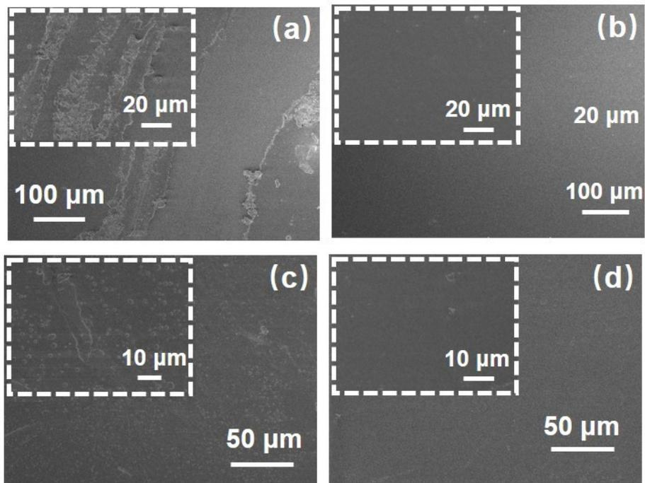
**Fig. S11** SEM images of EP/PDMS-g-PFA-DB (a) being damaged by de-icing abrasion ; (b) recovering at 90 °C for 30 min; (c) being impacting by sand and (d) recovering at 90 °C for 30 min.
