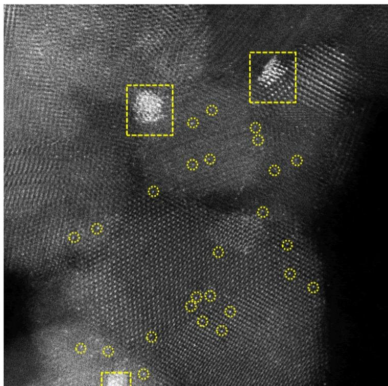
**Fig.S1** HAADF-STEM image of Pt-anchored CCO (squares represent the  $\text{PtO}_x$  clusters and the circles represent the Pt single atoms).
