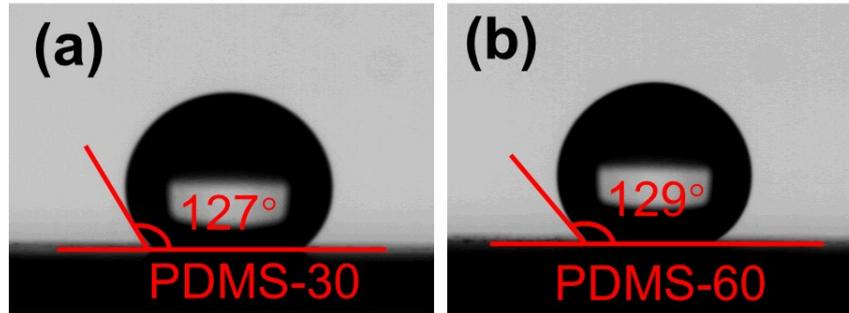
**Fig.S7** The contact angle of (a) PDMS-30 and (b) PDMS-60. (Note that the contact angle was measured on the porous CCO sensing layer on the alumina substrate.).
