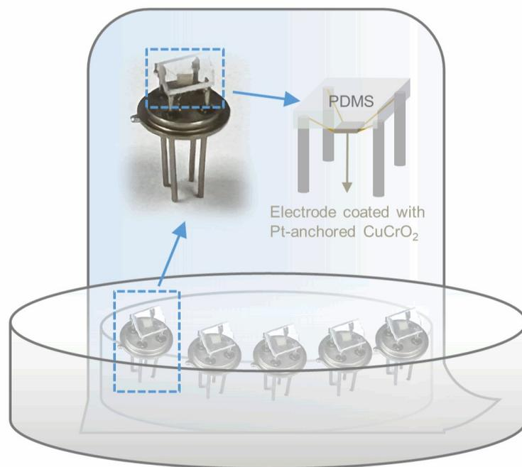
**Fig.S3** Schematic diagram of PDMS coating onto the chemiresistor devices by thermal evaporation.
