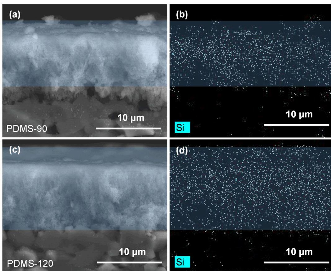
**Fig.S6** Cross-sectional SEM image of (a) PDMS-90 and (c) PDMS-120. Si element mapping of (b) PDMS-90 and (d) PDMS-120. Note that the porous CCO sensing layer was coated on the alumina substrate.
