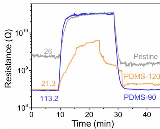
**Fig.S11** Response curve of Pristine, PDMS-90 and PDMS-120 to 5 ppm H<sub>2</sub>S at an operation temperature of 100 °C at RH 50% after 235 days.
