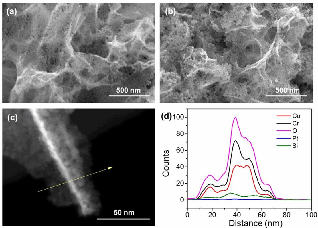
**Fig.S4** SEM images of (a) Pristine, (b) PDMS-90. (c-d) Elemental line-scanning profile of a single layer of PDMS-90 along cross section direction.
