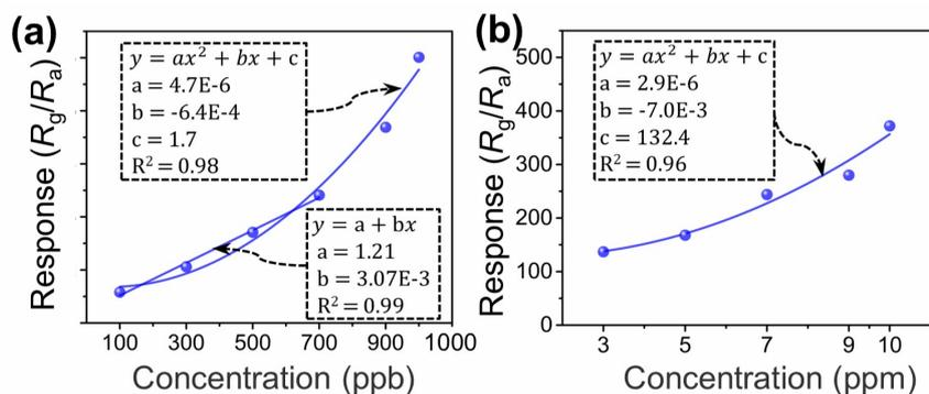
**Fig.S9** Response of PDMS-90 versus (a) 100–1000 ppb and (b) 3–10 ppm H<sub>2</sub>S at an operation temperature of 100 °C at RH 50%.
