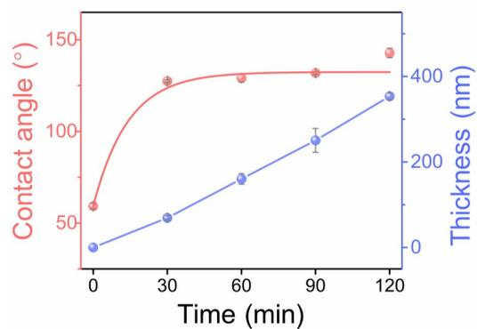
**Fig.S5** The variation of contact angle and the net PDMS film (deposited onto a flat surface alumina substrate) thicknesses of Pristine, PDMS-30, PDMS-60, PDMS-90, and PDMS-120 with PDMS deposition time. Note that the contact angle was measured on the chemiresistor surface (porous CCO sensing layer on the alumina sensing substrate).
