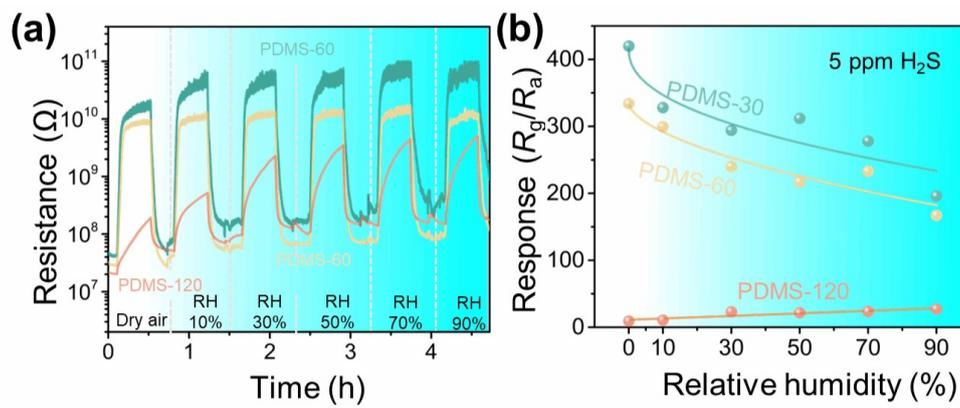
**Fig.S8** (a) The resistance and (b) response of PDMS-30, PDMS-60, and PDMS-120 to 5 ppm H<sub>2</sub>S under different relative humidity levels.
