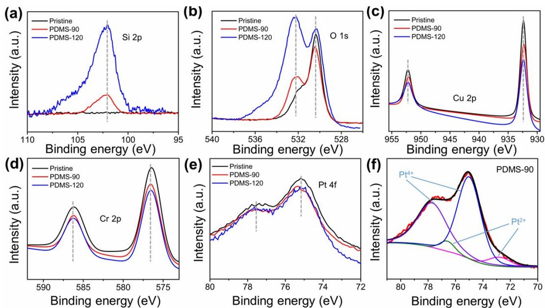
**Fig.S2** XPS spectra of (a) Si 2p, (b) O 1s, (c) Cu 2p, (d) Cr 2p, and (e) Pt 4f for Pristine, PDMS-90 and PDMS-120. (f) Pt 4f XPS spectrum of PDMS-90.
