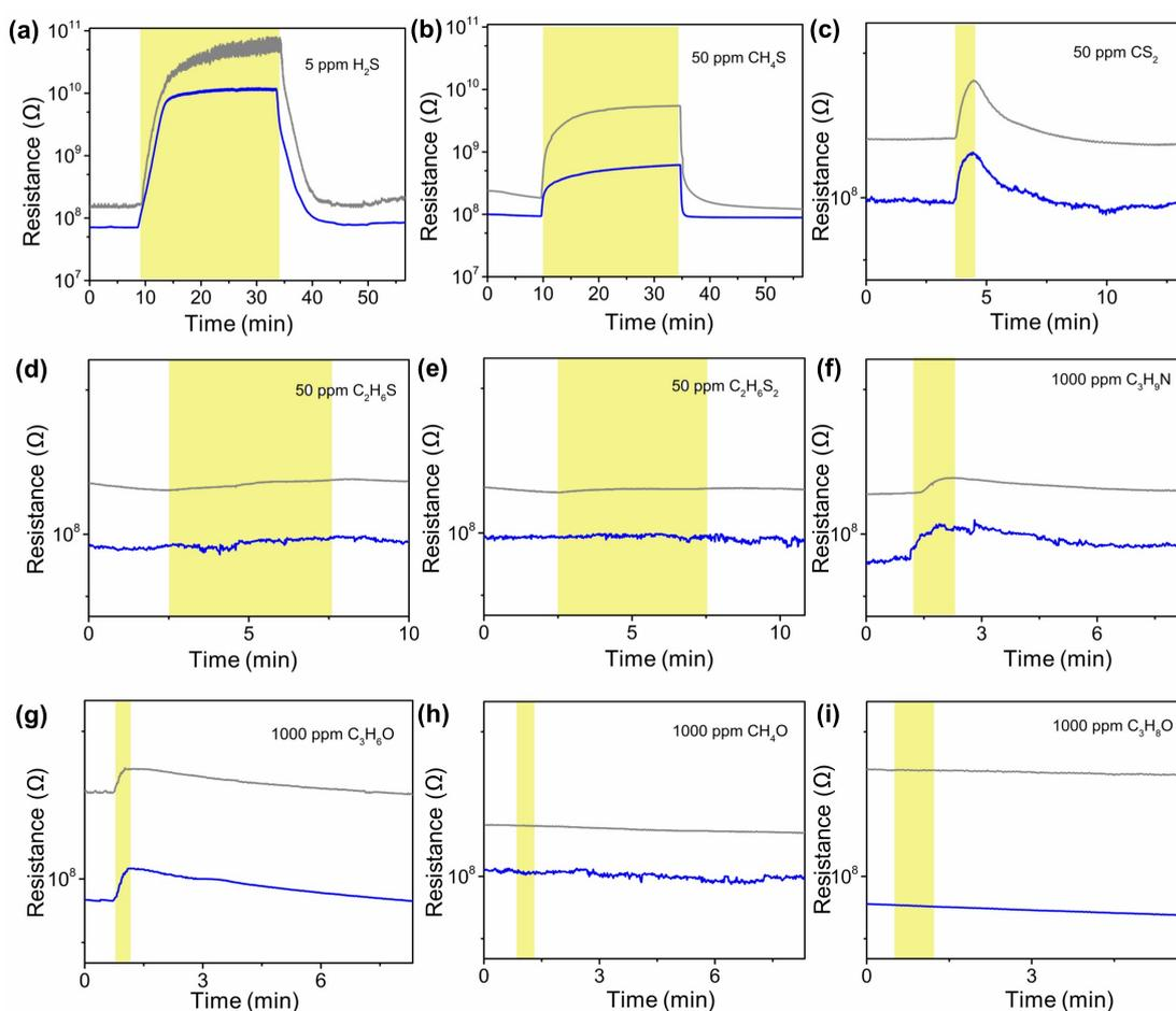
**Fig.S10** Response curve of PDMS-90 to different vapors at an operation temperature of 100 °C at RH 50%.
