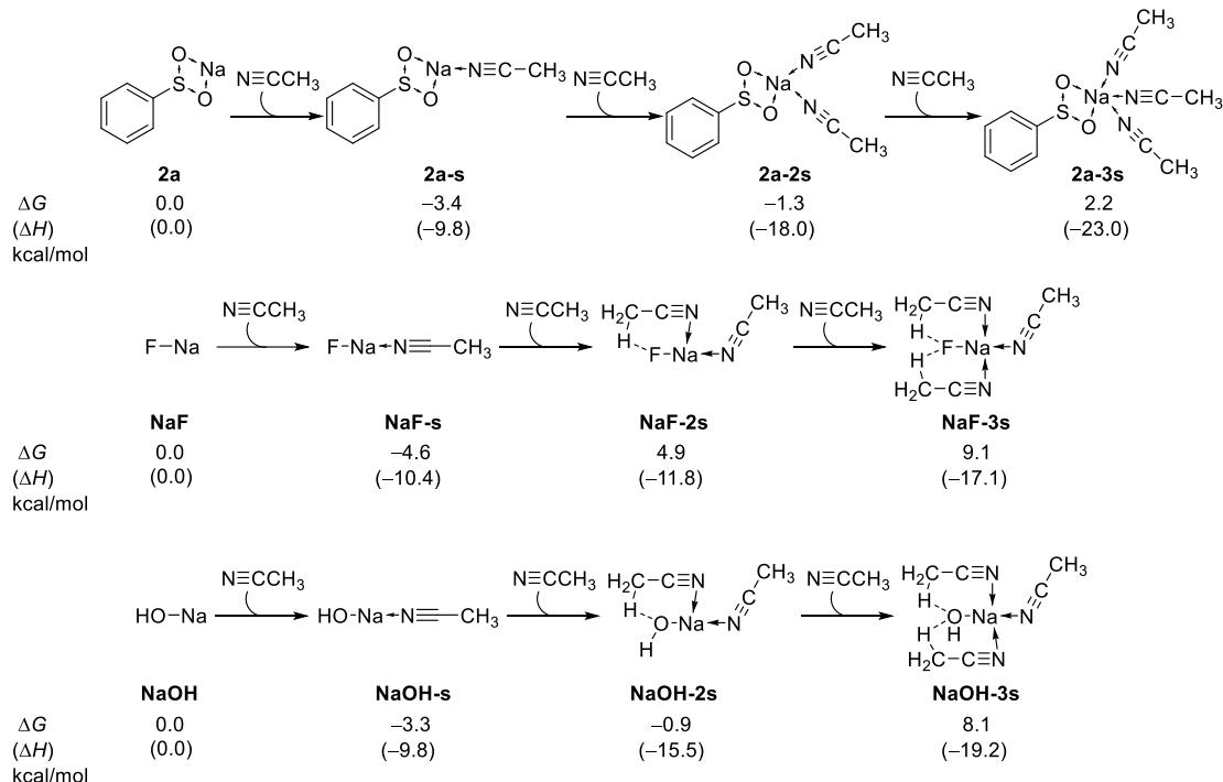
**Figure S1.** Calculated energy profiles of solvation energy of sodium salts with MeCN as solvent. All results were calculated at the M06-2X/6-31G(d) level of theory.
