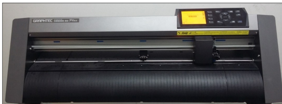
Figure S2. A) Photo of the cutter plotter (cutting speed 3 cm/s and cutting force for PVC foil 19 (out of 38 steps from 0.2 to 4.41 N). B) Display of laminator and values of speed (3 cm/min) and temperature (160 °C) parameters.
