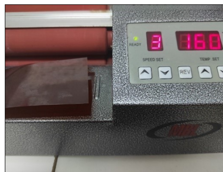
Figure S2. A) Photo of the cutter plotter (cutting speed 3 cm/s and cutting force for PVC foil 19 (out of 38 steps from 0.2 to 4.41 N). B) Display of laminator and values of speed (3 cm/min) and temperature (160 °C) parameters.
