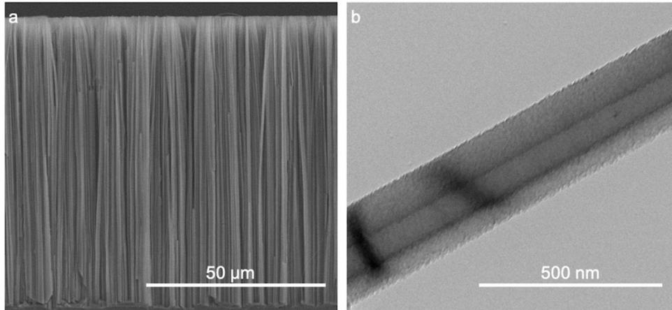
6 **Fig. S1** a) SEM image of the nanowire array cross-section; b) the TEM image of
