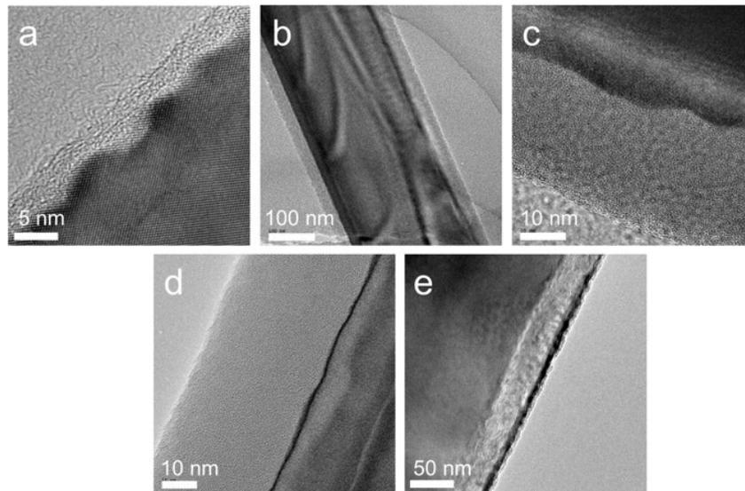
9 **Fig. S2.** The HRTEM of the single nanowire annealed at 900°C for 0 min (a), 25 min
