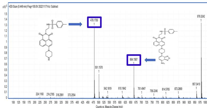
**Fig. S3.** ESI-HRMS spectrum of probe **ER-Nap-NBD** treated with  $\text{Na}_2\text{S}$ .
