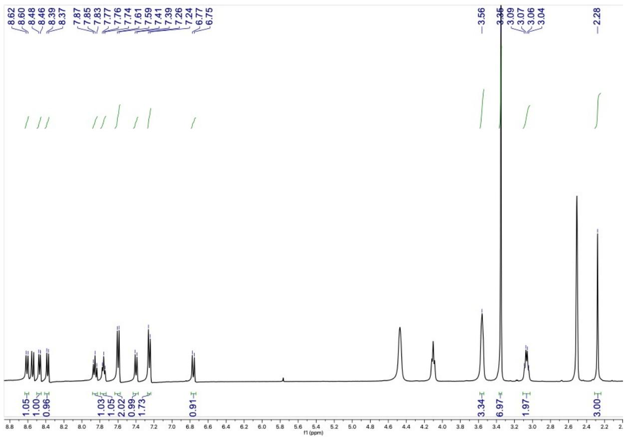
**Fig. S13.**  $^1\text{H-NMR}$  spectrum of ER-Nap-NBD in  $\text{DMSO-}d_6$ .
