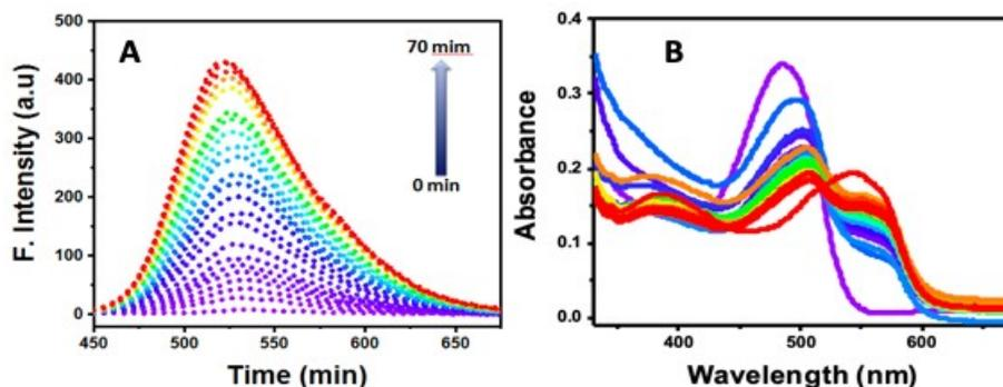
**Fig. S1.** (A) Time-function fluorescence of **ER-Nap-NBD** 10  $\mu\text{M}$  for the measurement of 1mM  $\text{Na}_2\text{S}$  for 70 min (B) UV-vis absorption spectra of **ER-Nap-NBD** (10  $\mu\text{M}$ ) upon addition of 0-1 mM  $\text{Na}_2\text{S}$  in EtOH-PBS (1:1, v/v, pH=7.4) solution.  $\lambda_{\text{Ex}}=400$  nm and  $\lambda_{\text{Em}}=530$  nm.
