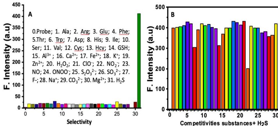
**Fig. S2.** (A) The selectivity test of probe **ER-Nap-NBD** (10  $\mu\text{M}$ ) to measure other chemicals (1 mM). (B) The competitiveness fluorescence signals of probe **ER-Nap-NBD** (10  $\mu\text{M}$ ) in the presence of 1 mM  $\text{H}_2\text{S}$  and other chemicals (1 mM) in solution.
