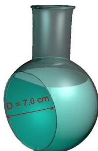
Fig. S15 Schematic illustration of the photoreactor used in our system for AQY measurement.
