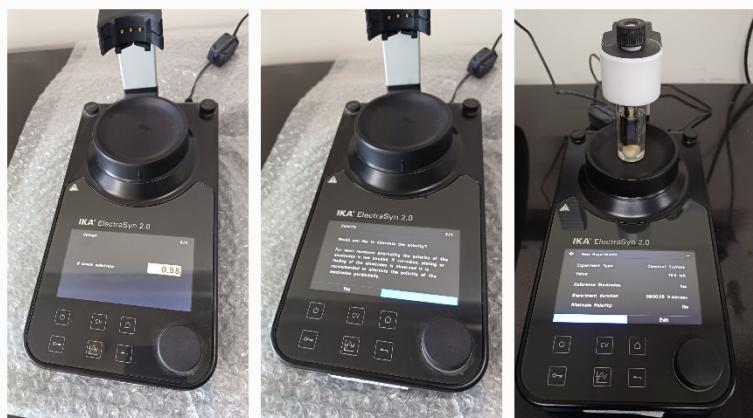
**Left:** Select “0.98 mmol” **Middle:** Alternate the polarity Chose “No” **Right:** Select “Start the experiment”
