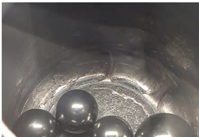
Figure S1. Lithium particles directly milled in hydrogen atmosphere.
