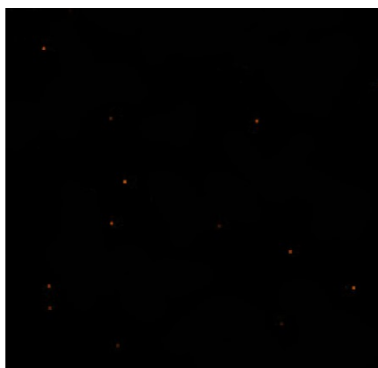
Fig. S5. The distribution of N on the surface of CNT-VP obtained from STEM-EDS mapping.
