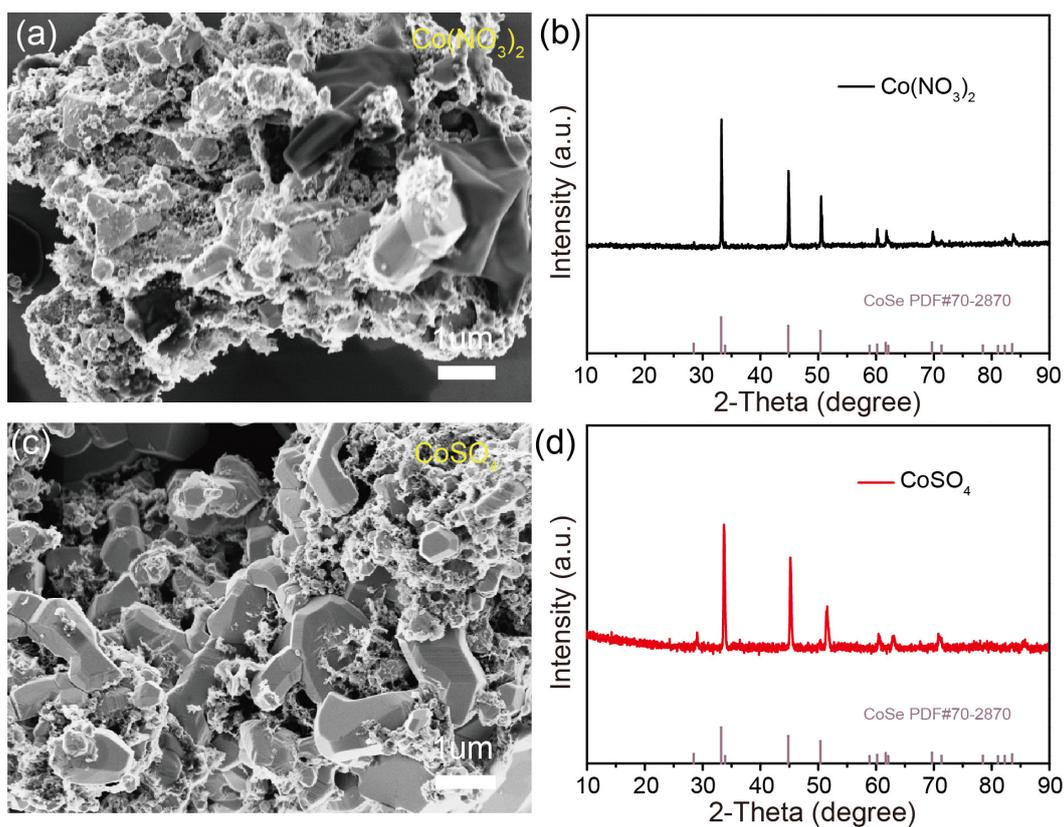
**Fig. S9** (a, c) SEM images of the pyrolyzed products using  $\text{Co}(\text{NO}_3)_2$  or  $\text{CoSO}_4$ . (b, d) XRD patterns of corresponding pyrolyzed products.
