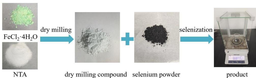
**Fig. S1** Scheme for scale-up synthesis of FeSe/NC catalyst, showing the weight of corresponding product.
