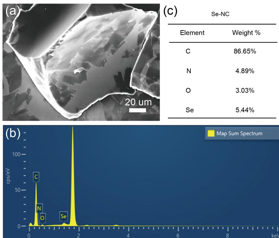
**Fig. S2** (a) SEM image, (b) EDS spectrum, and (c) elemental quantification of the Se-NC (pyrolyzed product using NTA and Se power as the precursors).
