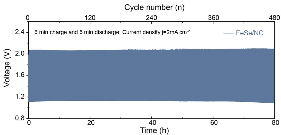
**Fig.S18** Cycling stability of the FeSe/NC-based Zn-air battery at a discharge/charge current density of  $2\text{ mA/cm}^2$ .
