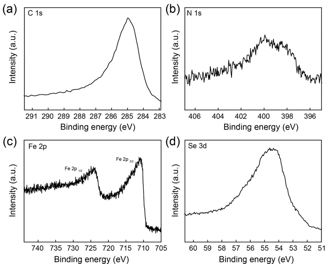
**Fig. S10** (a) C 1s, (b) N 1s, (c) Fe 2p, and (d) Se 3d XPS spectra of FeSe/NC.
