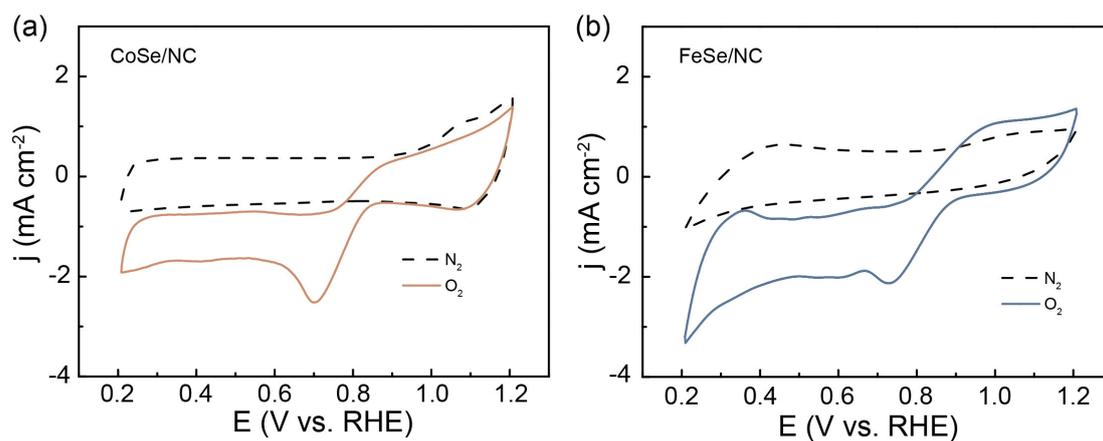
**Fig. S11** CV curves of (a) CoSe/NC and (b) FeSe/NC in  $N_2$ - or  $O_2$ -saturated 0.1M KOH solution.
