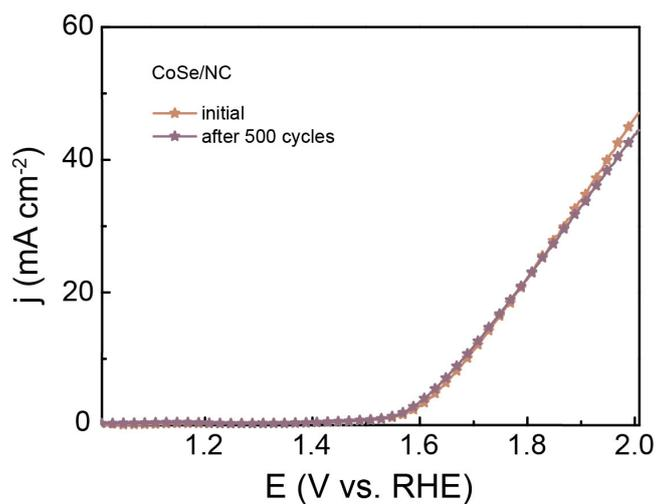
**Fig. S15** LSV curves of CoSe/NC for the OER before and after 500 CV cycles.
