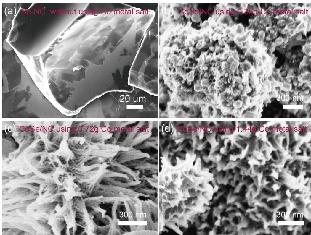
**Fig. S3** SEM images of (a) Se-NC without Co salt, (b) CoSe/NC using 0.36 g Co salt, (c) CoSe/NC using 0.72 g Co salt, and (d) CoSe/NC using 1.44 g Co salt.
