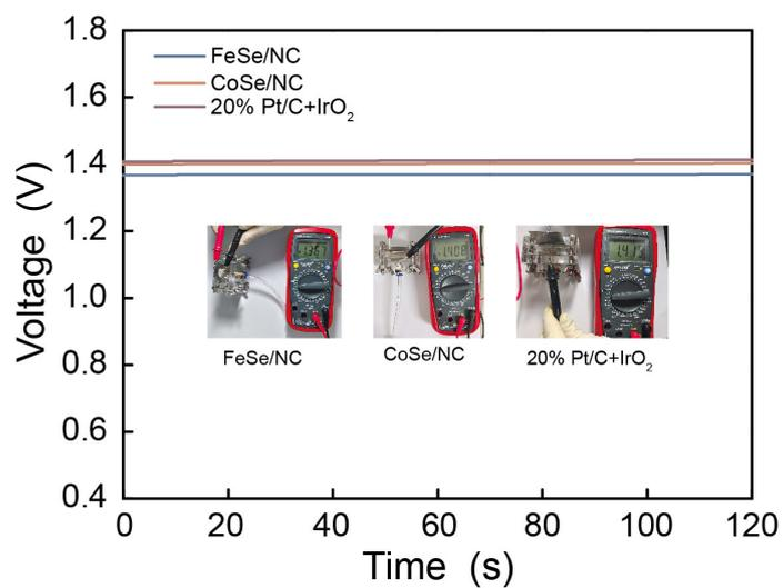
**Fig. S16** Open-circuit voltage of the Zn-air batteries based on CoSe/NC, FeSe/NC, and 20%Pt/C+IrO<sub>2</sub> (inset: direct voltage observation).
