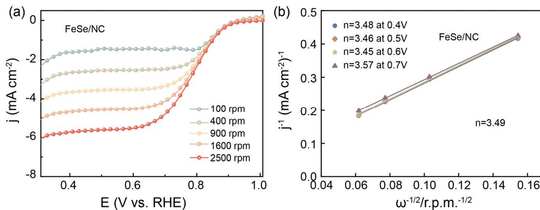
**Fig. S12** (a-b) LSV curves of FeSe/NC at various rotation speeds and its corresponding K-L plots at various potentials and the calculated electron transfer number.
