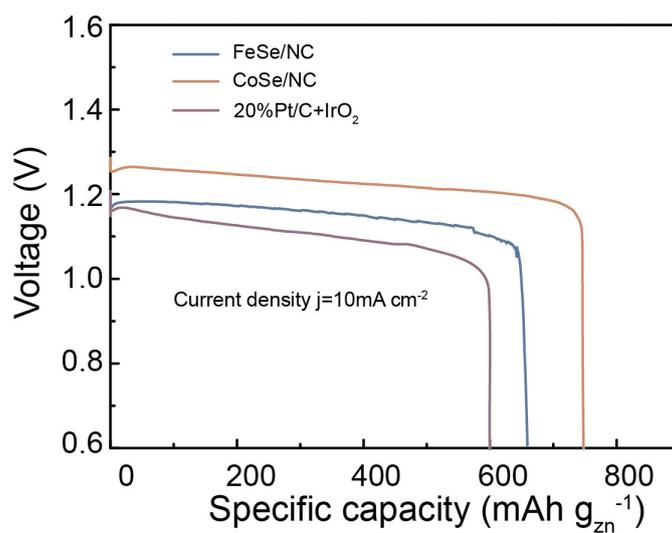
**Fig. S17** Specific capacities of the Zn-air batteries using CoSe/NC, FeSe/NC, and 20%Pt/C+IrO<sub>2</sub>.
