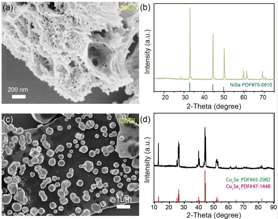
**Fig. S8** (a, c) SEM images of the pyrolyzed products using NiCl<sub>2</sub> or CuCl<sub>2</sub>. (b, d) XRD patterns of corresponding pyrolyzed products.
