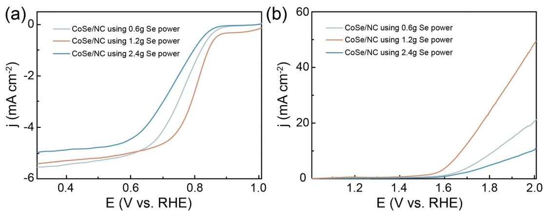
**Fig. S4** LSV curves record at 1600 rpm of CoSe/NC catalysts with different amounts of Se power, showing the ORR and OER activity.
