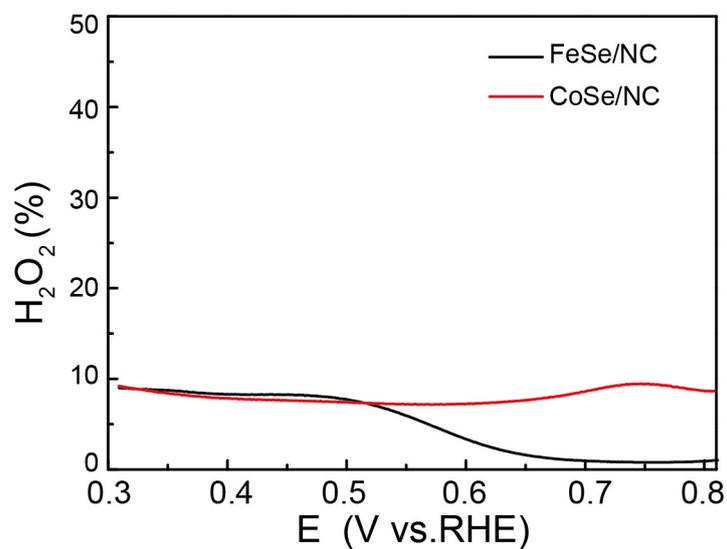
**Fig. S13**  $H_2O_2$  yield recorded with RRDE at a scan rate of 10 mV s<sup>-1</sup> and rotation speed of 1600 rpm.
