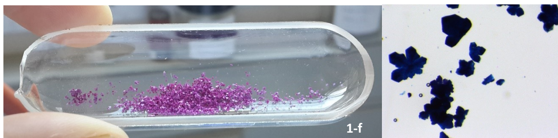
Fig. S31. Left: material after drying in a vacuum oven for 24 h at 85 °C ( 1-f ), the guest DMF has been removed. Right: blue crystals of 1 post TGA. The crystals after heating during TGA to 400 °C.
