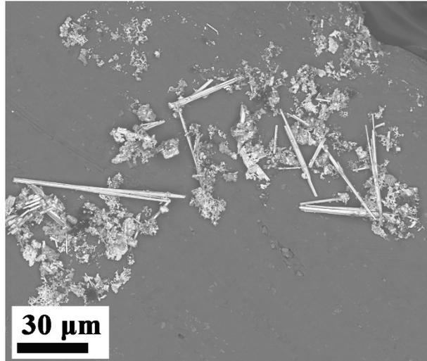
**Figure S4.** SEM image of the sample (H1Z1-14-C) synthesized by molten-salt-assisted BCTR method at 1400 °C for 180 min, with B<sub>4</sub>C as reducing agent.
