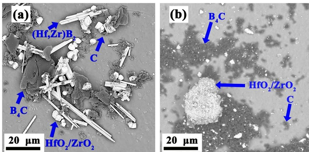
**Figure S3.** SEM images of samples (H1Z1-11-M and H1Z1-11-C) prepared at 1100 °C/ 20 min by either (a) microwave-assisted or (b) molten-salt-assisted BCTR method.
