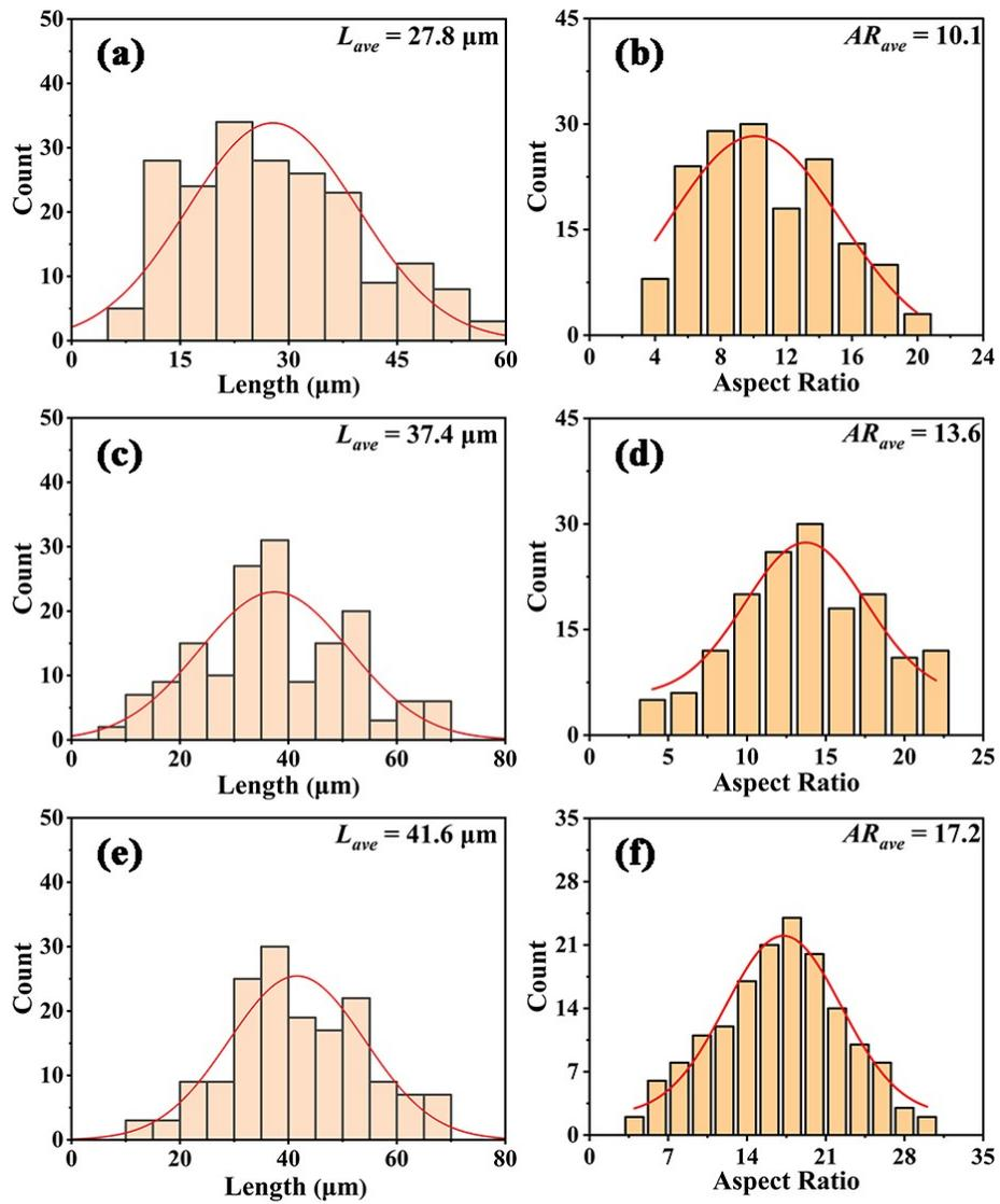
**Figure S1.** Histograms of (a, c, e) length and (b, d, f) aspect-ratio of  $(\text{Hf}_x\text{Zr}_{1-x})\text{B}_2$  ( $x = 0.25, 0.50$  and  $0.75$ ) particles in the samples (H1Z3-11, H1Z1-11 and H3Z1-11) synthesized by MSM-BCTR method at  $1100^\circ\text{C}/20$  min, respectively.
