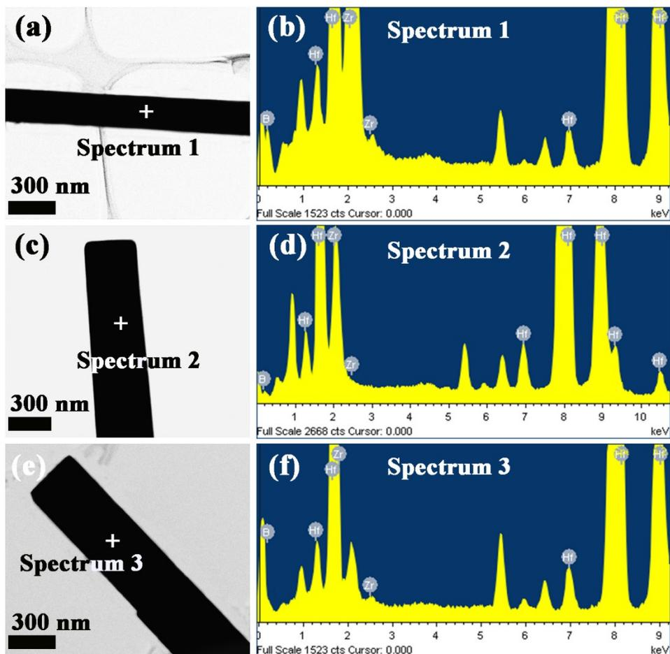
**Figure S2.** (a, c, d) Low-resolution TEM images and (b, d, f) EDS-dotting spectra of the rod-like  $(\text{Hf}_x\text{Zr}_{1-x})\text{B}_2$  crystals ( $x = 0.25, 0.50$  and  $0.75$ ) synthesized by MSM-BCTR method.
