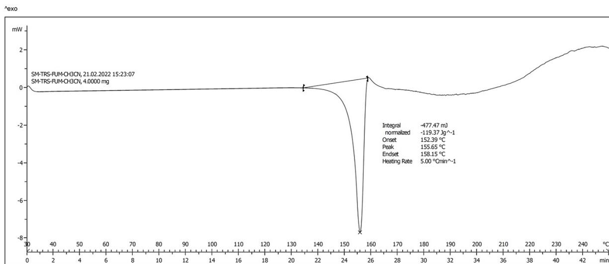
**Figure S15.** DSC thermogram of torasemide fumarate (TRS-FUM) salt (1:1) recorded at heating rate of 5°C/min from RT to 250°C. It shows a single melting endothermic event ( $T_{\text{onset}}$  at  $152.3 \pm 0.2^\circ\text{C}$ ,  $T_{\text{peak}}$  at  $155.6^\circ\text{C} \pm 0.2^\circ\text{C}$ ,  $T_{\text{endset}}$  at  $158.1 \pm 0.2^\circ\text{C}$ , Heat of fusion value of  $119.3 \pm 0.5 \text{ J/g}$ ).
