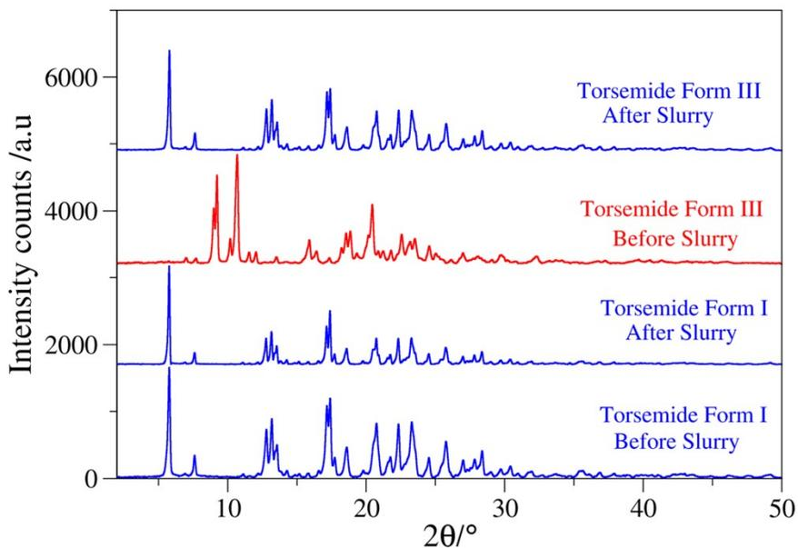
**Figure S19.** Slurry experiments of Torasemide in water. Torasemide form I remained stable after 24 hours of slurry, while Torasemide T-III/T-N converted to Torasemide form I, as indicated by changes in the powder X-ray diffraction pattern.
