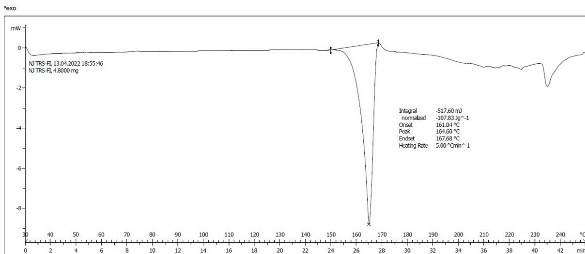
**Figure S13.** DSC thermogram of polymorph T-I of torasemide recorded at heating rate of 5°C/min from RT to 250°C. It shows a single melting endothermic event ( $T_{\text{onset}}$  at 161.0±0.2°C,  $T_{\text{peak}}$  at 164.6°C ±0.2°C,  $T_{\text{endset}}$  at 167.7±0.2°C, Heat of fusion value of 107.8±0.5 J/g).
