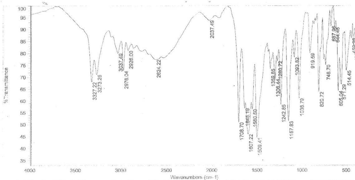
**Figure S11.** The FT-IR spectrum of torasemide oxalate (TRS-OX) salt (2:1).
