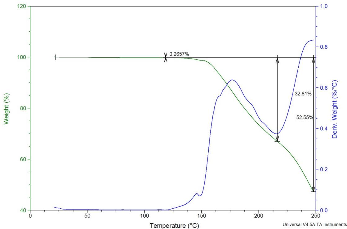
**Figure S18.** TGA plot of torasemide oxalate (TRS-FUM) salt (2:1) recorded at heating rate of 5°C/min from RT to 250°C. It shows a weight loss of 0.26% from RT to 100°C.
