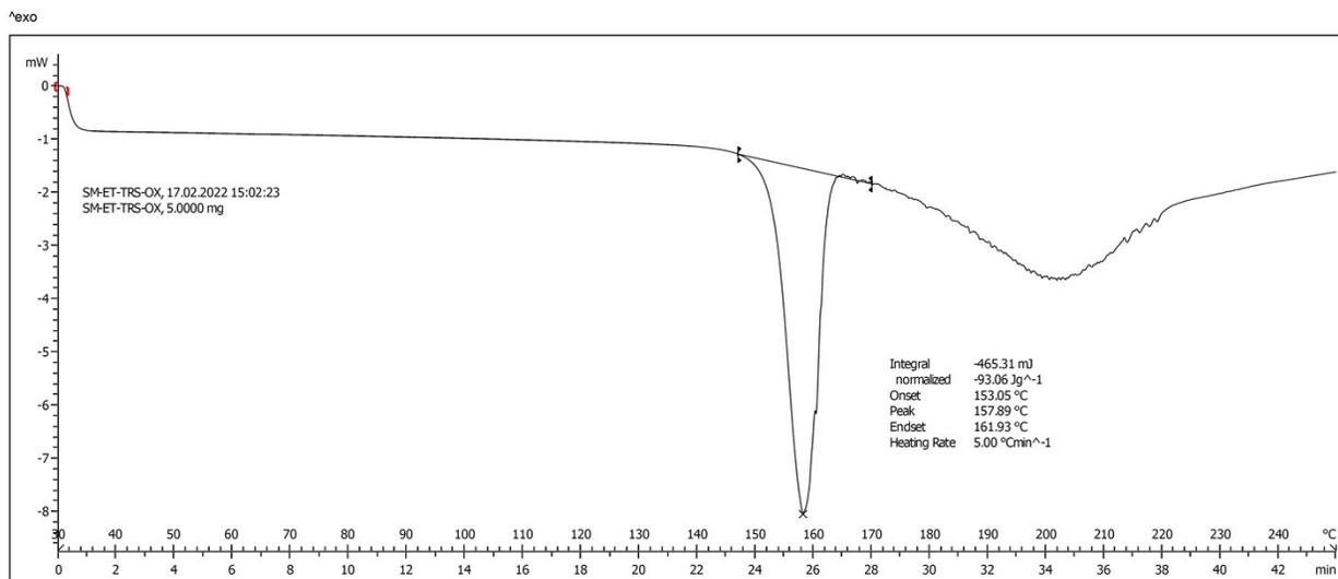
**Figure S16.** DSC thermogram of torasemide oxalate (TRS-OX) salt (2:1) recorded at heating rate of 5°C/min from RT to 250°C. It shows a single melting endothermic event ( $T_{\text{onset}}$  at 153.0±0.2°C,  $T_{\text{peak}}$  at 157.8°C ±0.2°C,  $T_{\text{endset}}$  at 161.9±0.2°C, Heat of fusion value of 93.0±0.5 J/g).
