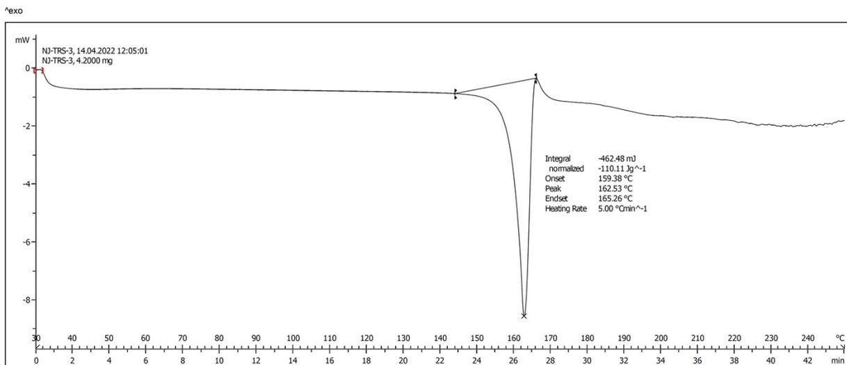
**Figure S14.** DSC thermogram of polymorph T-III/T-N of torasemide recorded at heating rate of 5°C/min from RT to 250°C. It shows a single melting endothermic event ( $T_{\text{onset}}$  at  $159.3 \pm 0.2^\circ\text{C}$ ,  $T_{\text{peak}}$  at  $162.5^\circ\text{C} \pm 0.2^\circ\text{C}$ ,  $T_{\text{endset}}$  at  $165.2 \pm 0.2^\circ\text{C}$ , Heat of fusion value of  $110.1 \pm 0.5 \text{ J/g}$ ).
