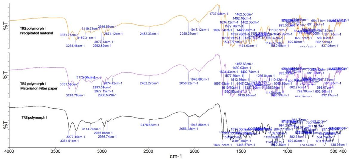
**Figure S20.** Slurry experiments of torasemide in water. Torasemide Form I remained stable after 24 hours of slurry.
