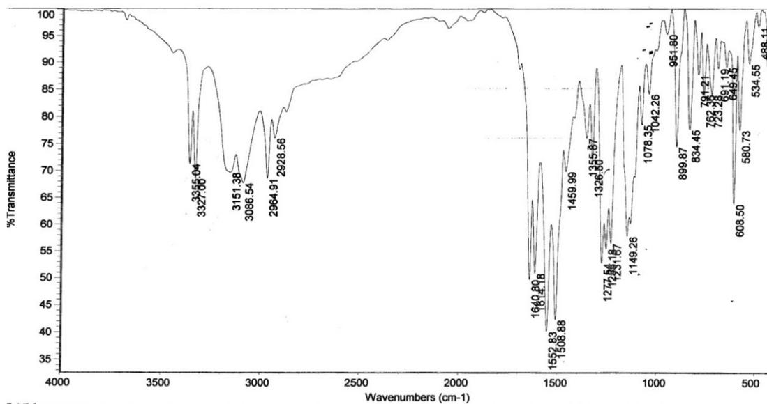
Figure S9. The FT-IR spectrum of polymorph T-III/T-N of torasemide.
