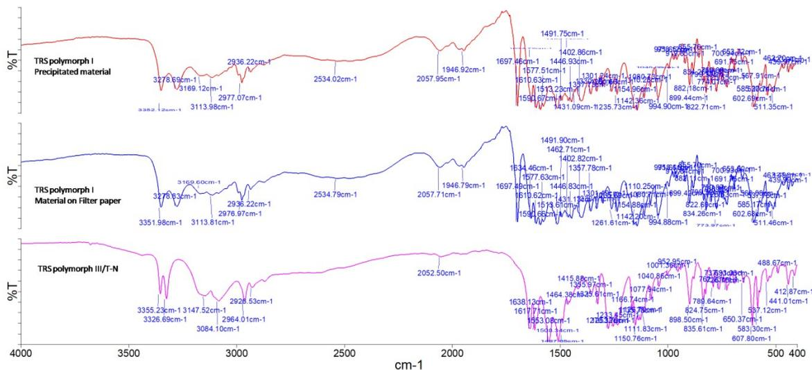
**Figure S21.** Slurry experiments of torasemide in water. Torasemide form III/T-N transformed to T-I after 24 hours of slurry.
