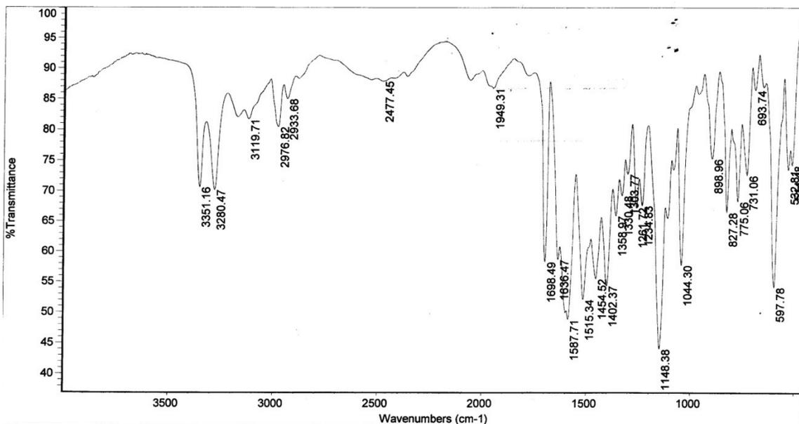
Figure S8. The FT-IR spectrum of polymorph T-I of torasemide.
