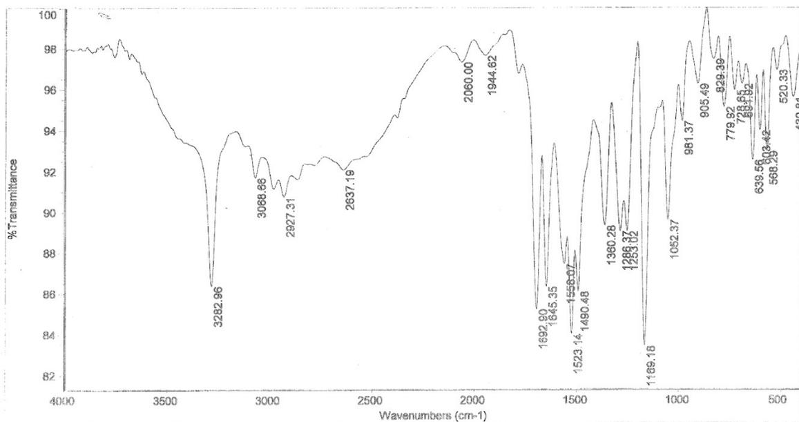
**Figure S10.** The FT-IR spectrum of torasemide fumarate (TRS-FUM) salt (1:1).
