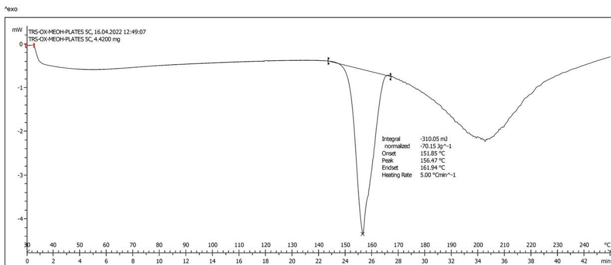
**Figure S17.** DSC thermogram of torasemide oxalate methanolate (TRS-OX-M) salt (2:1:0.56) recorded at heating rate of 5°C/min from RT to 250°C. It shows a single melting endothermic event ( $T_{\text{onset}}$  at 151.8±0.2°C,  $T_{\text{peak}}$  at 156.4°C ±0.2°C,  $T_{\text{endset}}$  at 161.9±0.2°C, Heat of fusion value of 70.1±0.5 J/g).
