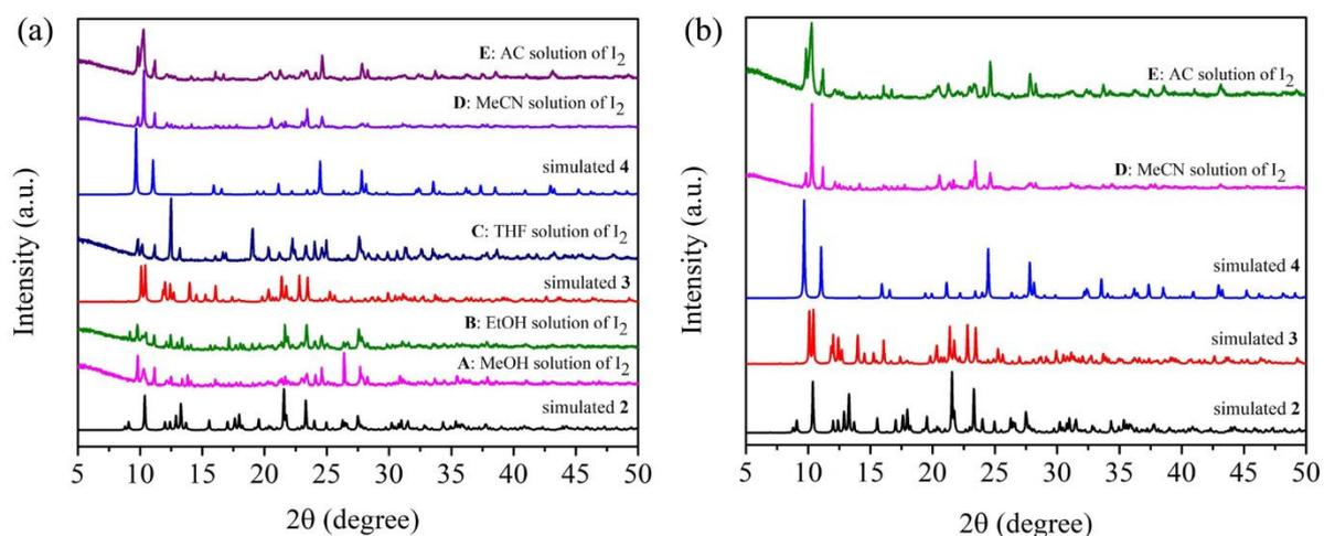
**Fig. S4** PXRD patterns of the final products synthesized by using CdI<sub>2</sub> and phen as precursors in I<sub>2</sub> solutions compared with the simulated patterns of complexes **2-4**.
