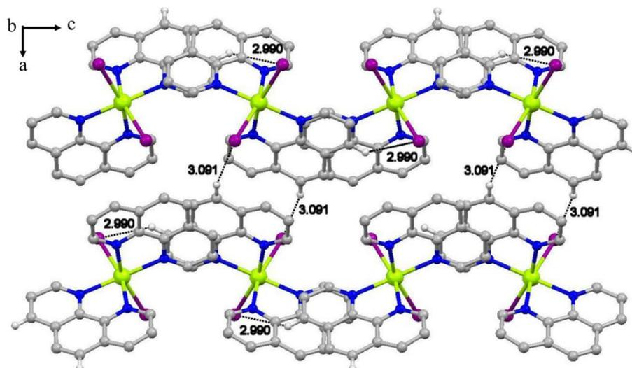
**Fig. S9** 3D supramolecular framework of **9** stabilized by weak I...H interactions with distances of 3.091 Å for I1...H16A and 2.990 Å for I1...H9A.<sup>1</sup>
