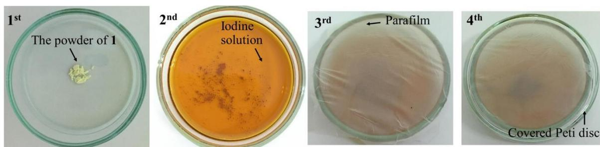
**Fig. S3** Experimental set up for following the DRST process. The ground powder of **1** (10 mg) was firstly placed into the Petri disc. Then, 6 mL of iodine solution was added. Parafilm was used to cover the reaction first, then closed by another Petri disc. All covers were removed at different time intervals, and the image of crystal growth was immediately captured under an optical microscope.
