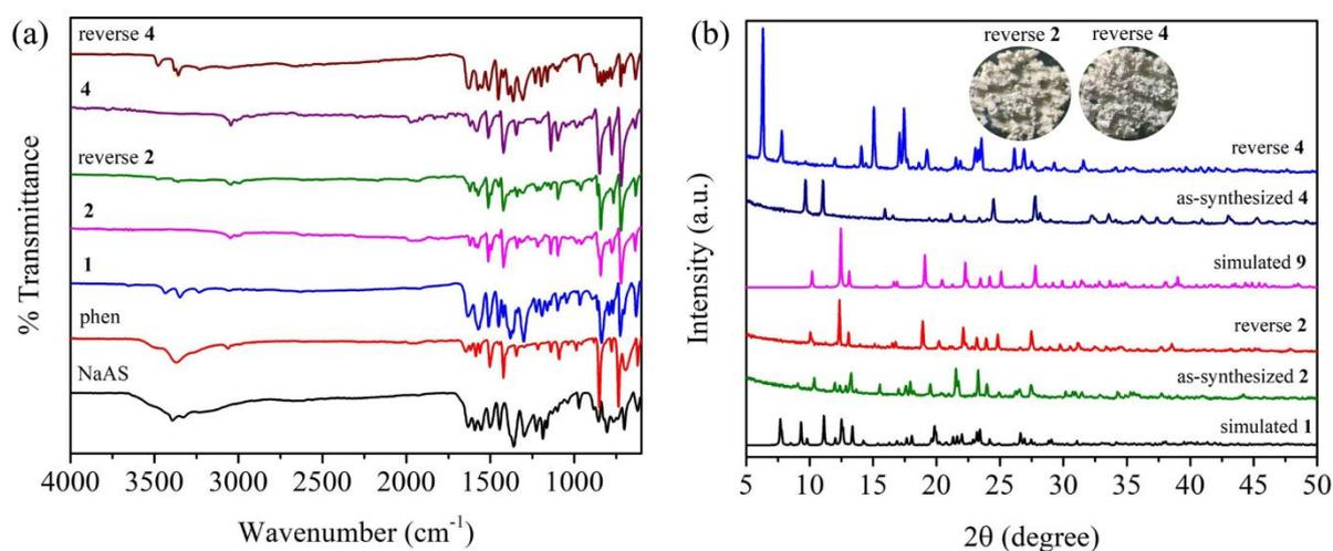
**Fig. S10** (a) FT-IR spectra, and (b) PXRD patterns of **2** and **4** after reverse experiments.
