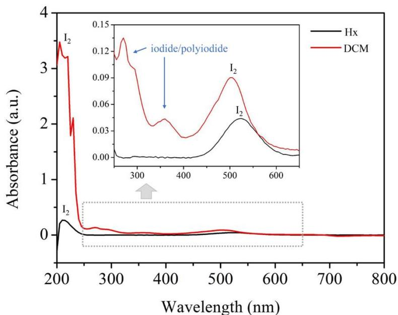
**Fig. S7** UV-vis spectra of hexane (Hx) and dichloromethane (DCM) solutions of iodine. The absorption bands appear around 204 and 500-520 nm belong to the neutral  $I_2$  molecules, and the bands at 288 and 360 nm are attributed to the iodide/polyiodide ions.
