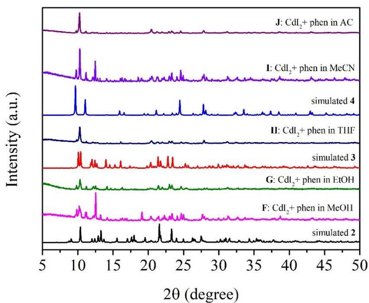
**Fig. S5** PXRD patterns of the final products synthesized by using CdI<sub>2</sub> and phen as precursors in different pure solvents compared with the simulated patterns of complexes **2-4**.
