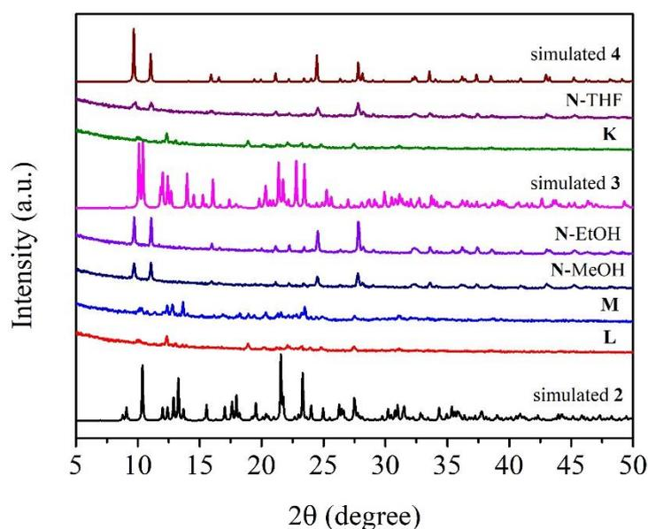
**Fig. S6** PXRD patterns of the final products synthesized by using the starting complexes without AS ligand in I<sub>2</sub> solutions compared with the simulated patterns of complexes **2-4**.
