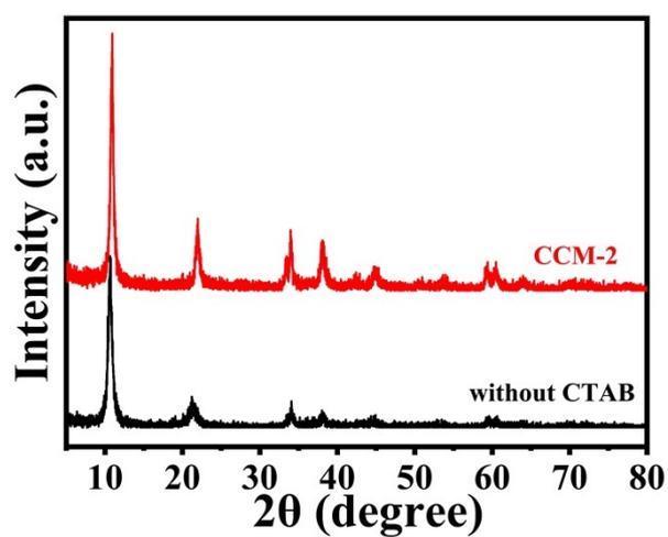
**Fig. S5** XRD patterns of the CCM-2 with and without CTAB.
