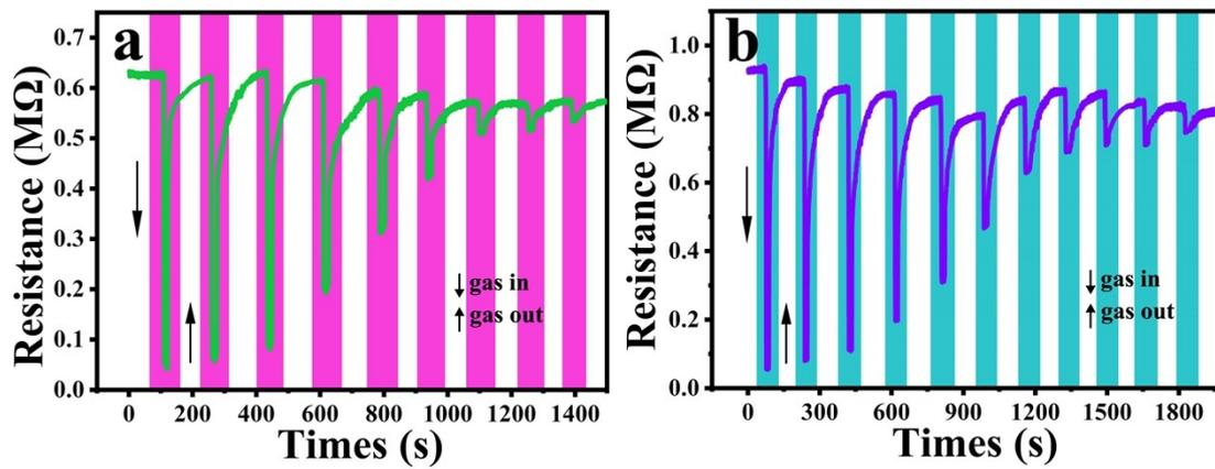
**Fig. S7** The dynamical response/recovery transient curves of (a) CCM-1 sensor to 100-0.3 ppm NO<sub>2</sub> and (b) CCM-3 sensor to 100-0.05 ppm NO<sub>2</sub>.
