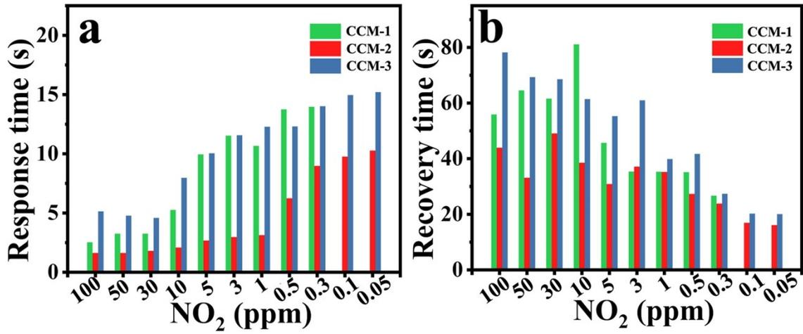
Fig. S8 (a) Response time and (b) recovery time of the CCM-1, CCM-2 and CCM-3 sensor, respectively.
