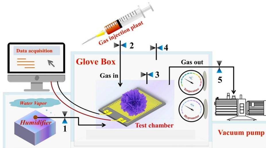
**Fig. S1** The diagram of the gas delivery system for the gas sensing process.
