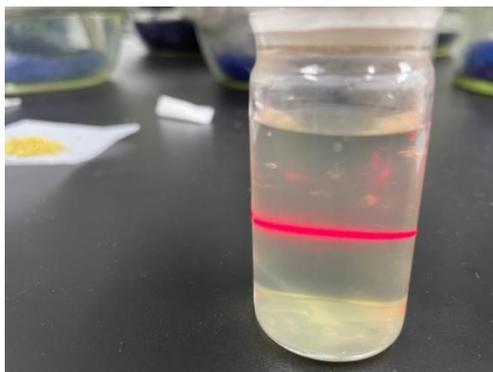
Fig. S2 The Tyndall effect of the CCM-2 colloidal solution.
