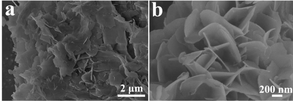
**Fig. S6** SEM images of CCM-2 (a) with and (b) without CTAB.
