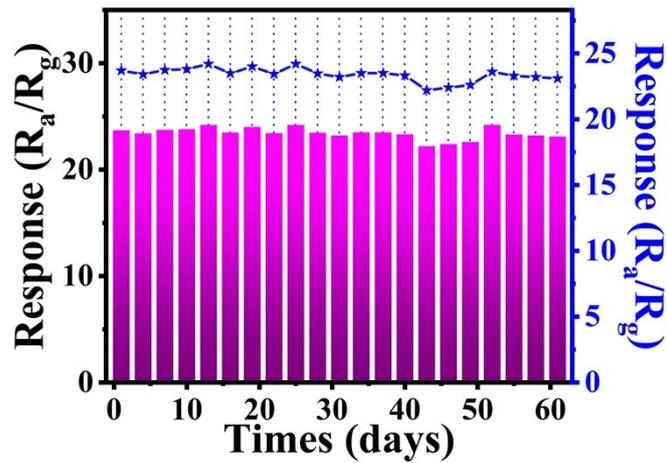
Fig. S9 The stability of the CCM-2 sensor to 100 ppm NO<sub>2</sub> for 60 days at RT.
