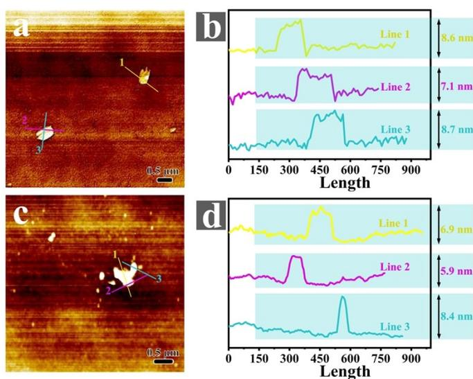
Fig. S3 AFM images and height profiles of CCM-1 (a, b) and CCM-3 (c, d)
