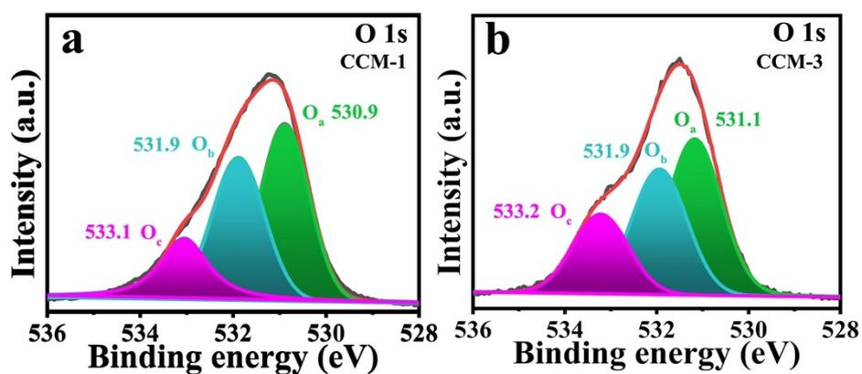
Fig. S4 O 1s high-resolution XPS survey spectra of (a) CCM-1 and (b) CCM-3, respectively.
