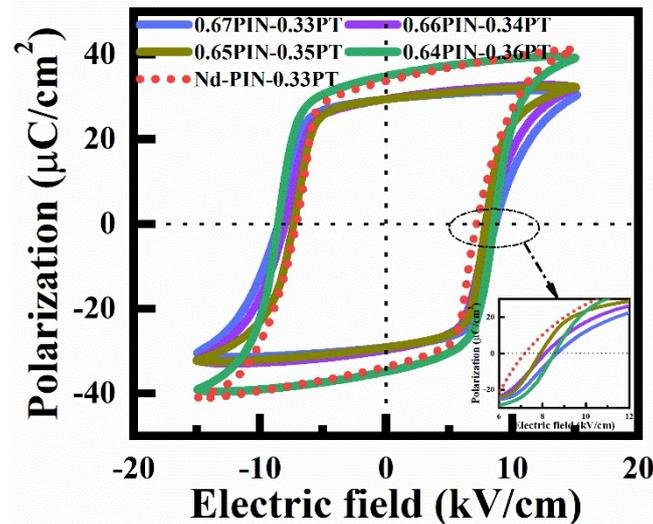
**FIG. S2** The comparison of  $P$ - $E$  hysteresis loops of  $[001]_c$ -oriented PIN-PT and Nd-PIN-0.33PT crystals at room temperature.
