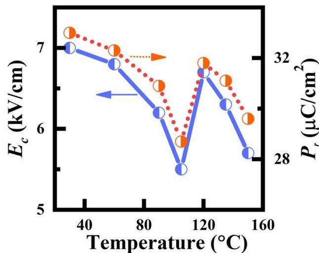
**FIG. S4** Temperature dependence of  $E_c$  and  $P_r$  of  $[001]_c$ -oriented Nd-PIN-0.33PT crystals.
