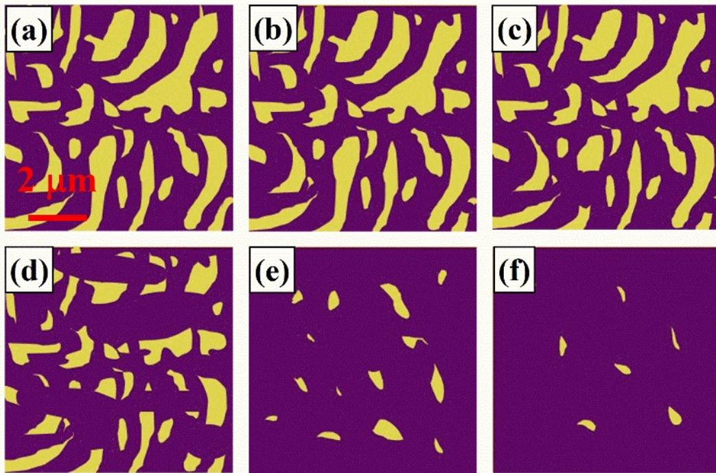
**FIG. S5** The out-of-plane domain images of  $[001]_c$ -oriented Nd-PIN-0.33PT crystals as a function of temperature (a) 30 °C, (b) 60 °C, (c) 90 °C, (d) 120 °C, (e) 150 °C, (f) 180 °C.
