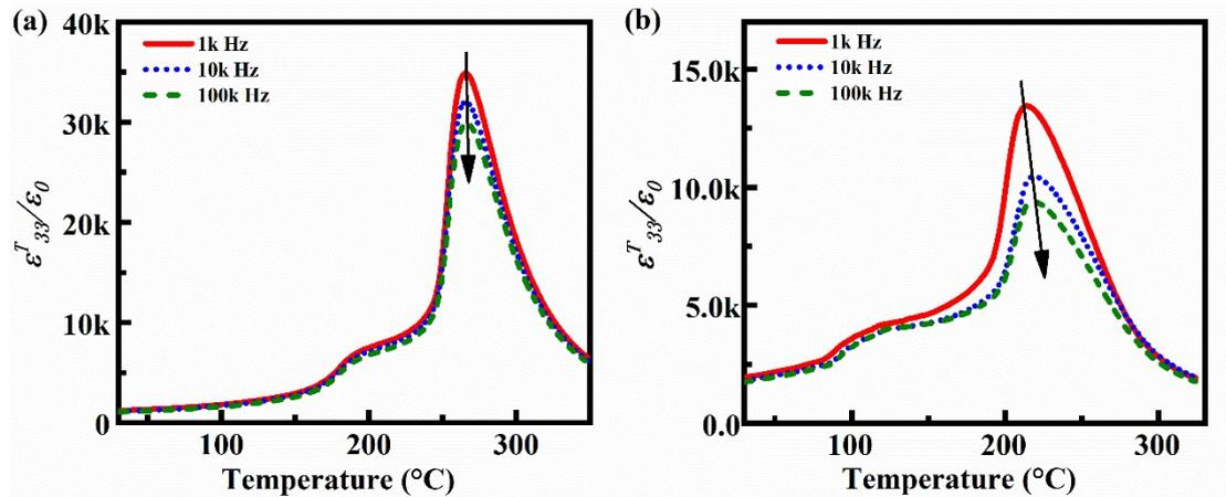
**FIG. S3** Temperature dependence of  $\varepsilon_{33}^T/\varepsilon_0$  of unpoled  $[001]_c$ -oriented (a) PIN-0.33PT and (b) Nd-PIN-0.33PT crystals.
