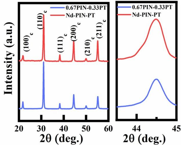
**FIG. S1** The powder XRD patterns of PIN-0.33PT and Nd-PIN-0.33PT single crystals.
