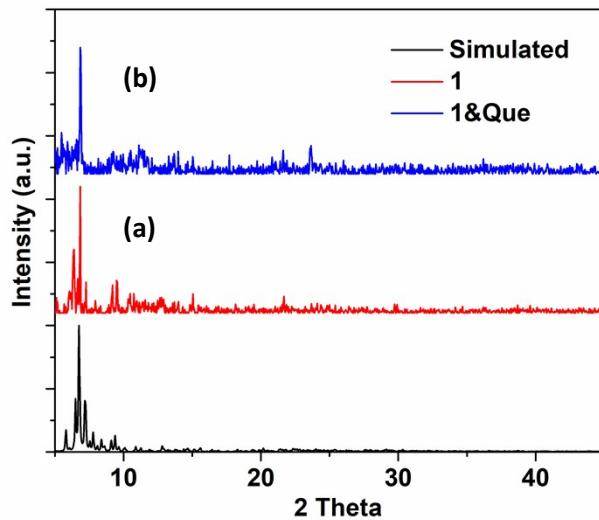
**Figure S4.** Powder XRD patterns of 1 before (a) and after (b) treated with Que.
