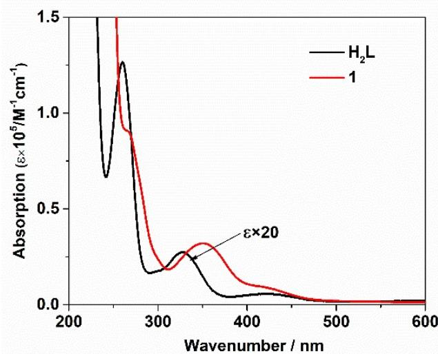
**Figure S5.** UV-vis absorption spectra of the free ligand H<sub>2</sub>L and **1** in CH<sub>3</sub>CN.
