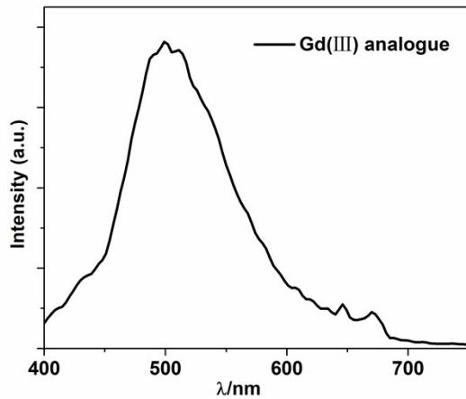
**Figure S12.** The phosphorescence spectrum of the Gd(III) analogue ( $10 \mu\text{M}$ ) at 77 K. ( $\lambda_{\text{ex}} = 367 \text{ nm}$ )
