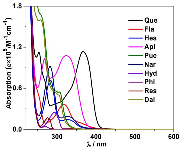
**Figure S13.** The UV-vis absorption spectra of analytes in  $\text{CH}_3\text{CN}$  at room temperature.
