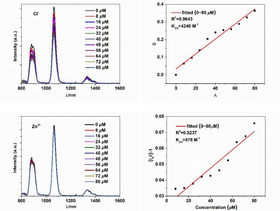
**Figure S9.** The NIR luminescent sensing of **1** (10  $\mu\text{M}$ ) to analytes in  $\text{CH}_3\text{CN}$ . ( $\lambda_{\text{ex}} = 371 \text{ nm}$ )
