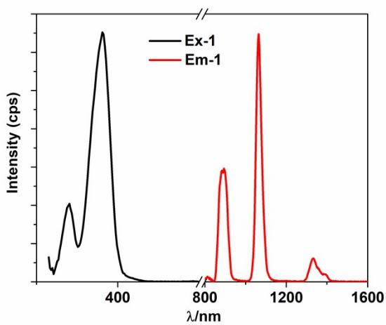
**Figure S7.** The excitation ( $\lambda_{\text{em}} = 1064 \text{ nm}$ ) and NIR luminescence ( $\lambda_{\text{ex}} = 371 \text{ nm}$ ) spectra of **1** ( $10 \mu\text{M}$ ) in  $\text{CH}_3\text{CN}$ .
