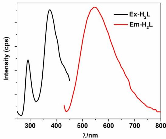
**Figure S6.** The excitation ( $\lambda_{em} = 643$  nm) and visible emission ( $\lambda_{ex} = 368$  nm) spectra of the free ligand H<sub>2</sub>L in CH<sub>3</sub>CN.
