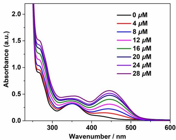
**Figure S11.** UV-vis titration of **1** ( $10 \mu\text{M}$ ) to the addition of Que in  $\text{CH}_3\text{CN}$ .
