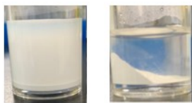
Figure S3. Photographic images of water dispersions of \text{NaNbO}_3\text{-Me} (line) and \text{NaNbO}_3\text{-(1Me+10Et)} (right).
