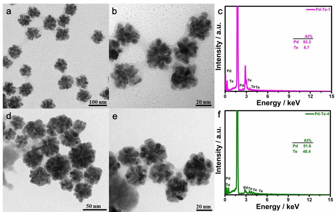
**Fig.S2** Representative TEM images of the (a, b) Pd-Te-1 NCs and (d, e) Pd-Te-4 NCs. SEM-EDS spectra of the Pd-Te-1 NCs and Pd-Te-4 NCs.
