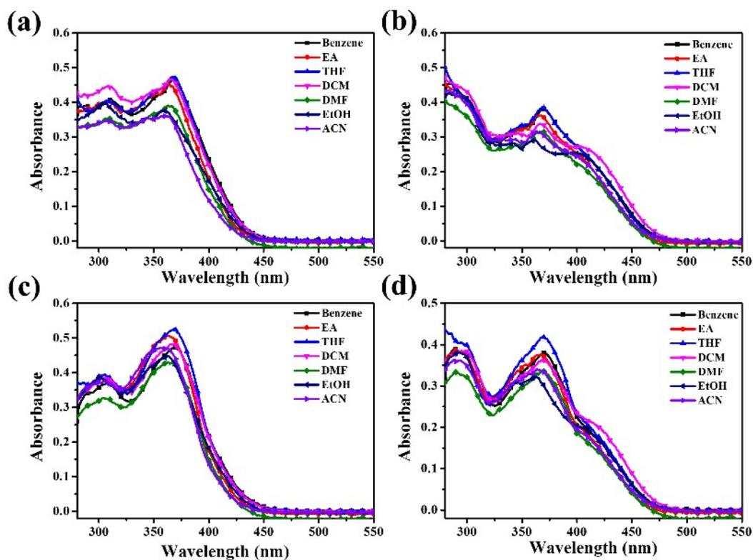
**Fig. S3.** UV-vis spectra of compounds (a) M1, (b) M2, (c) M3, and (d) M4 in different solvents (10  $\mu$ M).
