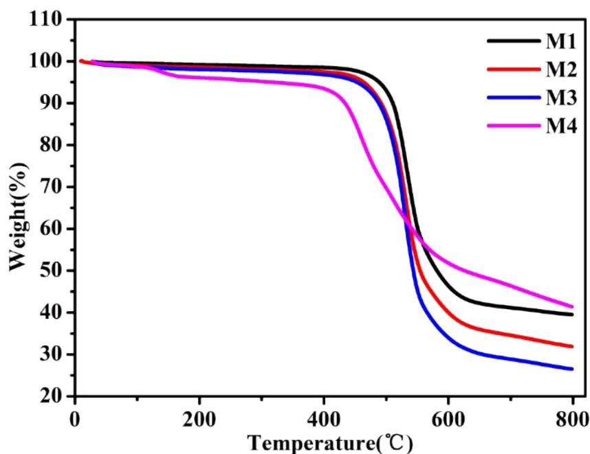
Fig. S1. The TGA curve of compounds **M1**, **M2**, **M3**, and **M4**.
