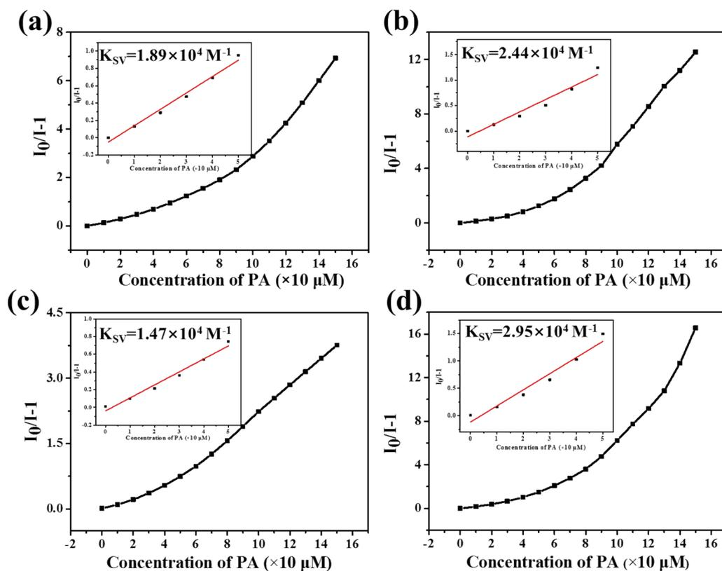
**Fig. S6.** Stern-Volmer plot of (a) **M1**, (b) **M2**, (c) **M3**, and (d) **M4** in response to PA.
