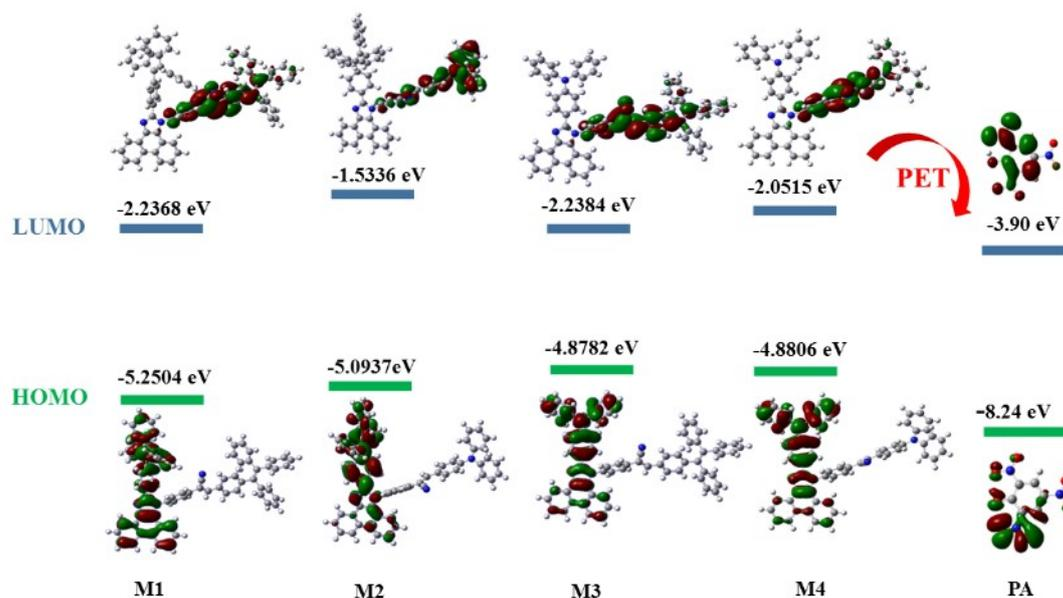
**Fig. S8.** Optimized molecular structures and molecular orbital amplitude plots of the LUMO and HOMO levels, energy gaps and electron cloud distribution of M1, M2, M3, M4, and PA calculated using the B3LYP/6-31G\* basis set.
