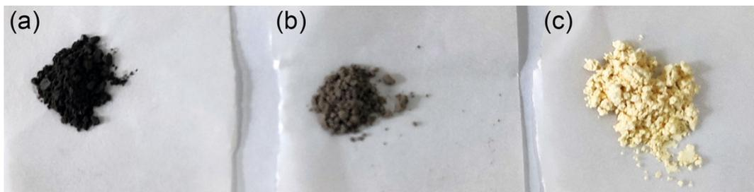
**Fig. S1.** The photographs of (a)  $g\text{-C}_3\text{N}_4\text{-PPy-FeCl}_3$ , (b)  $g\text{-C}_3\text{N}_4\text{-PPy-Fe}_2\text{O}_3$  and (c)  $g\text{-C}_3\text{N}_4$ .
