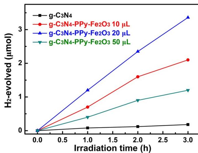
**Fig. S2** The photocatalytic hydrogen production activity of  $g\text{-C}_3\text{N}_4$  and  $g\text{-C}_3\text{N}_4\text{-PPy-Fe}_2\text{O}_3$  with different volume of Py.
