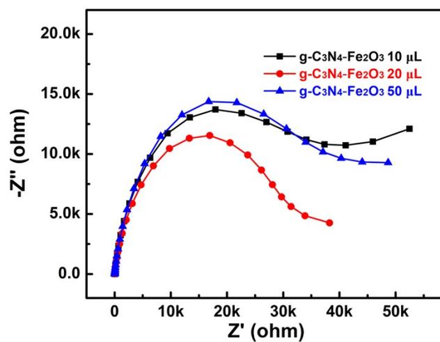
Fig. S4 The electrochemical impedance spectroscopy (EIS) spectra of  $g\text{-C}_3\text{N}_4$  and  $g\text{-C}_3\text{N}_4\text{-PPy-Fe}_2\text{O}_3$  with different volume of Py.
