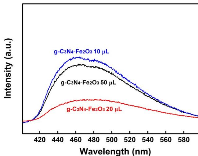
Fig. S3 The PL emission spectra of  $g\text{-C}_3\text{N}_4$  and  $g\text{-C}_3\text{N}_4\text{-PPy-Fe}_2\text{O}_3$  with different volume of Py.
