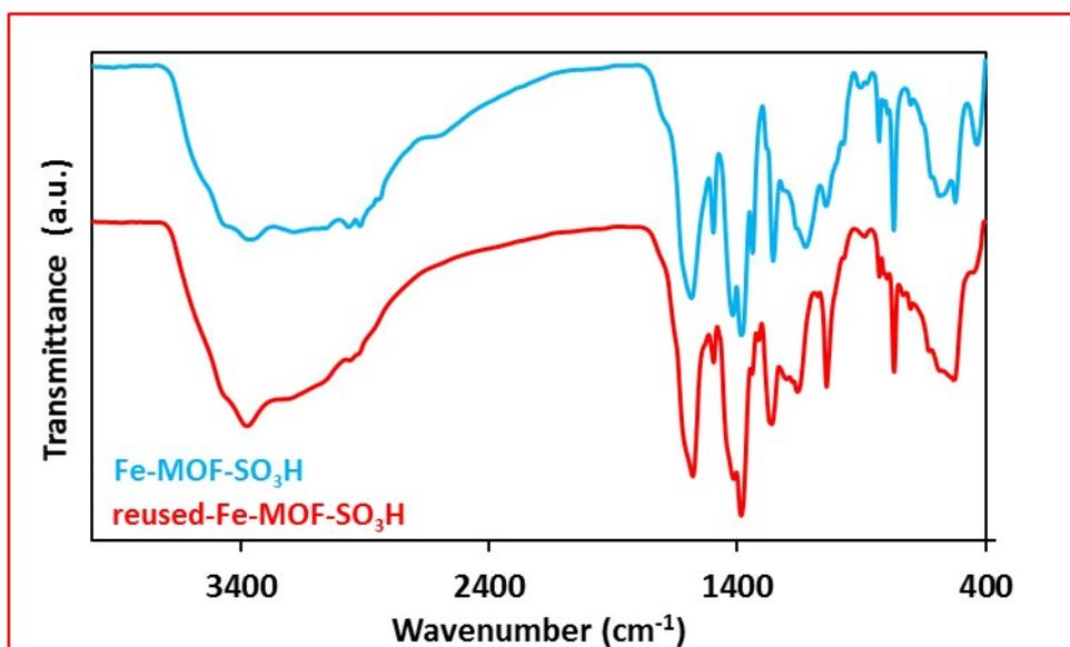
**Figure S7.** FT-IR spectra of fresh and 5<sup>th</sup> recovered Fe-MOF-SO<sub>3</sub>H after catalytic reaction.
