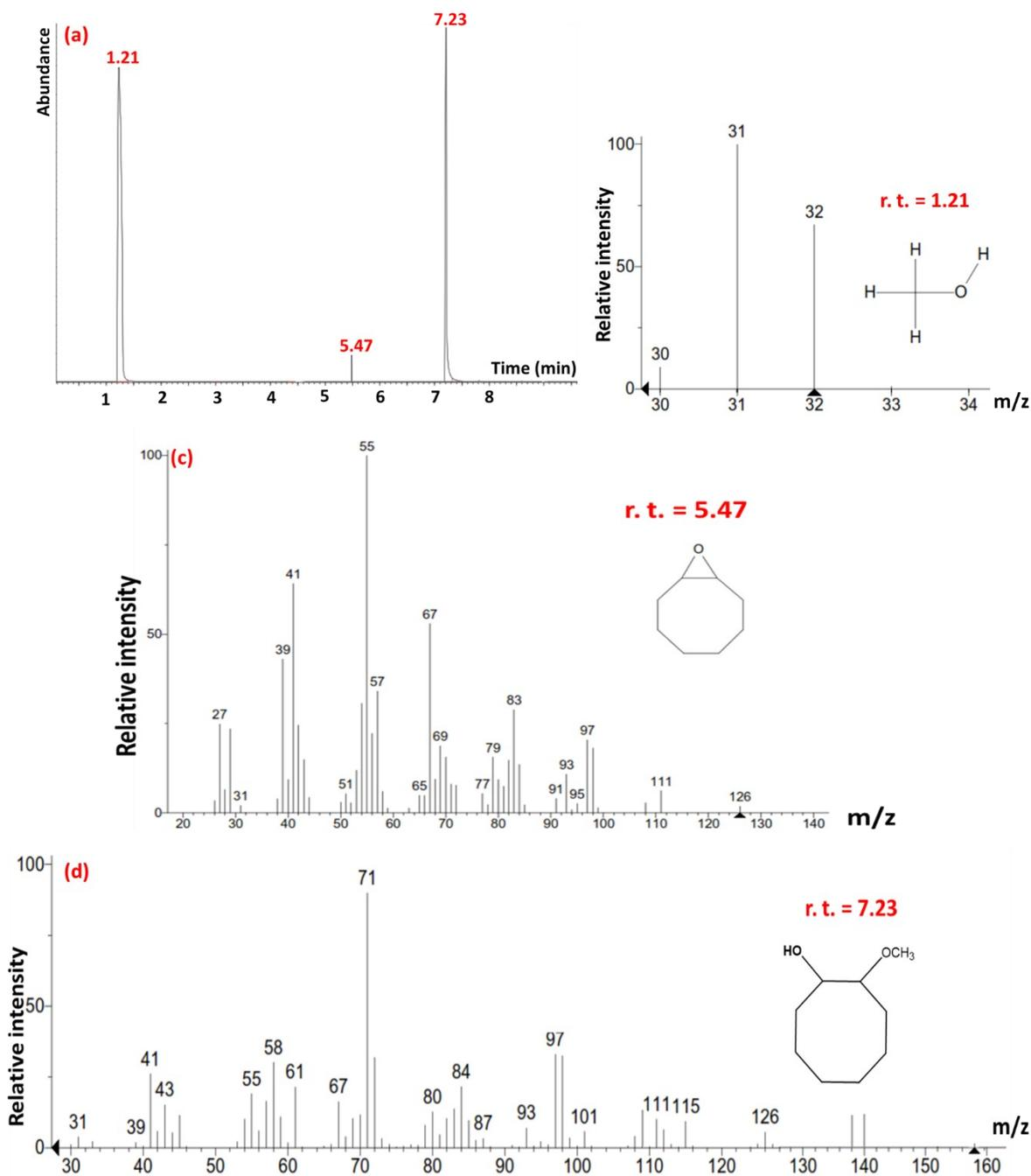
**Figure S3.** (a) GC; (b), (c) and (d) mass spectra of the products of 1,2-epoxy cyclooctane ring-opening reaction after 5 min.
