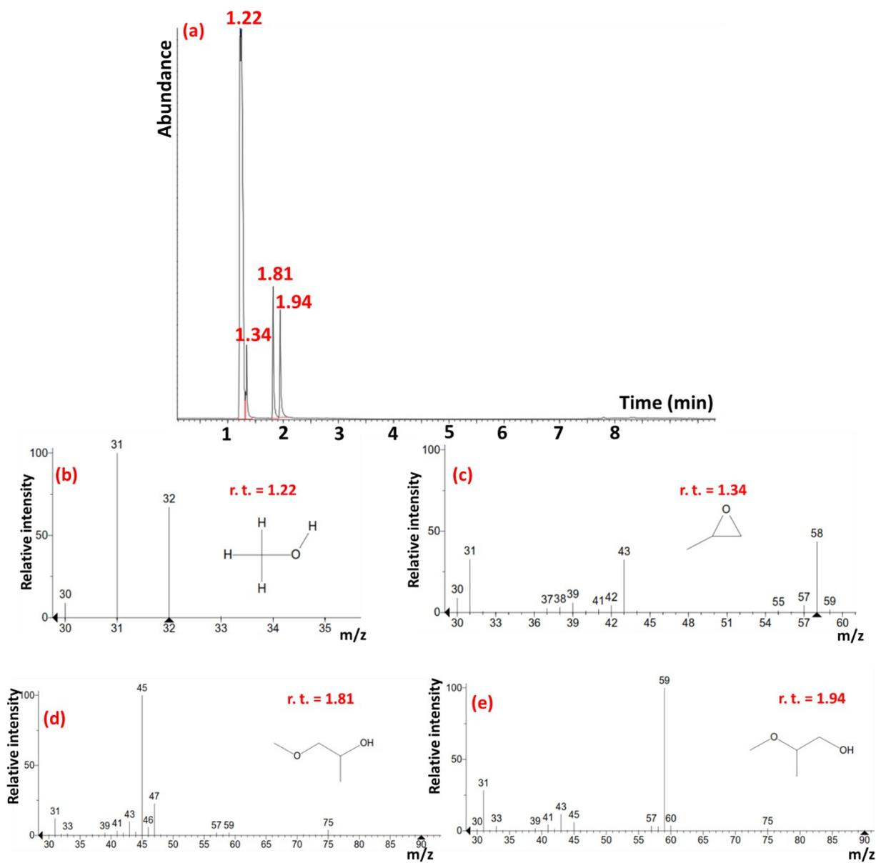
**Figure S4.** (a) GC; (b), (c), (d) and (e) mass spectra of the products of propylene oxide ring-opening reaction after 5 min.
