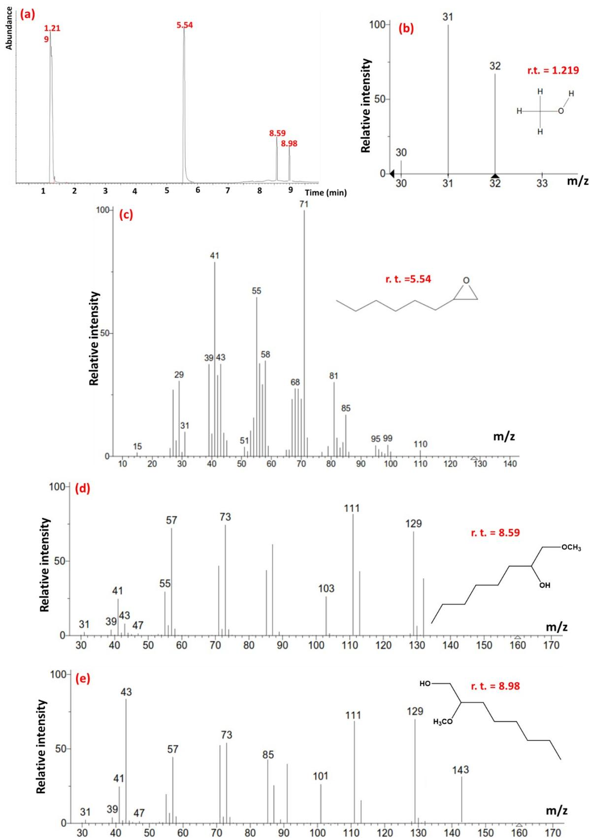
**Figure S6.** (a) GC; (b), (c), (d) and (e) mass spectra of the products of 1,2-epoxyoctane ring-opening reaction after 5 min.
