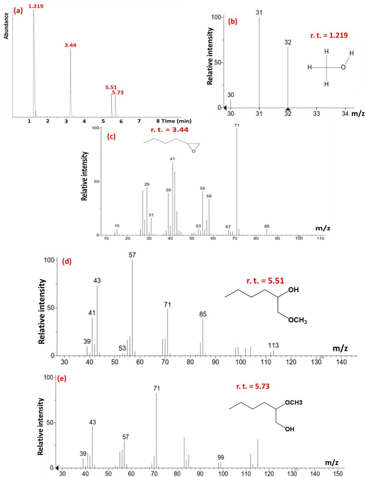
**Figure S5.** (a) GC; (b), (c), (d) and (e) mass spectra of the products of 1,2-epoxyhexane ring-opening reaction after 5 min.
