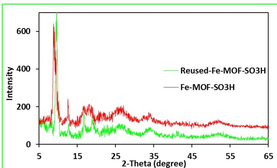
**Figure S8.** XRD patterns of fresh and 5<sup>th</sup> recovered Fe-MOF-SO<sub>3</sub>H.
