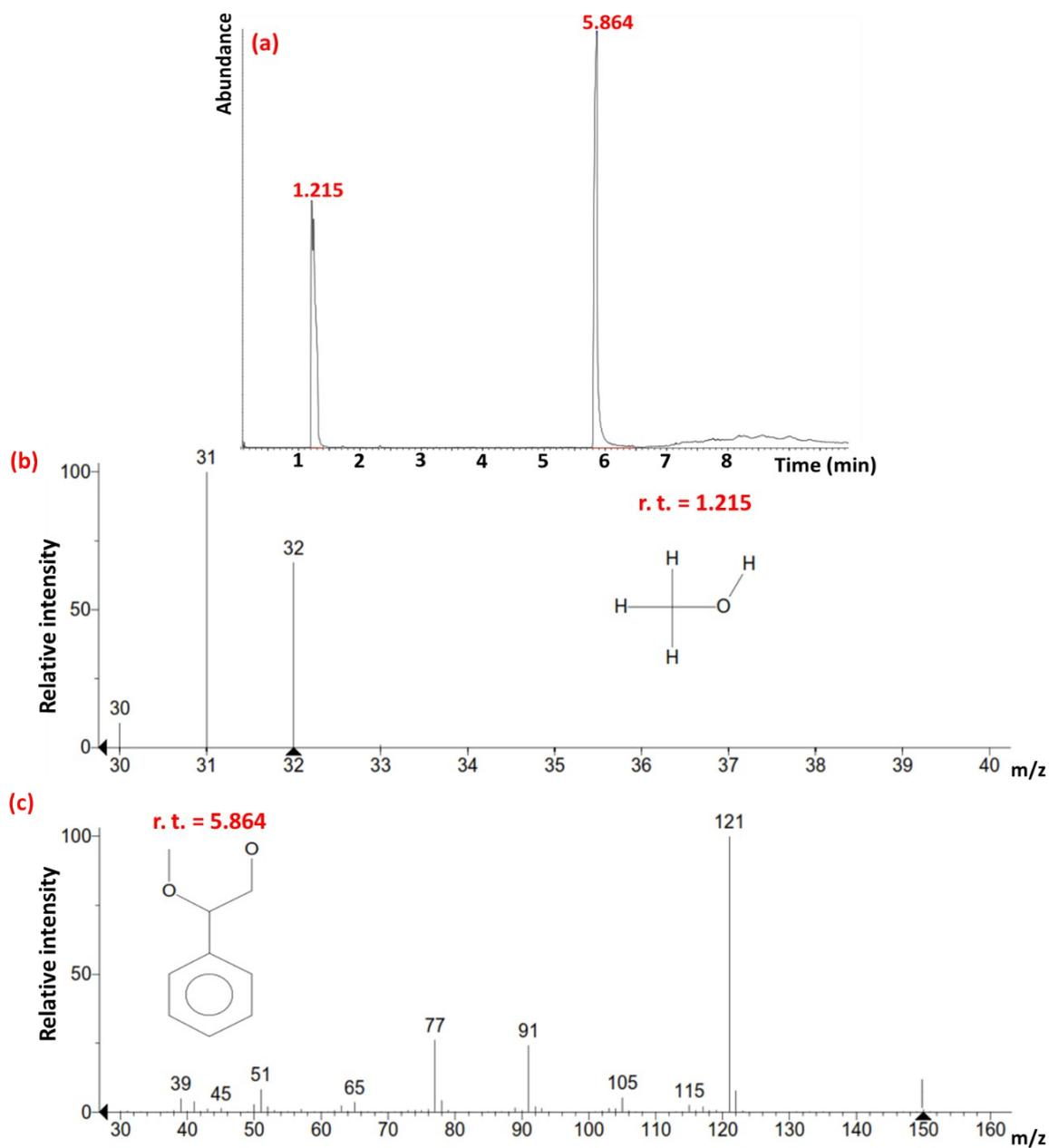
**Figure S1.** (a) GC; (b) and (c) the mass spectra of the products of styrene oxide ring-opening reaction after 3 min.
