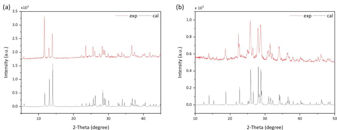
**Figure S1** Powder X-ray diffraction patterns for (a) compound (1) and (b) compound (2) (red line). For comparison, calculated X-ray diffraction patterns (black line) were included.
