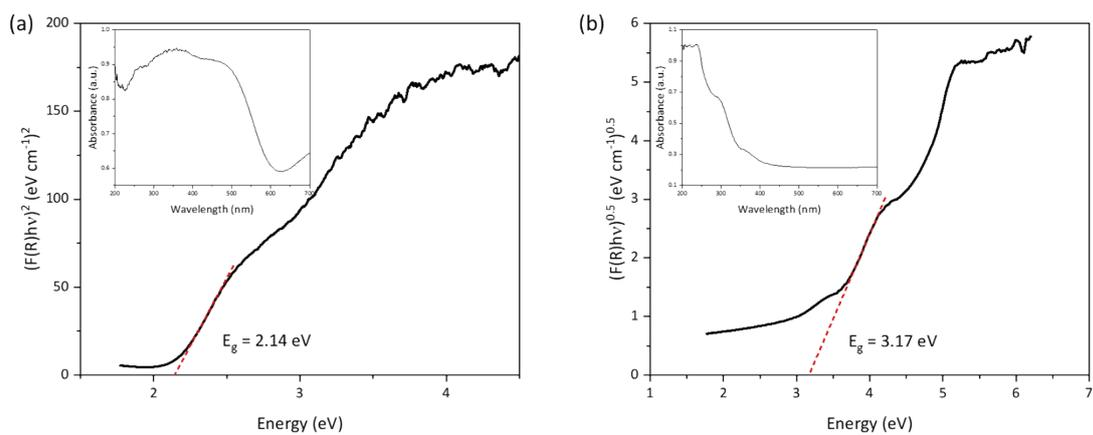
**Figure S3** Kubelka-Munk function for (a) compound (1) and (b) compound (2). The determinations of  $E_g$  are shown as dotted red lines. The inset shows the corresponding measured spectrum.
