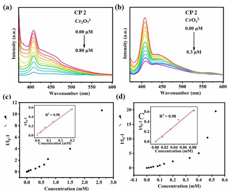
Figure S5. The fluorescence spectra of CP 2 with different concentrations of (a)  $\text{Cr}_2\text{O}_7^{2-}$  and (b)  $\text{CrO}_4^{2-}$  anions; the Ksv plot of CP 2 for sensing of (c)  $\text{Cr}_2\text{O}_7^{2-}$  and (d)  $\text{CrO}_4^{2-}$  anions (insert: S–V plots at low concentrations).
