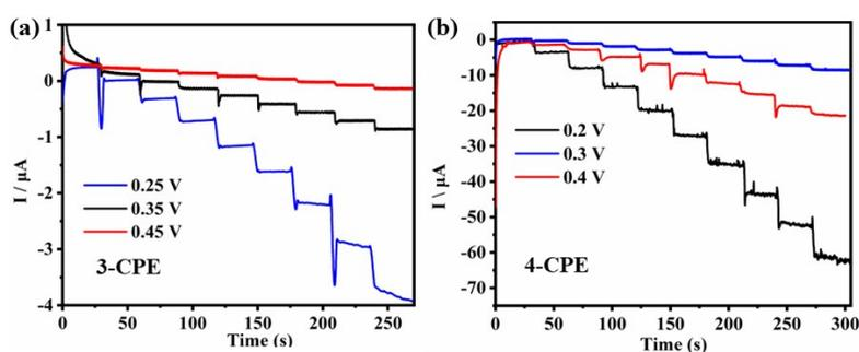
**Figure S12.** Amperometric current responses of CPs **3–4-CPE** upon addition of  $\text{Cr}_2\text{O}_7^{2-}$  ions.
