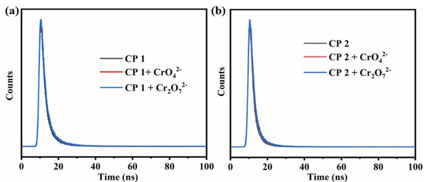
Figure S10. Lifetime decay curves of CPs 1–2 before and after the addition of analytes.
