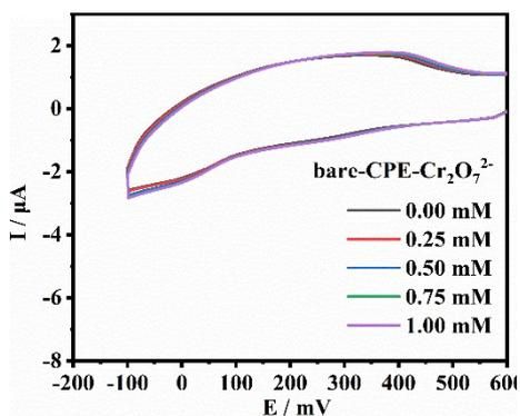
**Figure S11.** The cyclic voltammogram of bare-CPE in a buffer solution containing different concentrations of  $\text{Cr}_2\text{O}_7^{2-}$  ions (Scan rate:  $60 \text{ mV s}^{-1}$ ).
