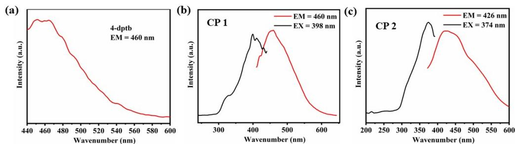
**Figure S3.** Solid-state fluorescence spectra of CPs 1–2 and 4-dptb.
