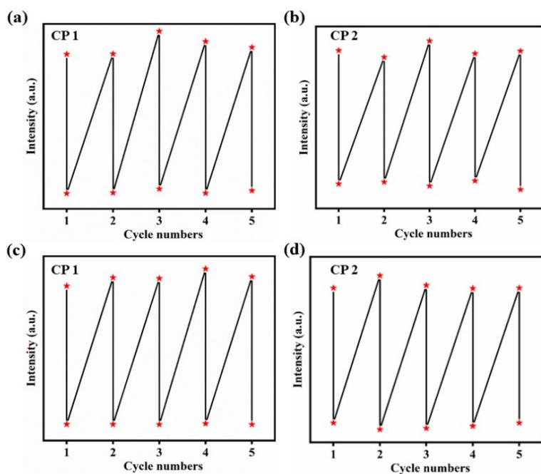
**Figure S7.** Recyclability for sensing (a–b)  $\text{Cr}_2\text{O}_7^{2-}$  and (c–d)  $\text{CrO}_4^{2-}$  anions of CPs 1–2 with five continuously quenching cycles.
