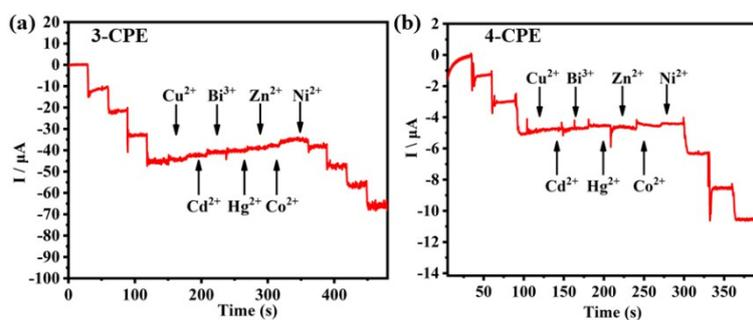
**Figure S13.** Amperometric current responses of CPs **3–4-CPE** in a buffer solution containing  $\text{Cr}_2\text{O}_7^{2-}$  ions with successive additions of  $100 \mu\text{M}$  of various metal ions.
