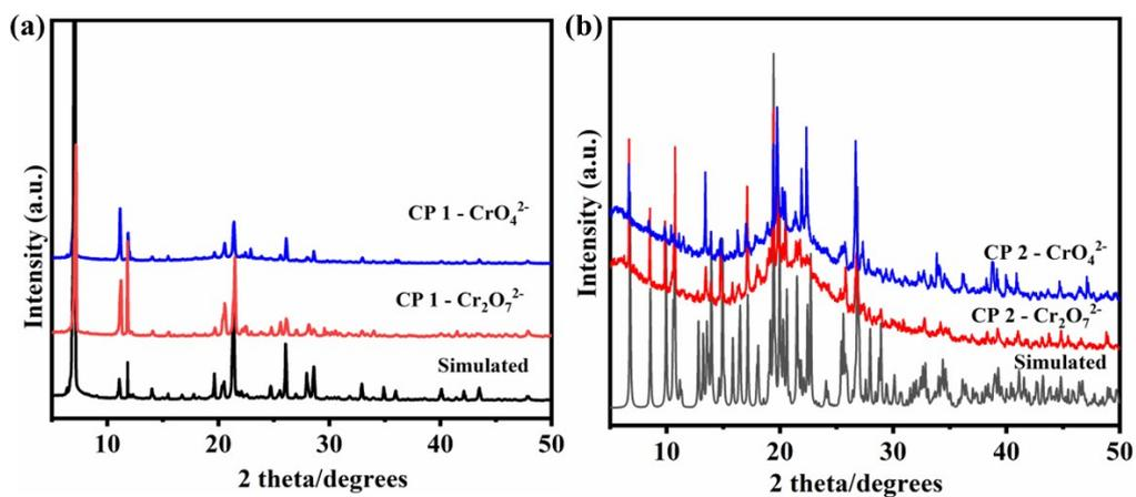
Figure S8. The PXRD patterns of CPs 1–2 before and after exposure to different analytes.
