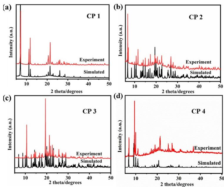
**Figure S2.** The experimental and simulated X-ray powder diffraction of CPs 1–4.
