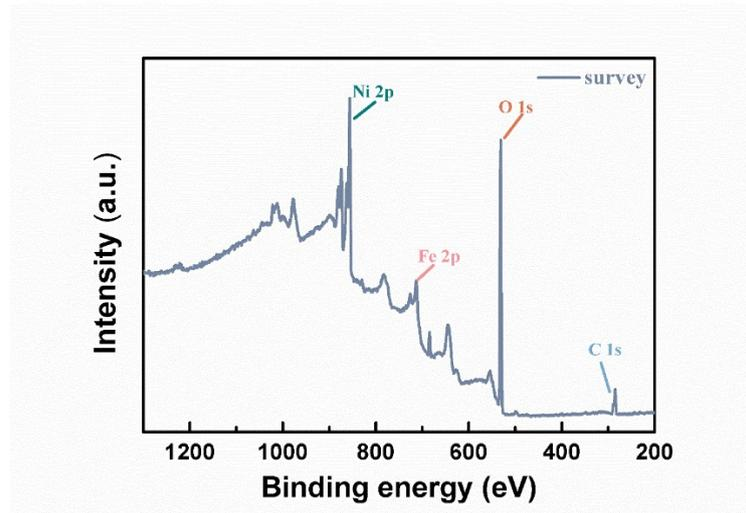
Fig. S7. The survey spectrum of NiFe NCs/GO. The only found of Ni, Fe, C and O elements.
