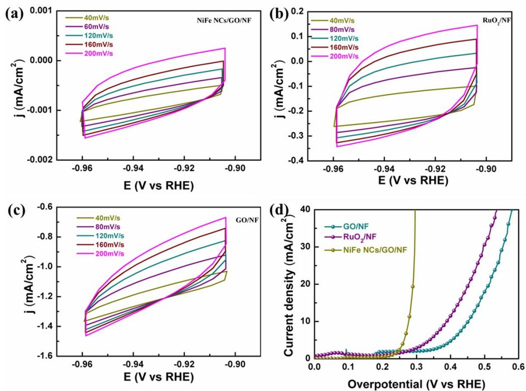
**Fig. S11.** Cyclic voltammograms of (a) NiFe NCs/GO/NF, (b) RuO<sub>2</sub>/NF, (c) GO/NF at different scan rates in 1 M KOH. (d) The LSV polarization curve normalized by the Electrochemical surface area.
