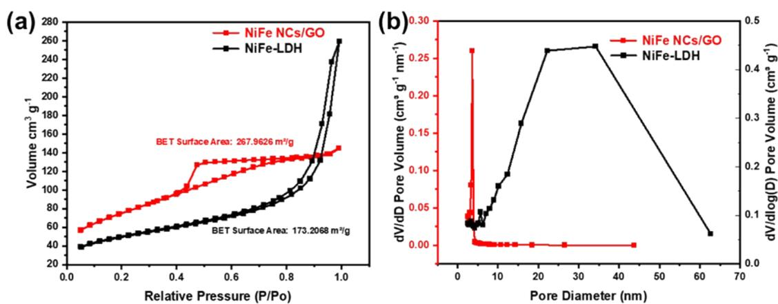
Fig. S5. (a) Nitrogen adsorption–desorption isotherms and (b) Pore sizes distribution
