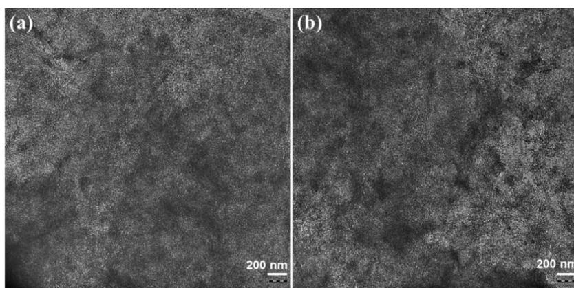
**Fig. S12.** The TEM image of NiFe NCs/GO (a) before and (b) after the 12h i-t test.
