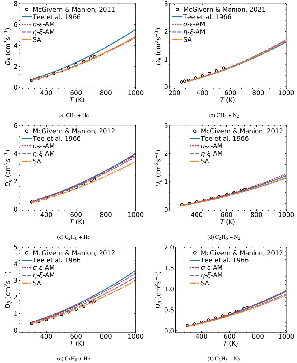
Figure S-1: Comparison of binary diffusion coefficients of  $\text{CH}_4$ ,  $\text{C}_2\text{H}_6$ , and  $\text{C}_3\text{H}_8$  in  $\text{He}$  or  $\text{N}_2$ . Symbols are experimental diffusion data; solid lines are calculated by empirical parameters; dashed lines are calculated by Lennard-Jones parameters obtained via different averaging rules.
