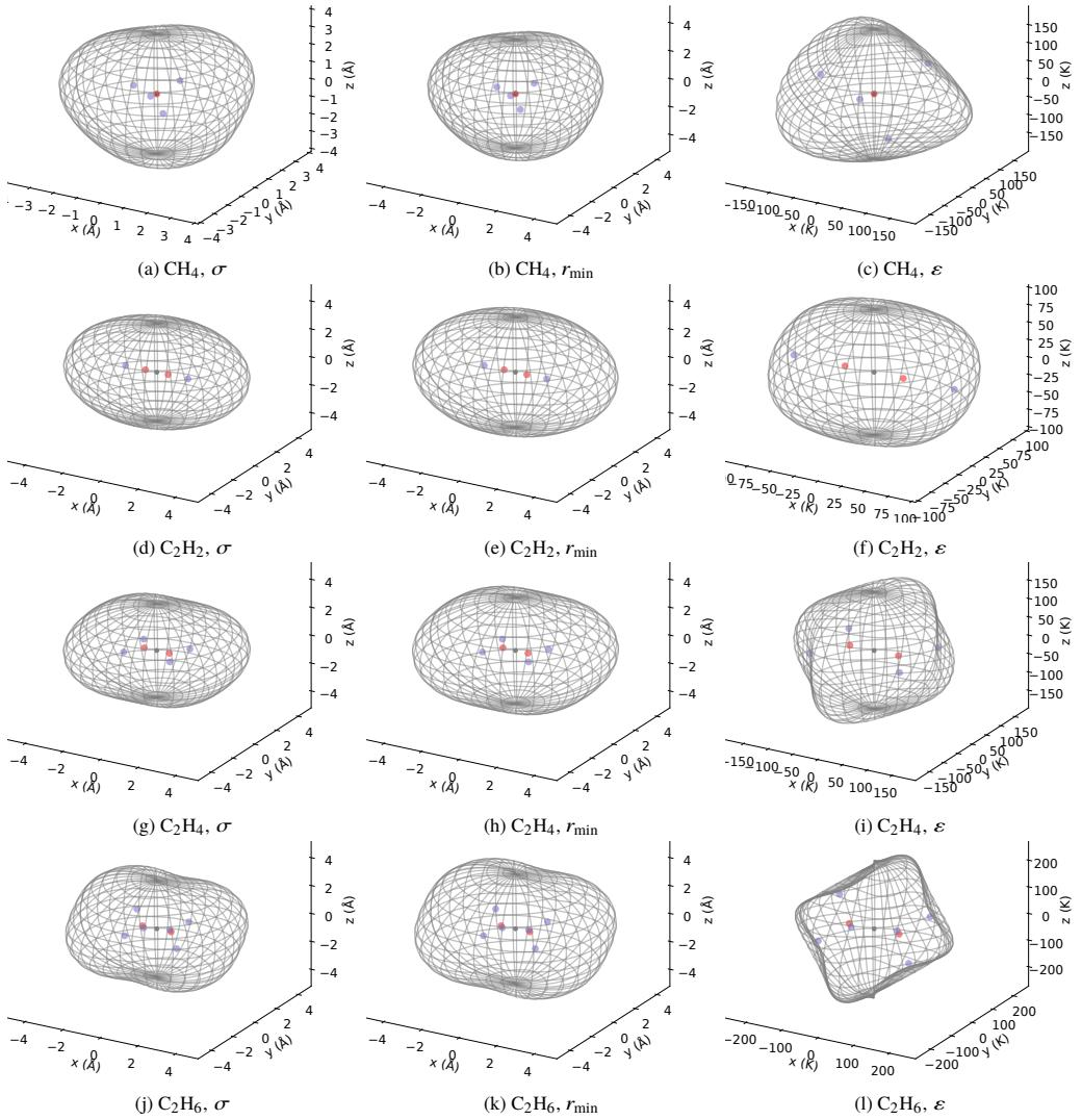
Figure S-4: Three-dimensional parametric surfaces of the collision diameter  $\sigma$ , well location  $r_{\min}$ , and well depth  $\varepsilon$  by the developed iterative search method for a set of target-Ar pairs.
