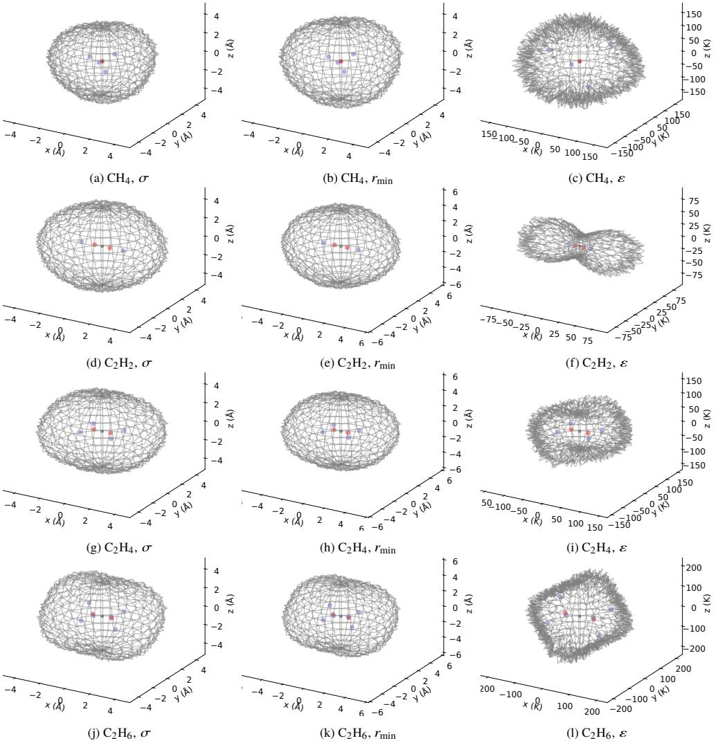
Figure S-5: Three-dimensional parametric surfaces of the collision diameter  $\sigma$ , well location  $r_{\min}$ , and well depth  $\varepsilon$  by the developed iterative search method for a set of target-N<sub>2</sub> pairs. The non-smoothness of related surfaces is due to the self-rotation of the diatomic bath gase during ensemble generation.
