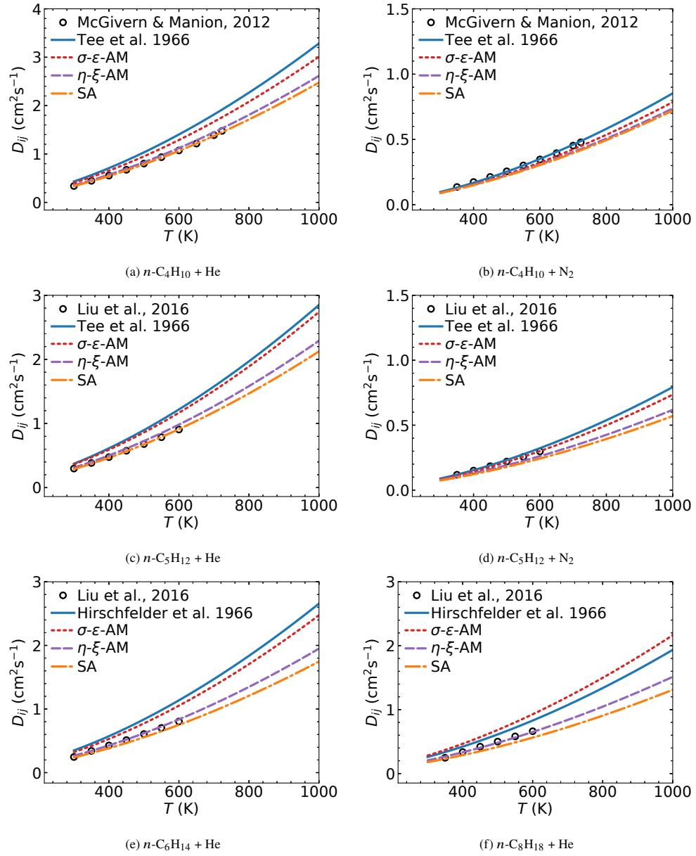
Figure S-2: Comparison of binary diffusion coefficients of  $n\text{-C}_4\text{H}_{10}$ ,  $n\text{-C}_5\text{H}_{12}$ ,  $n\text{-C}_6\text{H}_{14}$ , and  $n\text{-C}_8\text{H}_{18}$  in He or  $\text{N}_2$ .
