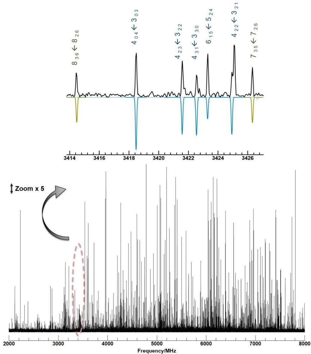
**Figure S8.** Microwave spectrum of the phenyl alcohol dimer in the region 2-8 GHz, following subtraction of the rotational transitions of the monomer. The upper trace expansion illustrates typical transitions from the heterochiral ( $G'G'-GG'-Lp+$ , purple) and homochiral ( $G'G'-G'G'-Lp+$ , orange) isomers.
