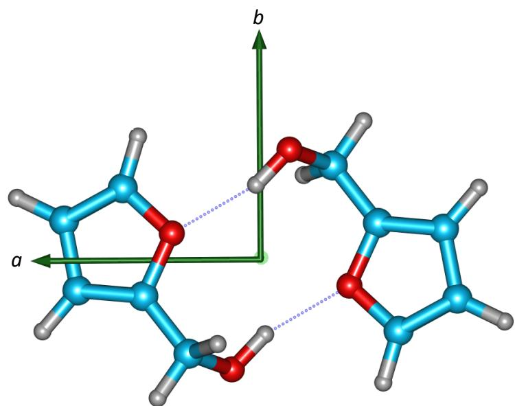
**Figure S5.** An illustration of thenyl alcohol dimers with a parallel-displaced near-staked orientation of the two thenyl rings. For these isomers some of the monomers may adopt anticalinal orientations of the sidechain. The smaller electronic energies for these configurations are 1.5-3.7 kJ mol<sup>-1</sup> (B3LYP-D3(BJ)). Other stacked conformations may be possible.
