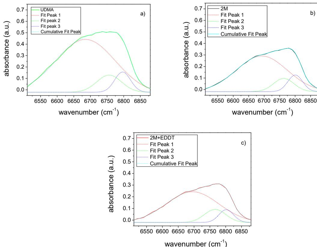
**Fig. S2** Gaussian peak decomposition of the N-H absorption band for uncured a) UDMA, b) 2M and c) 2M+EDDT samples.
