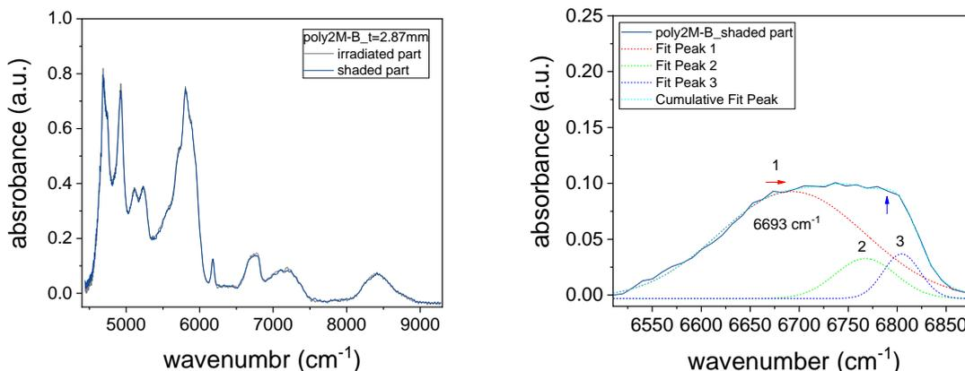
**Fig. S4** NIR spectra for cured poly2M-B sample via mask (left), measured in the irradiated middle and shaded part of disc, with Gaussian peak decomposition of the N-H absorption band for the shaded part (right).
