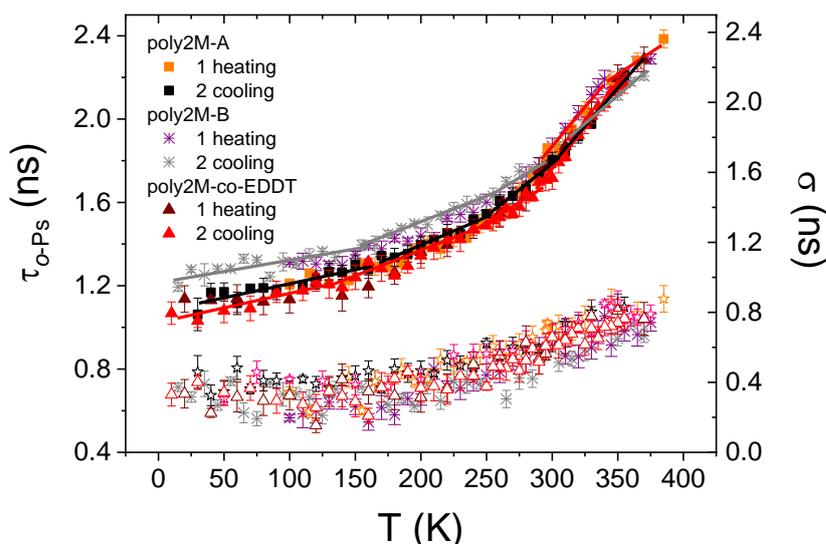
**Fig. S5** Temperature dependences of the *o*-Ps lifetimes (full symbols) and the lifetime dispersions (empty symbols) for poly2M-A, poly2M-B samples and poly2M-co-EDDT. The lines show the trend of  $\tau_{o-Ps}$  and  $\sigma$  for the cooling cycle.
