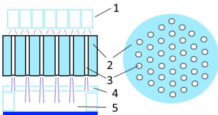
**Fig. S1** A scheme of the irradiated sample through the mask. 1–LED light source, 2–Al block as a shield, 3–lightguides (diameter 1.1 mm, length 9 mm), 4–quartz window, 5–sample in a chamber.
