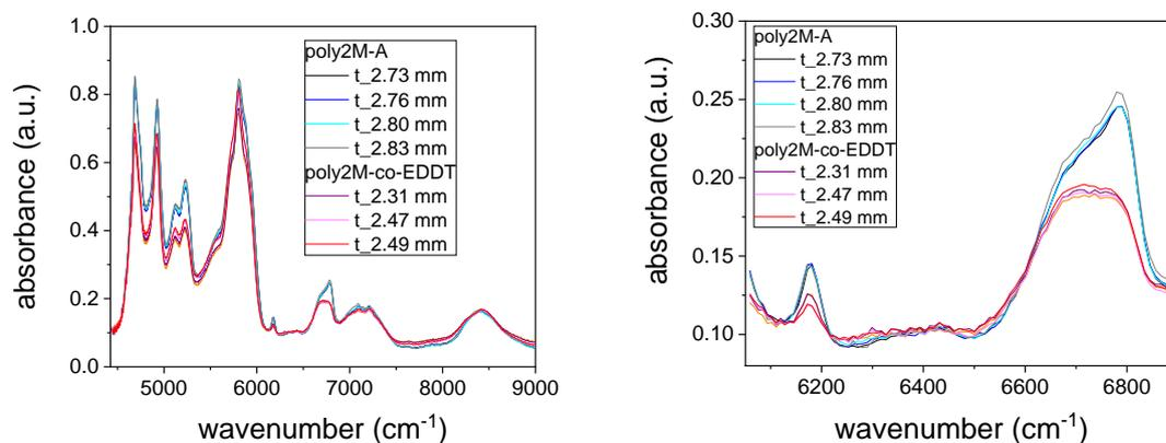
**Fig. S3** NIR spectra for cured poly2M-A and poly2M-co-EDDT samples (left), measured in the middle part of discs, with detailed region of  $>C=CH_2$  and N-H absorption peaks (right).
