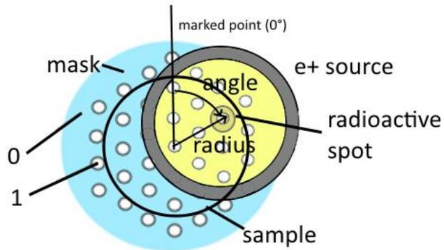
**Fig. S6** The scheme of PALS measurement for directly illuminated and shielded places of cured poly2M-B sample using radioactive positron source for mapping. The measured positions on the mask. 0 – shaded area, 1 – directly illuminated area,  $e^+$  source -  $^{22}\text{NaCl}$  salt between two Kapton foils with radioactive spot in the middle of the disc.
