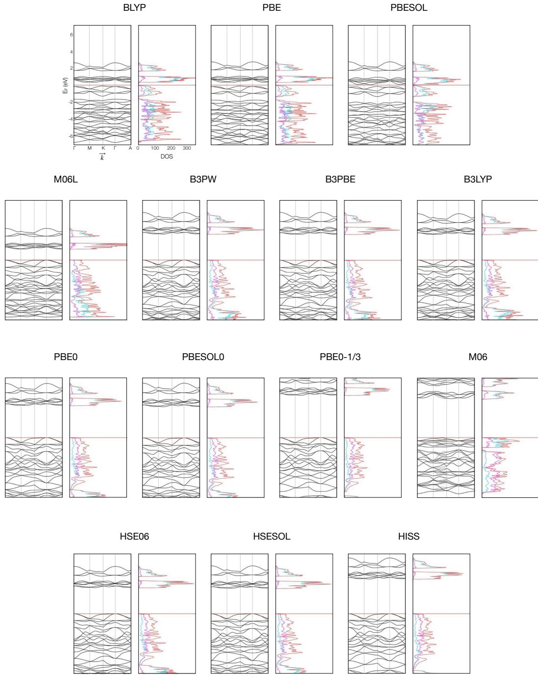
Figure S18: Band structure and density of states for  $\text{Fe}_2\text{O}_3$  calculated with different density functionals. Color-code DOS projections: *red* = total, *light blue* = iron, *pink* = oxygen.
