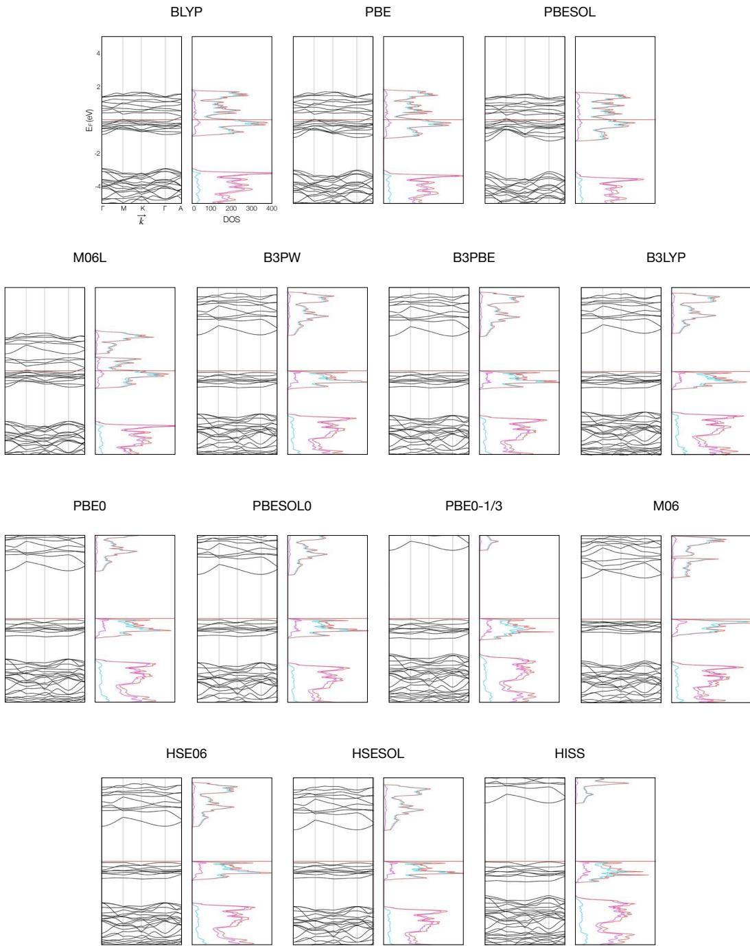
Figure S22: Band structure and density of states for  $\text{V}_2\text{O}_3$  calculated with different density functionals. Color-code DOS projections: *red* = total, *light blue* = vanadium, *pink* = oxygen.
