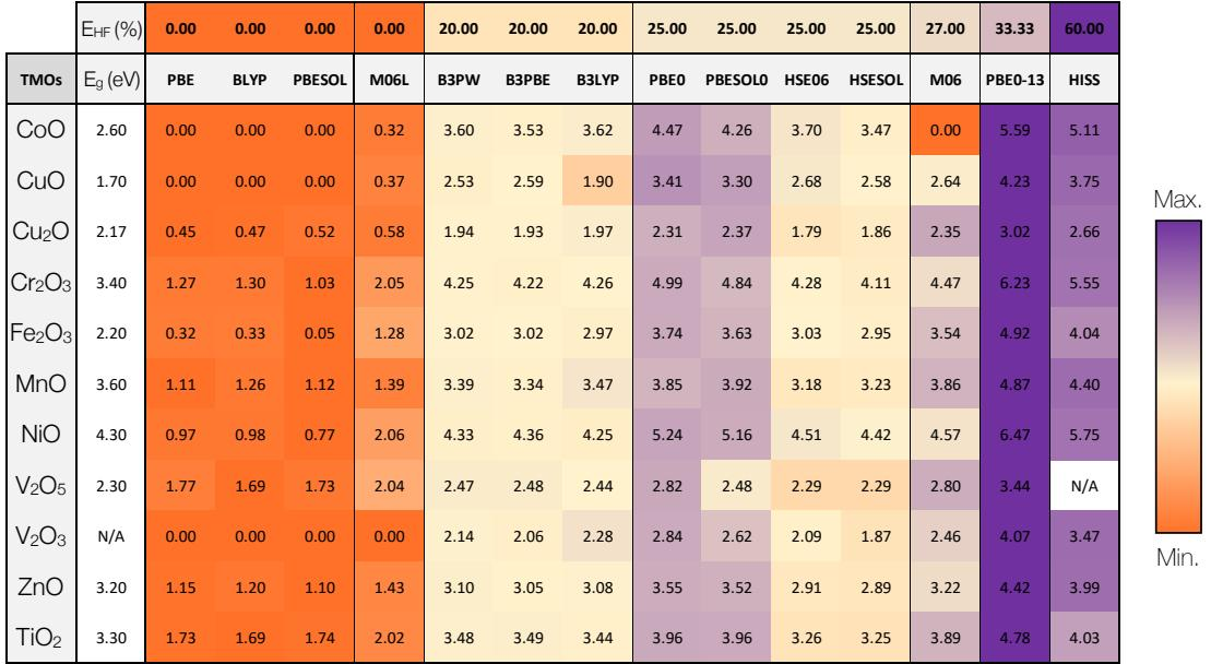
Figure S10: Band gap ( $E_g$ ) values calculated with different density functionals. Experimental data (first column) references: CoO,<sup>48–50</sup> CuO,<sup>51,52</sup> Cu<sub>2</sub>O,<sup>53</sup> Cr<sub>2</sub>O<sub>3</sub>,<sup>54,55</sup> Fe<sub>2</sub>O<sub>3</sub>,<sup>56</sup> MnO,<sup>48,49,57</sup> NiO,<sup>48,58</sup> V<sub>2</sub>O<sub>5</sub>,<sup>59,60</sup> ZnO,<sup>61</sup> TiO<sub>2</sub>.<sup>59</sup>
