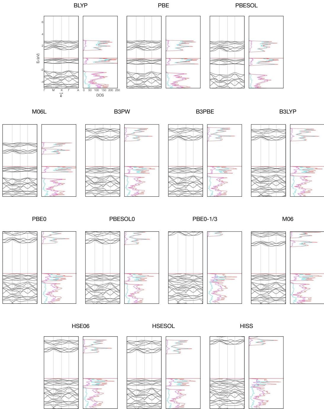
Figure S15: Band structure and density of states for  $\text{Cr}_2\text{O}_3$  calculated with different density functionals. Color-code DOS projections: *red* = total, *light blue* = chromium, *pink* = oxygen.
