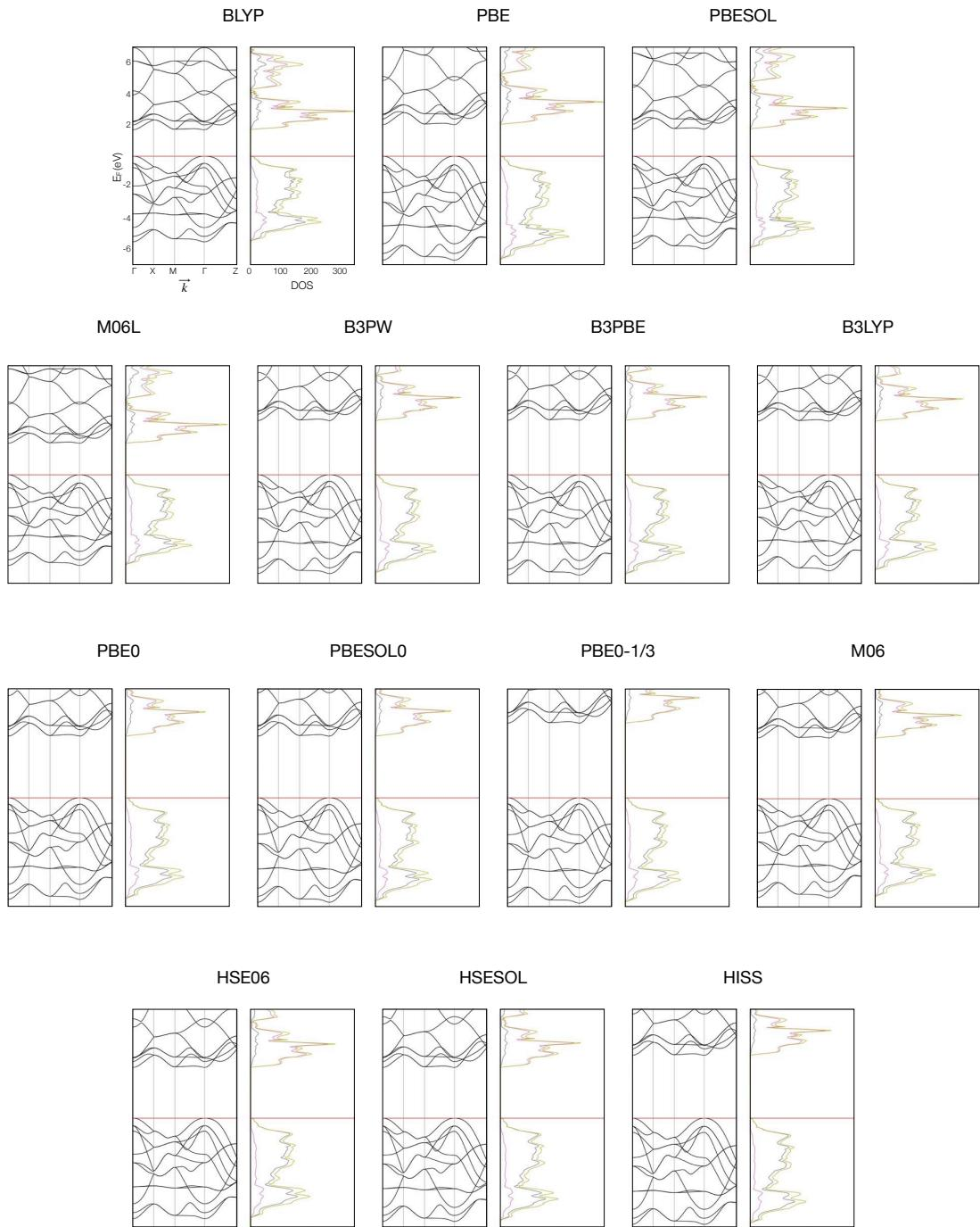
Figure S21: Band structure and density of states for TiO<sub>2</sub> calculated with different density functionals. Color-code DOS projections: *light green* = total, *pale pink* = titanium, *grey* = oxygen.
