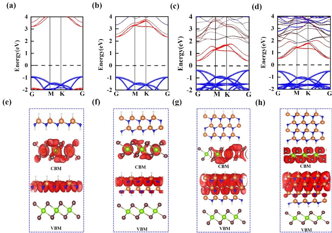
**Figure S7.** Projected band structure of N-GaN/MgI<sub>2</sub> heterostructures with the different GaN layers in (a) 1L, (b) 2L, (c) 3L, and (d) 4L. MgI<sub>2</sub> and GaN contributions to the heterostructures are represented by the red and blue balls, separately. The dashed lines indicate the Fermi level. CBM and VBM charge-density isosurfaces in 2D MgI<sub>2</sub>/N-GaN heterostructures with GaN layer thickness in (e) 1L, (f) 2L, (g) 3L, and (h) 4L.
