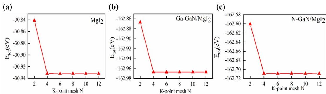
**Figure S1.** Total energies ( $E_{tot}$ ) of (a) pristine  $MgI_2$  monolayer, (b)  $MgI_2$ /Ga-GaN heterostructure, and (c)  $MgI_2$ /N-GaN heterostructure with different k-point mesh  $N$  (i.e.,  $N \times N \times 1$ ).
