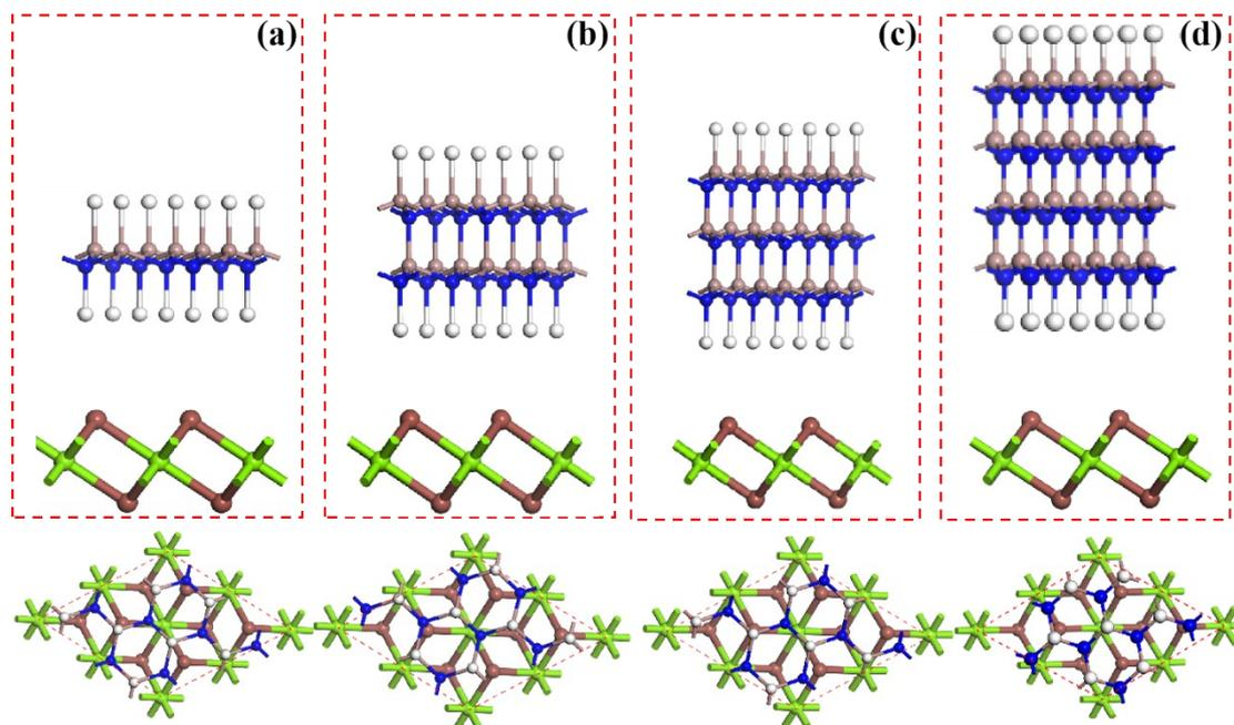
**Figure S4.** the different stacking patten of MgI<sub>2</sub>/N-GaN heterostructures with the thickness of GaN layer in (a) monolayer, (b) bilayer, (c) trilayer and(d) tetralayer.
