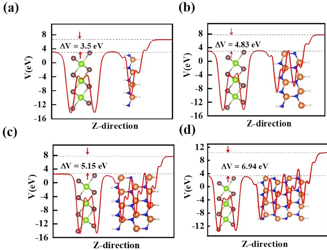
**Figure S6.** Electrostatic potential distribution ( $V$ ) of  $\text{MgI}_2/\text{N-GaN}$  heterostructures with the thickness of GaN layer in (a) monolayer, (b) bilayer, (c) trilayer and (d) tetralayer.  $\Delta V$  is the electrostatic potential difference between two terminations of the heterostructure.
