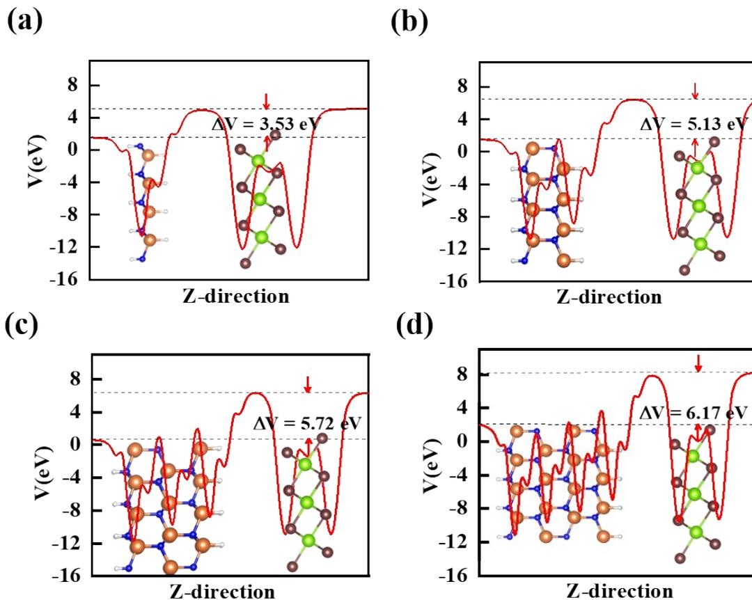
**Figure S5.** Electrostatic potential distribution ( $V$ ) of MgI<sub>2</sub>/Ga-GaN heterostructures with the thickness of GaN layer in (a) monolayer, (b) bilayer, (c) trilayer and (d) tetralayer.  $\Delta V$  is the electrostatic potential difference between two terminations of the heterostructures.
