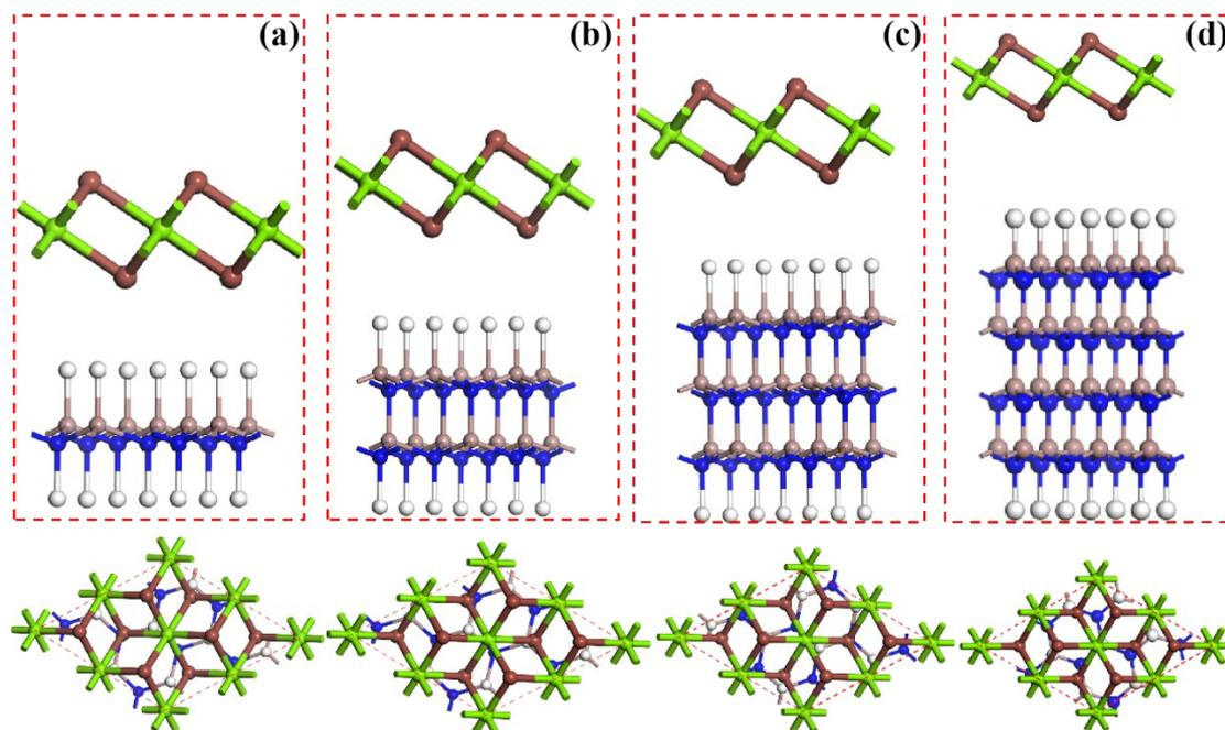
**Figure S3.** The different stacking patten of MgI<sub>2</sub>/Ga-GaN heterostructures with the thickness of GaN layer in (a) monolayer, (b) bilayer, (c) trilayer and(d) tetralayer.
