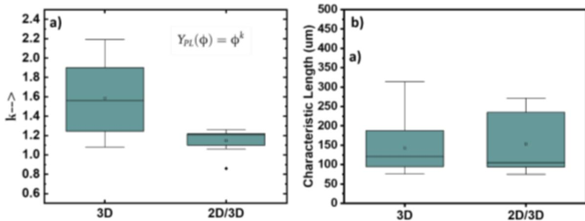
**Fig. S5** Excitation intensity dependent PL intensity measurement. PL intensity was found to obey power law, with  $k$  closer to 2 in 3D sample whereas  $k$  closer to 1 in 2D terminated samples, (b) Position dependent PL intensity variation in 3D and 2D terminated samples shows that the charge carrier diffusion is almost left untouched due to presence of 2D terminated perovskite.
