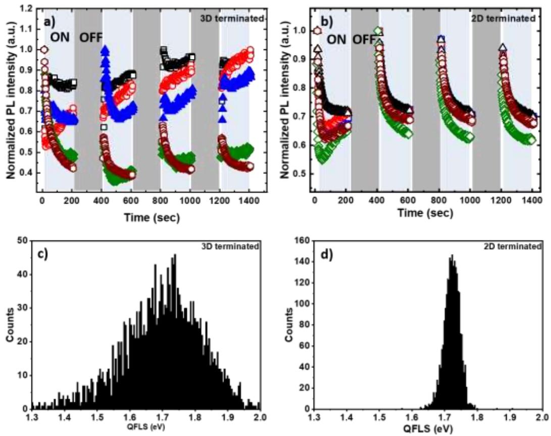
**Fig. S6** Light soaking experiment performed with 405 nm (50 mW) LASER in 75% humidity.
