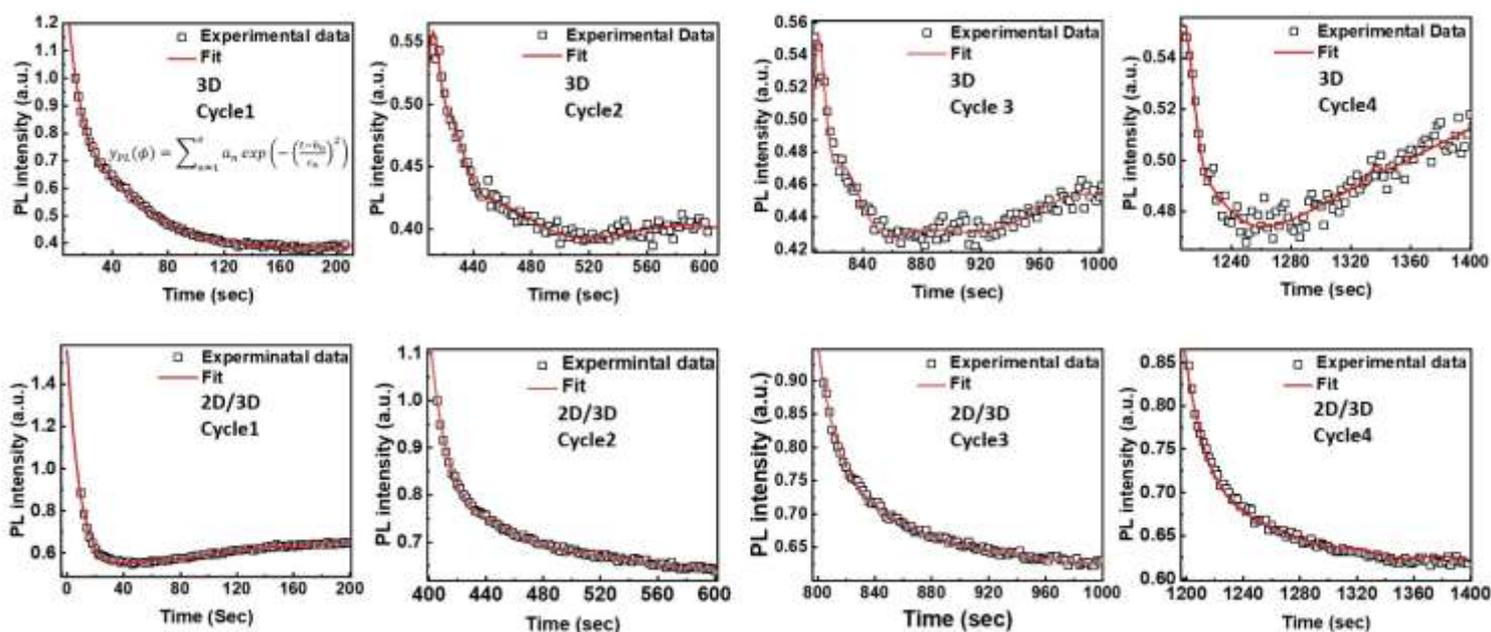
**Fig. S8** Fitting of PL intensity traces under light soaking experiment. PL intensity was measured in 4 cycles for both controlled and 2D/3D samples and fitted with a sum of 4 gaussian function. Fitting parameters can be found in table S1.
