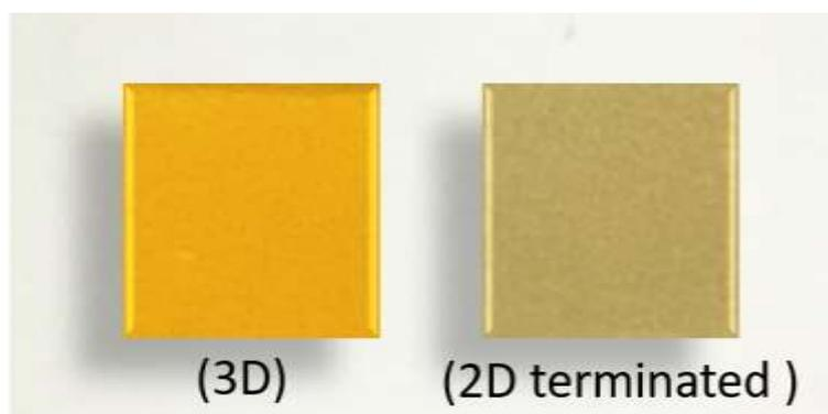
**Fig. S1** Photographic image of controlled 3D and post treated 2D terminated perovskite film. Both films show visual difference in colour due to their different spectral absorbance.
