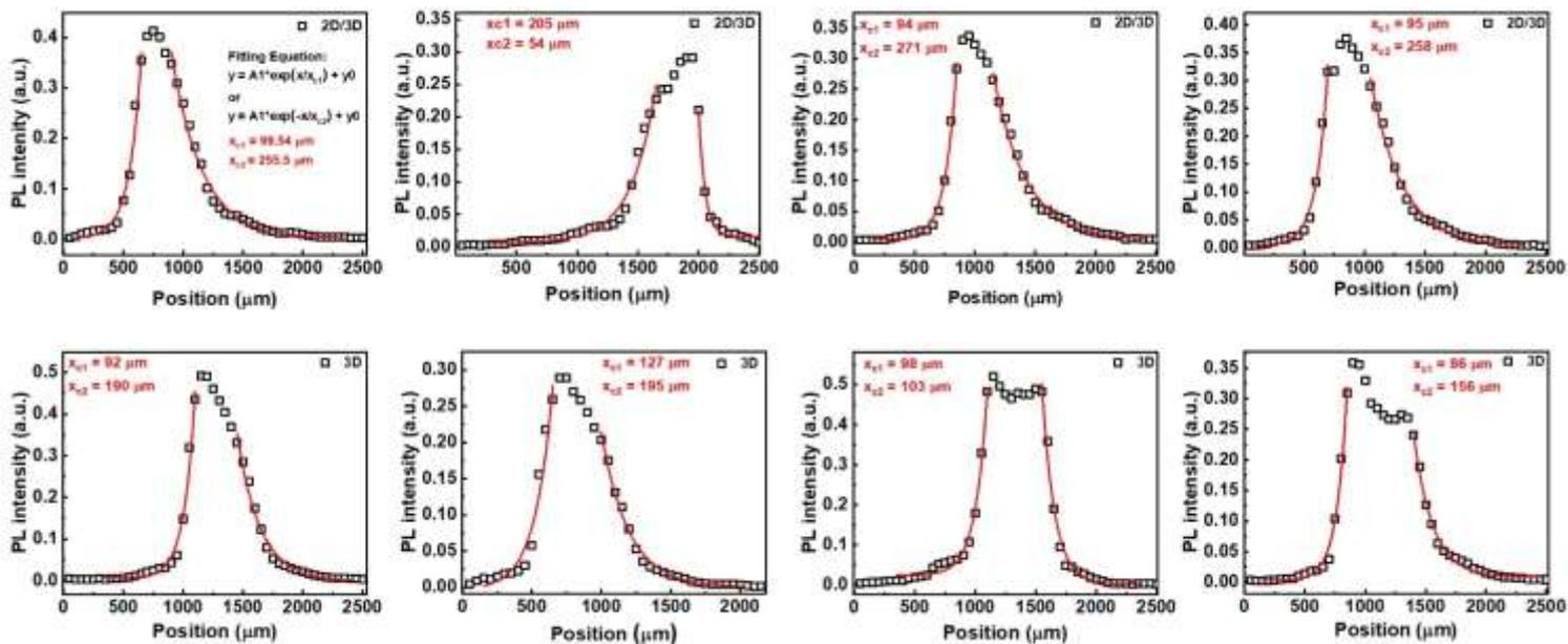
**Fig. S9** Fitting of position dependent PL intensity data.  $X_{C1/2}$  represent the characteristic distance over which intensity drops by a factor of  $1/e$ .
