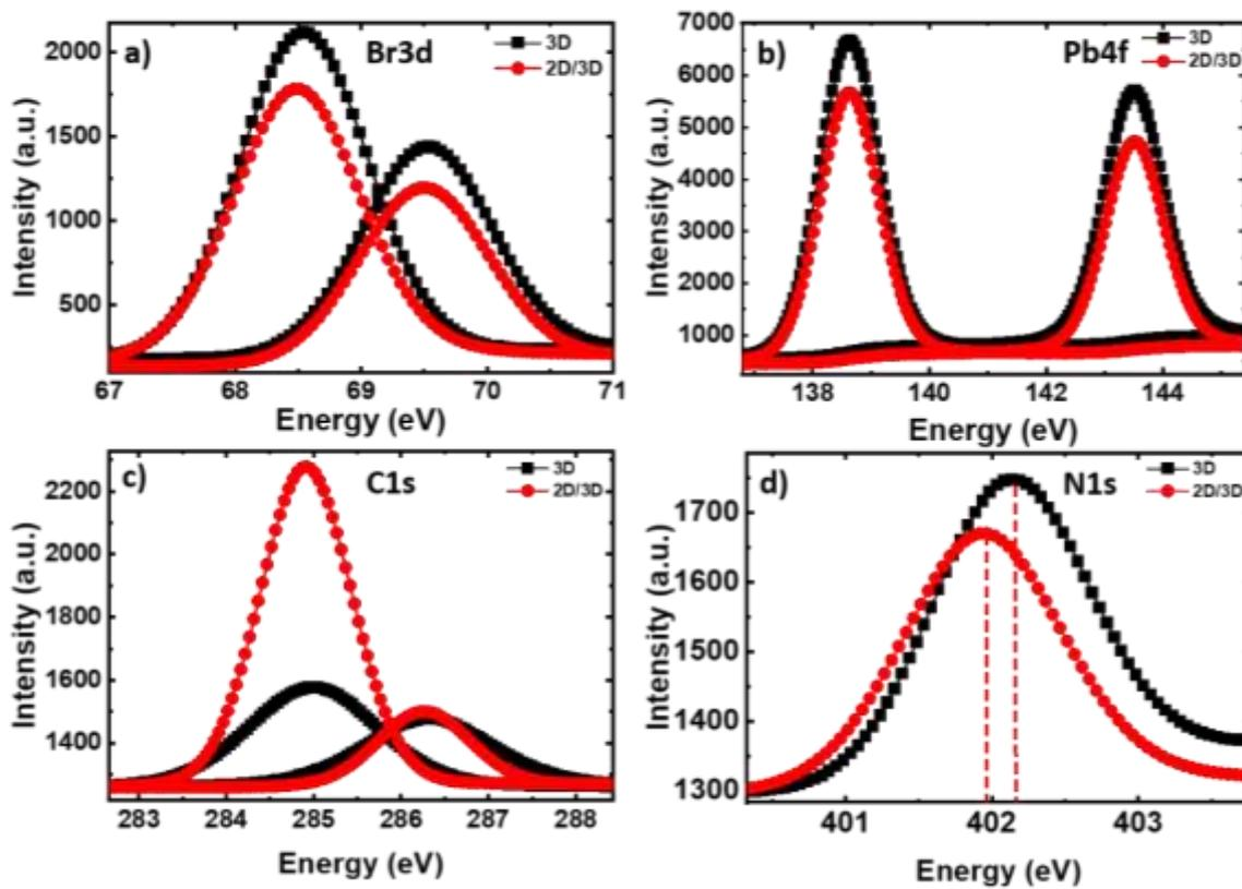
**Fig. S4** XPS spectra of controlled 3D and converted 2D/3D perovskite film. C1s1/2 peak show significant rise in intensity, also N1s peak shows a slight blue shift of ~ 170 meV.
