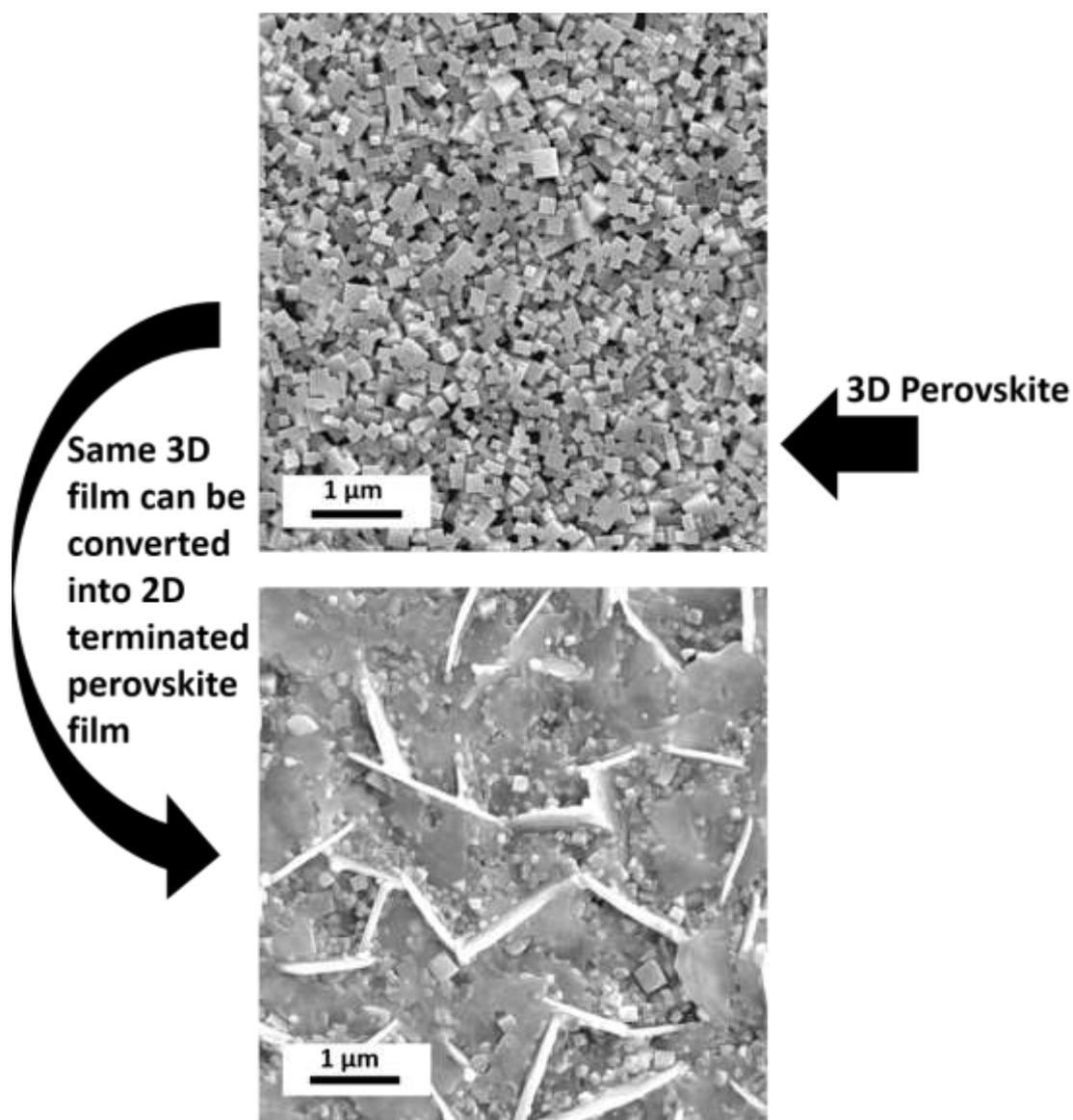
**Fig. S3** FESEM image of (a) controlled 3D and (b) partially redissolved 2D terminated perovskite film redissolved with a 2V% solution of benzylamine in IPA. Treated sample presents a typical morphology of a 2D perovskite sample.
