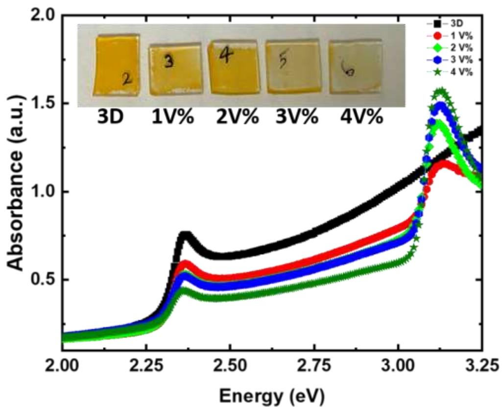
**Fig. S2** Absorption spectrum of controlled and post treated films, post treated films are partially redissolved by 1-4 V% solution of Benzylamine in IPA.
