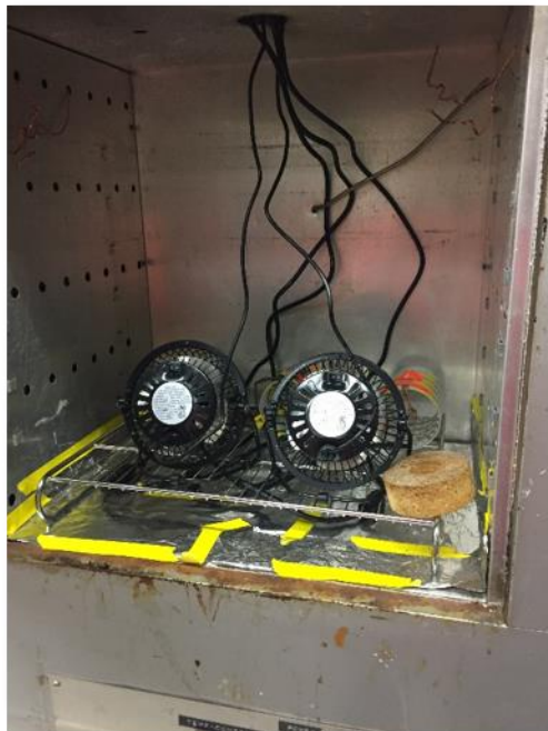
Figure S23. Photoreactor used in maximum radical concentration studies. A) View of set-up showing two fans facing the three cylindrical photoreactors. B) View of one cylindrical photoreactor comprised of a wash bottle that was cut open at both ends with a Waveform Lighting real UV LED strip wrapped along the interior of the cylinder.
