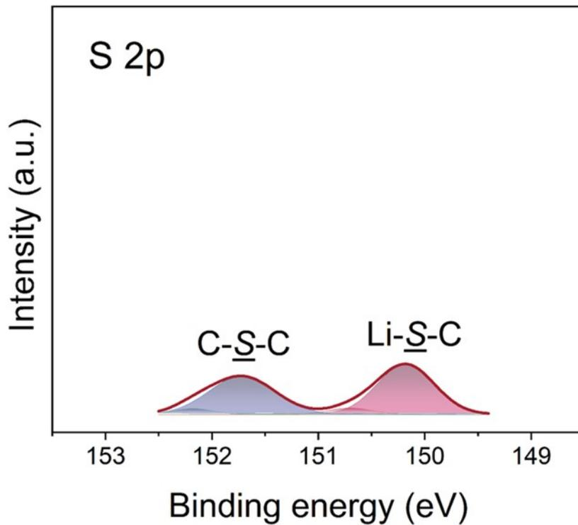
**Figure 2.** X-ray photoelectron spectroscopy (XPS) of S 2p of FSI-TFEO-DME
