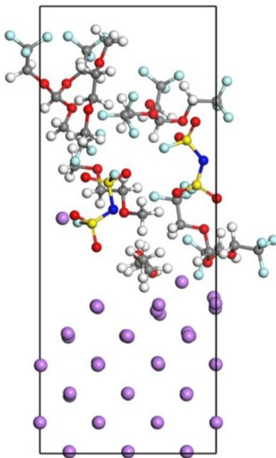
**Figure 1.** Initial model. Color: lithium, purple; oxygen, red; fluorine, cyan; carbon, gray; nitrogen, blue; sulfur, yellow, hydrogen, white.
