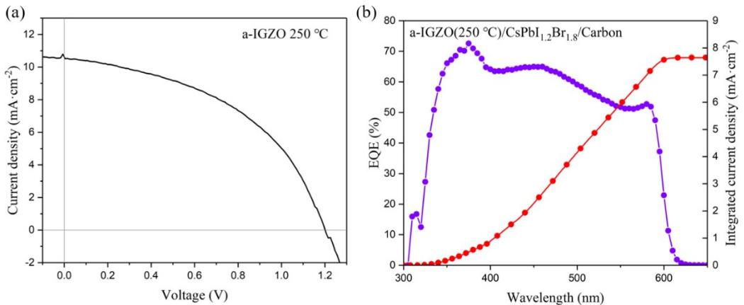
Figure S4. J-V curve (a) and EQE spectra and the corresponding integrated current densities (b) of the device with structure of ITO/a-IGZO (250 °C)/CsPbI<sub>1.2</sub>Br<sub>1.8</sub>/Carbon
