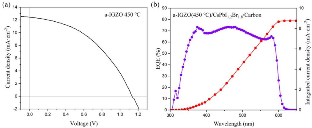
Figure S3. J-V curve (a) and EQE spectra and the corresponding integrated current densities (b) of the device with structure of ITO/a-IGZO (450 °C)/CsPbI<sub>1.2</sub>Br<sub>1.8</sub>/Carbon
