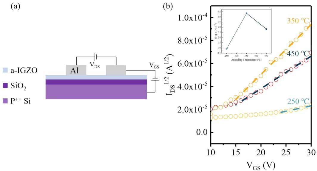
Figure S1. (a) A-IGZO thin film field effect transistor device structure diagram. (b)  $I_{DS}^{1/2}$ - $V_{GS}$  curve of a-IGZO thin films with different annealing temperature. The illustration shows the value of the slope of the fitting curve.
