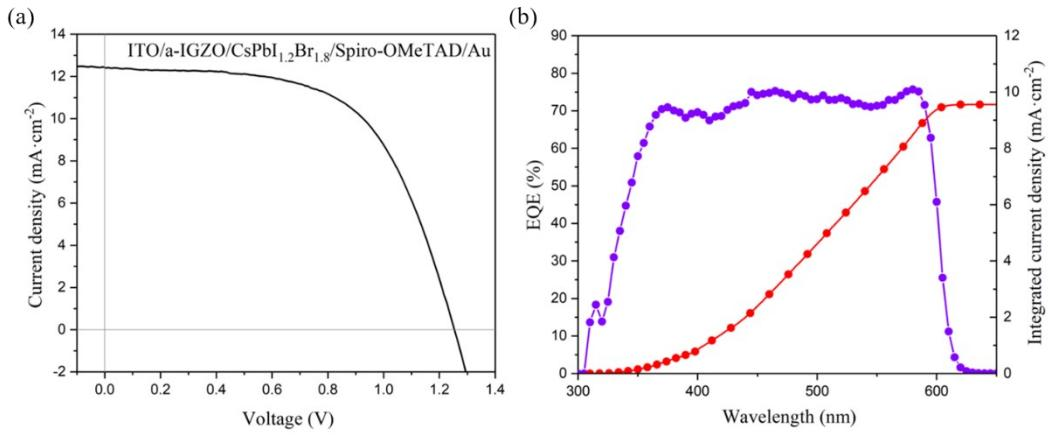
Figure S2. J-V curve (a) and EQE spectra and the corresponding integrated current densities (b) of the device with structure of ITO/a-IGZO (350 °C)/CsPbI<sub>1.2</sub>Br<sub>1.8</sub>/Spiro-OMeTAD/Au
