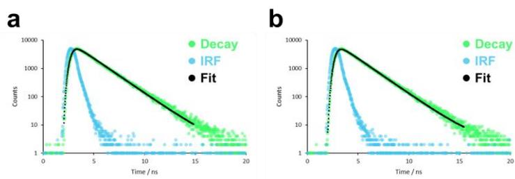
**Fig. S7** Emission decay curve of *uns*-CM and instrument response function (IRF) in a) benzene and b) toluene.
