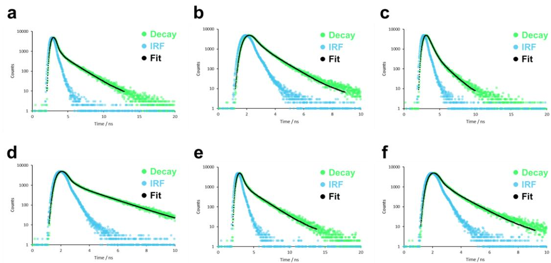
**Fig. S9** Emission decay curve of *uns*-CM and instrument response function (IRF) in (a) DMSO, (b) *i*PrOH, (c) acetone, (d) EtOH, (e) MeCN, and (f) MeOH.
