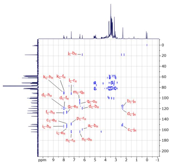
$^1\text{H}$ - $^{13}\text{C}$  HMQC NMR spectrum of *ins*-CM.
