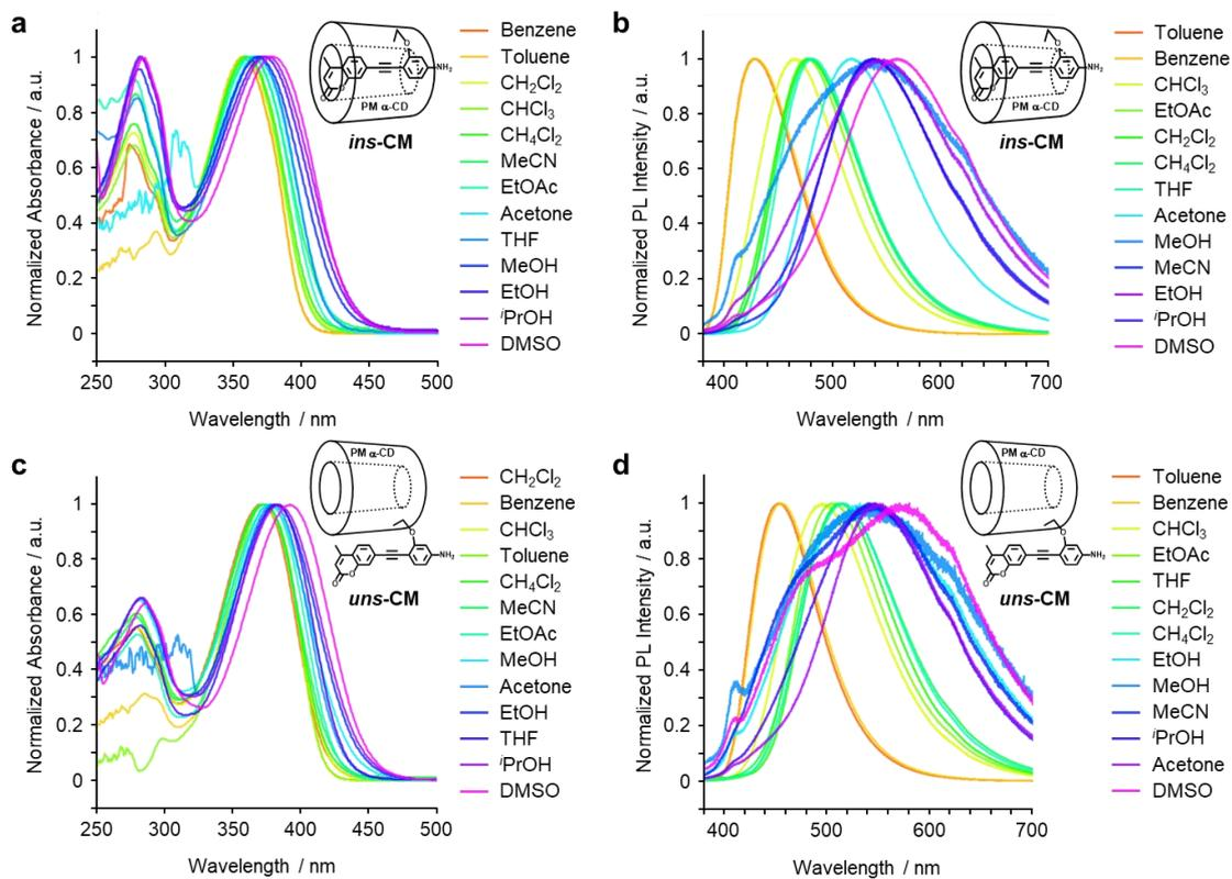
**Fig. S2** (a) Normalized absorption spectra and (b) photoluminescence spectra of *ins*-CM (excitation at 365 nm) in various solvents. (c) Normalized absorption spectra and (d) photoluminescence spectra of *uns*-CM (excitation at 365 nm) in various solvents.
