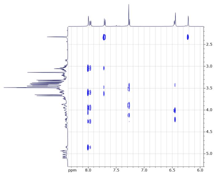
$^1\text{H}$ - $^{13}\text{C}$  HMBC NMR spectrum of *ins*-CM
