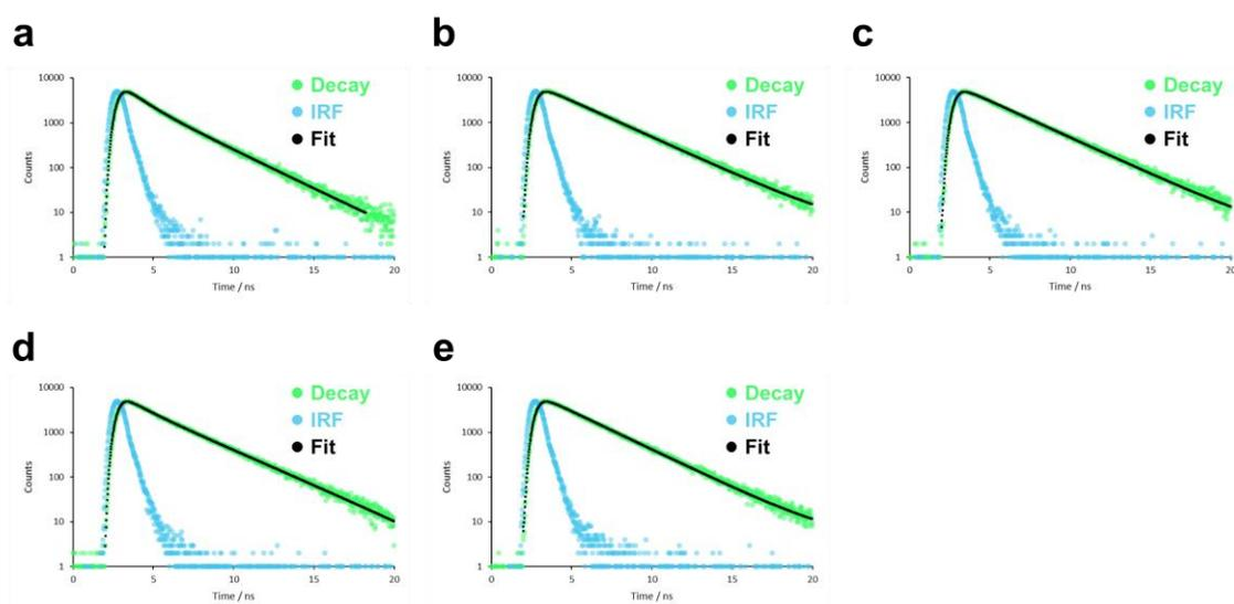
**Fig. S5** Emission decay curve of *ins*-CM and instrument response function (IRF) in (a)  $\text{CHCl}_3$ , (b) EtOAc, (c) THF, (d)  $\text{CH}_2\text{Cl}_2$ , and (e)  $\text{CH}_4\text{Cl}_2$ .
