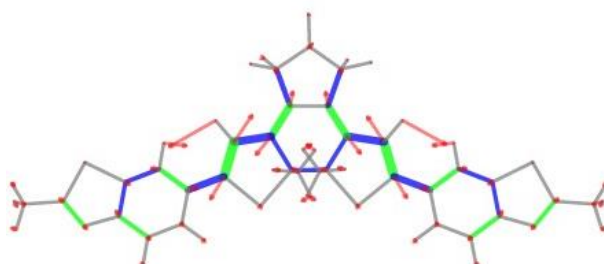
Figure S51. Raman normal mode corresponding to the CC skeletal vibration of 4 (left: 1550 \text{cm}^{-1} ; 227 \text{km/mol} ; 68237 \text{A}^4/\text{amu} ; right: 1548 \text{cm}^{-1} ; 53 \text{km/mol} ; 27990 \text{A}^4/\text{amu} ).
