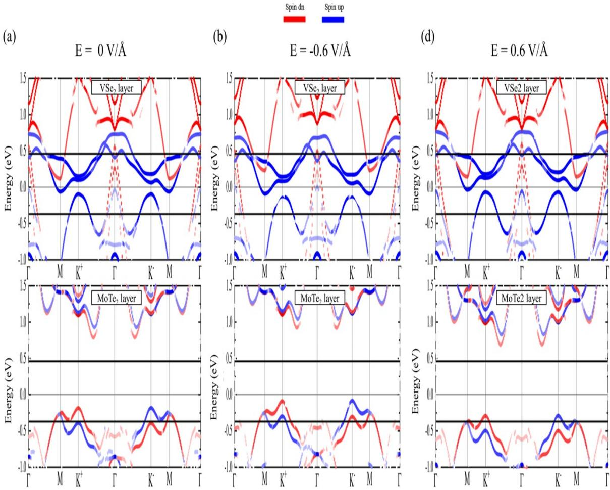
**Fig. S5** Layer dependent projected SOC band structure of MoTe<sub>2</sub>/VSe<sub>2</sub> heterostructure at (a)  $E = 0 \text{ V/\AA}$ , (b)  $E = -0.6 \text{ V/\AA}$ , and (c)  $E = 0.6 \text{ V/\AA}$ . Here, the blue line represents the majority spin component and the red line is the minority spin component.
