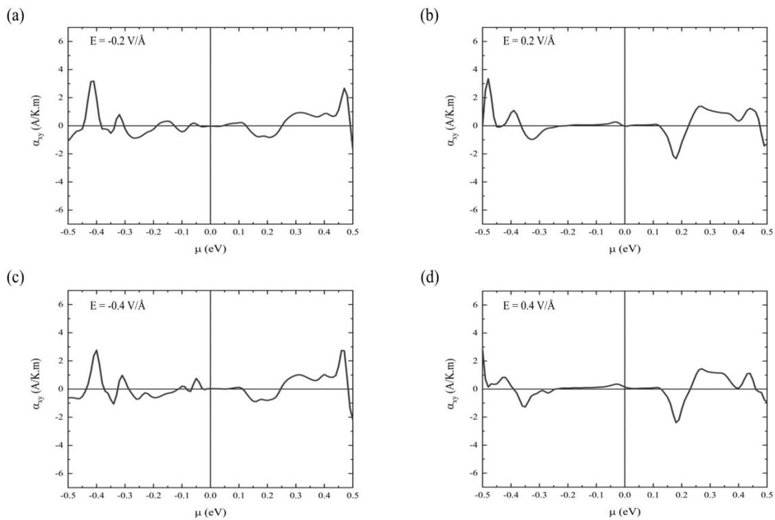
**Fig. S6** Electric field dependent anomalous Nernst conductivity ( $\alpha_{xy}$ ) as a function of chemical potential ( $\mu$ ) at (a)  $E = -0.2 \text{ V/\AA}$ , (b)  $E = 0.2 \text{ V/\AA}$ , (c)  $E = -0.4 \text{ V/\AA}$  and (d)  $E = 0.4 \text{ V/\AA}$ .
