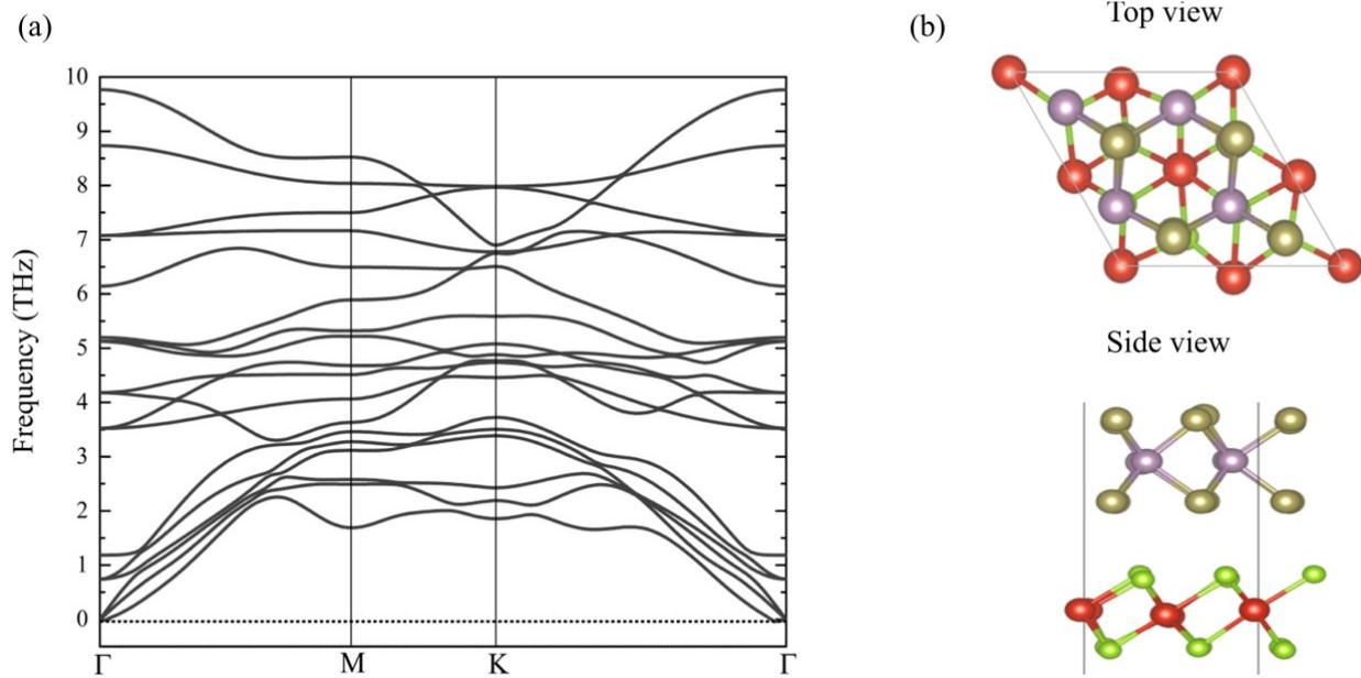
**Fig. S1** (a) calculated phonon dispersion of the MoTe<sub>2</sub>/VSe<sub>2</sub> heterostructure. (b) Top and side views snapshot of the molecular dynamics simulations of the MoTe<sub>2</sub>/VSe<sub>2</sub> heterostructure at 300 K up 5 ps.
