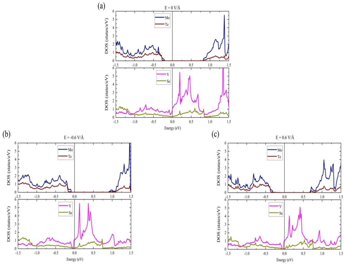
**Fig. S3** Layer dependent density of states (DOS) of MoTe<sub>2</sub>/VSe<sub>2</sub> heterostructure at (a)  $E = 0 \text{ V/\AA}$ , (b)  $E = -0.6 \text{ V/\AA}$ , and (c)  $E = 0.6 \text{ V/\AA}$ .
