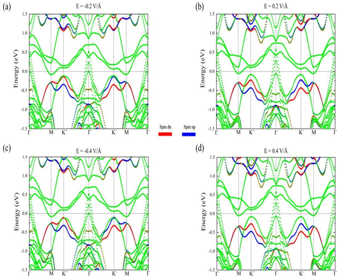
**Fig. S2** Electric field dependent SOC band structure of the MoTe<sub>2</sub>/VSe<sub>2</sub> heterostructure at (a)  $E = -0.2 \text{ V/\AA}$ , (b)  $E = 0.2 \text{ V/\AA}$ , (c)  $E = -0.4 \text{ V/\AA}$  and (d)  $E = 0.4 \text{ V/\AA}$ . Here, the green line represents the contribution from the VSe<sub>2</sub> layer while the blue line represents the majority spin component and the red line is the minority spin component from the MoTe<sub>2</sub> layer.
