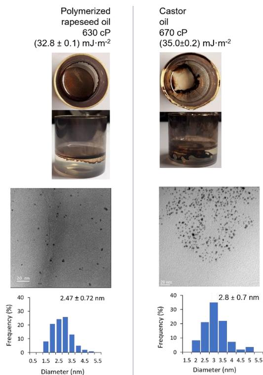
**Figure S7.** Comparison of the samples obtained by sputtering onto polymerized rapeseed oil (left) and castor oil (right). Sputtering conditions were identical: 4 g of oil, WD of 20 cm, argon pressure of 0.07 Pa, sputter power of 80 W and sputter time of 5 minutes.
