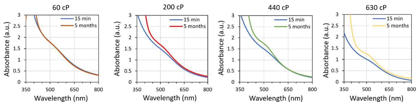
**Figure S5.** UV-vis spectra of colloidal solutions of AuNPs 15 minutes and 5 month after preparation in case of oil viscosity of 60 cP, 200 cP, 440 cP and 630 cP respectively.
