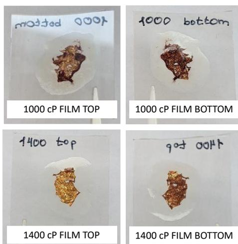
**Figure S4.** Images of the top and bottom sides of the gold films deposited onto oils with viscosities of 1000 cP and 1400 cP.
