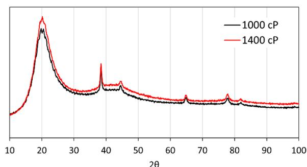
**Figure S6.** XRD of a gold metallic films placed on a glass plate covered with amorphous TiO<sub>2</sub>.
