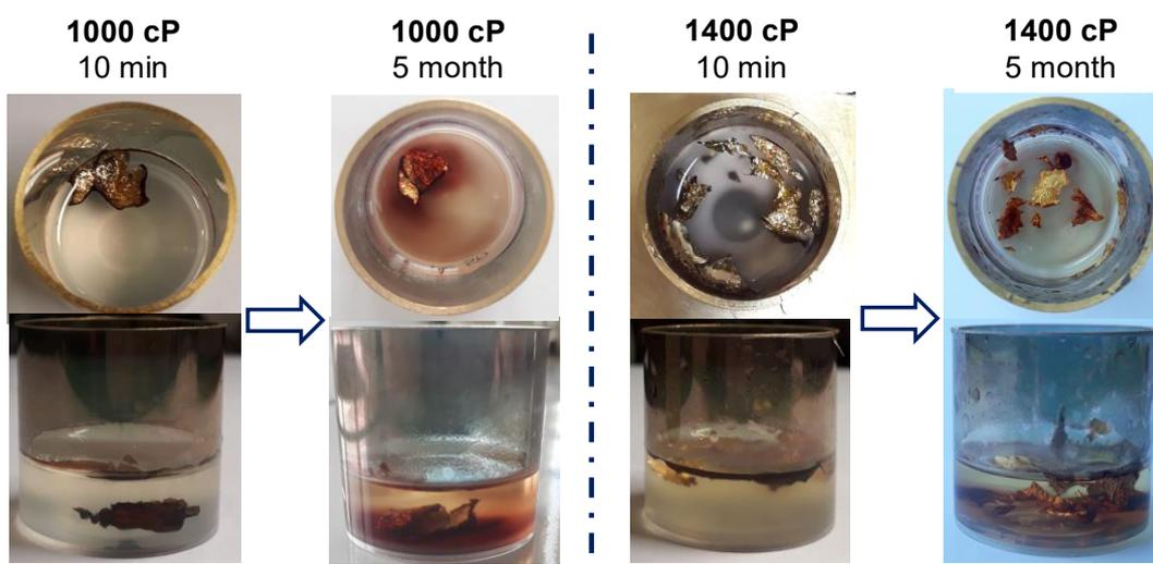
**Figure S3.** Migration of Au NPs from the bottom surface of the film to the bulk solution within storage time.
