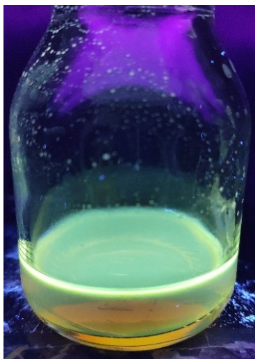
Figure S2. Light green emission from G-CQDs sample excited by 365 nm Uv lamp after the salting-out process.
