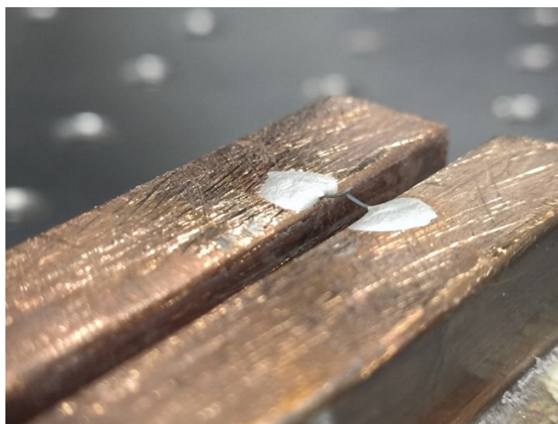
Figure S2. The MXene sample in heating treatment at 65°C
