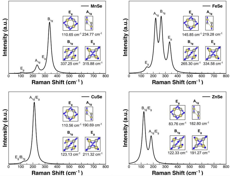
FIG. 6. Raman spectra and the vibrational characteristics of the Raman-active phonon modes for the single-layer MnSe, FeSe, CuSe and ZnSe.
