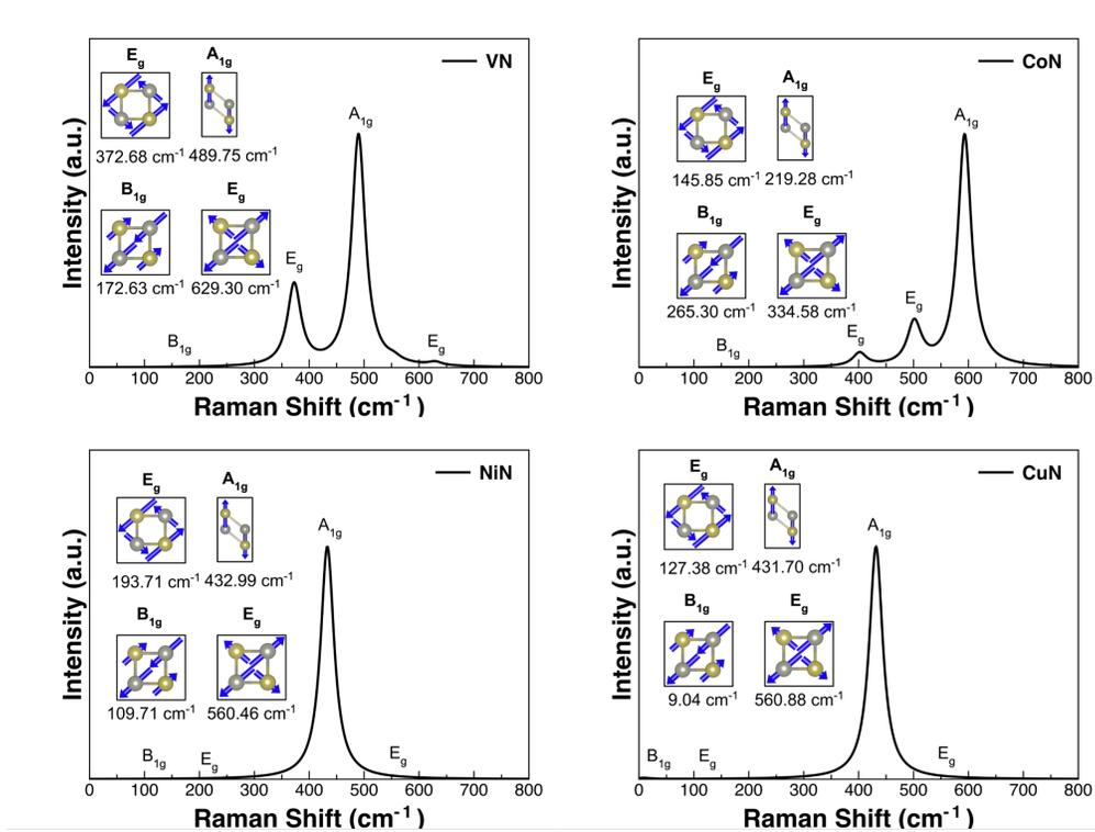
FIG. 4. Raman spectra and the vibrational characteristics of the Raman-active phonon modes for the single-layer VN, CoN, NiN, and CuN.
