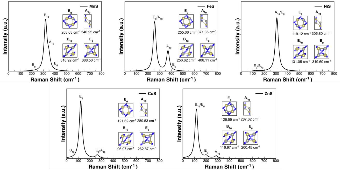
FIG. 7. Raman spectra and the vibrational characteristics of the Raman-active phonon modes for the single-layer MnS, FeS, NiS, CuS and ZnS.
