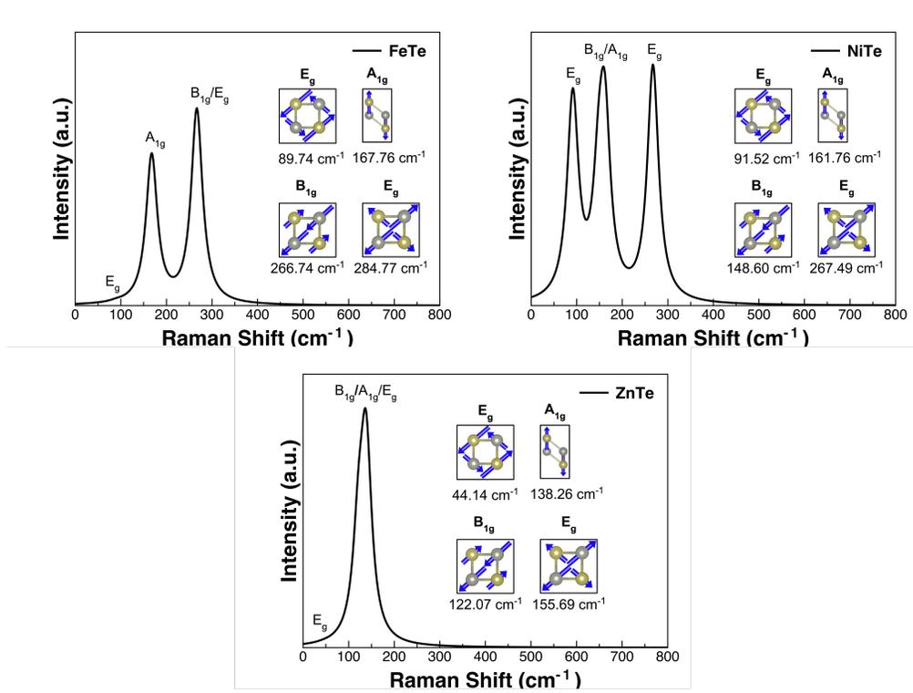
FIG. 8. Raman spectra and the vibrational characteristics of the Raman-active phonon modes for the single-layer FeTe, NiTe, and ZnTe.
