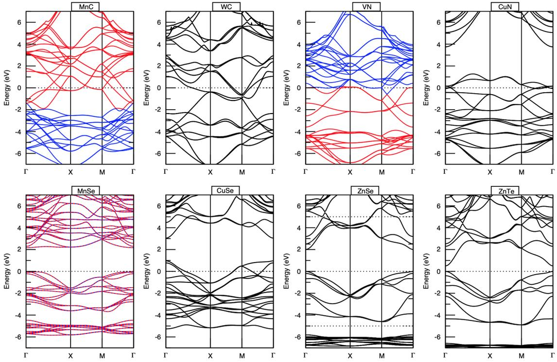
FIG. 2. Electronic structures of single layer MnC, WC, VN, CuN, MnSe, CuSe, ZnSe, and ZnTe. In all figures, blue, red and black lines correspond to spin-up, spin-down and non-magnetic case, respectively.
