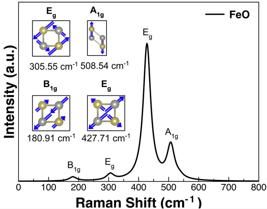
FIG. 5. Raman spectra and the vibrational characteristics of the Raman-active phonon modes for the single-layer FeO.
