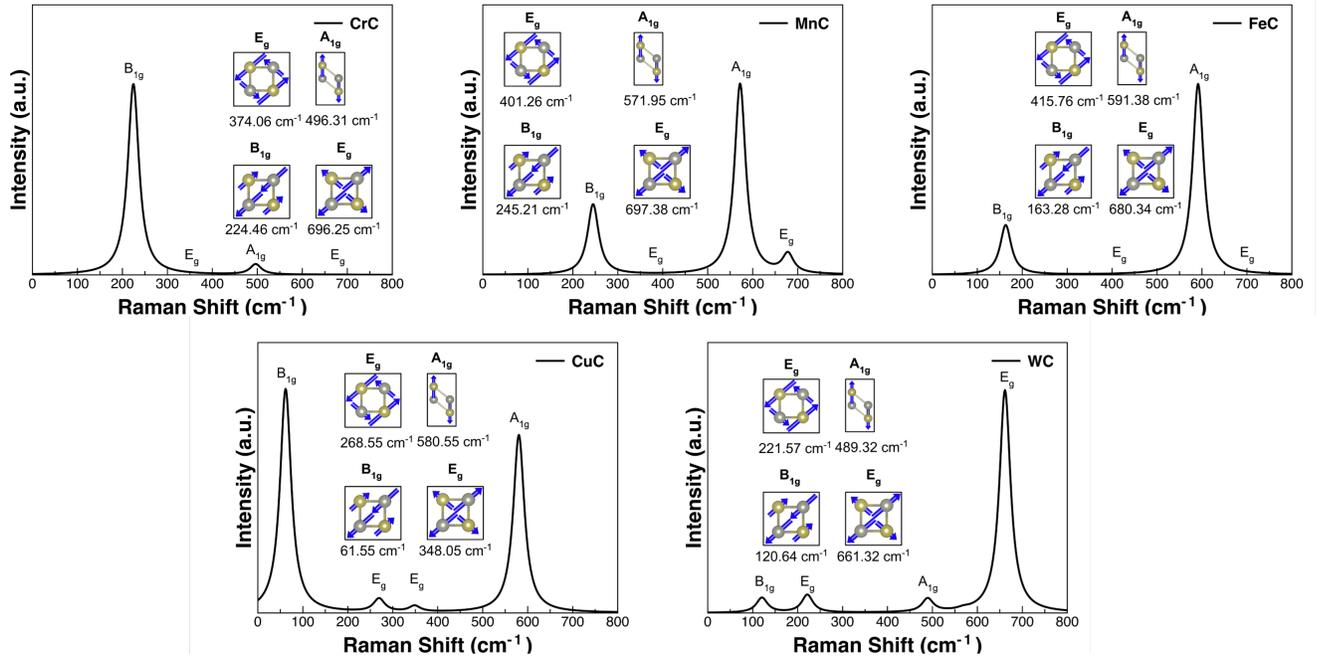
FIG. 3. Raman spectra and the vibrational characteristics of the Raman-active phonon modes for the single-layer CrC, MnC, FeC, CuC, and WC.
