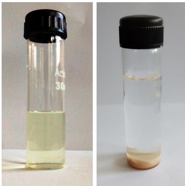
Fig. S4 Photo of (a) aqueous \text{HAuCl}_4 solution and (b) after adsorption of \text{AuCl}_4^- anions by SBA-15- pr -SH material.
