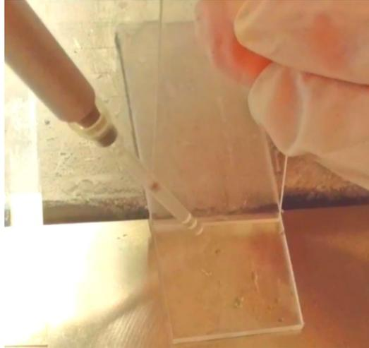
**SI-FIG. S4. Photo of the freeze extraction process.** The sapphire with the frozen sample was slid stripe by stripe over onto a 45°C warm aluminum block to melt the frozen sample stripe by stripe. To ensure that two adjacent stripes were not inadvertently mixed during the stripwise thawing, a hydrophobic barrier (glass cover slide wrapped with Teflon foil) was held between each stripe. The contents of each thawed stripe were pipetted into different low-binding Eppendorf tubes
